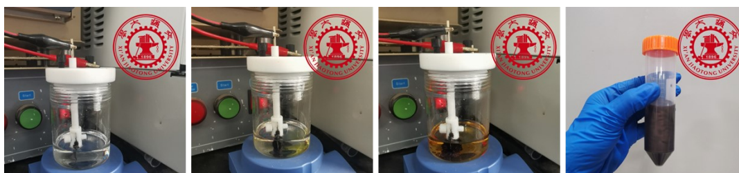
Fig. S4. Electrochemical cathode exfoliation process from bulk NiPS_3 to exf- NiPS_3 nanosheets.
