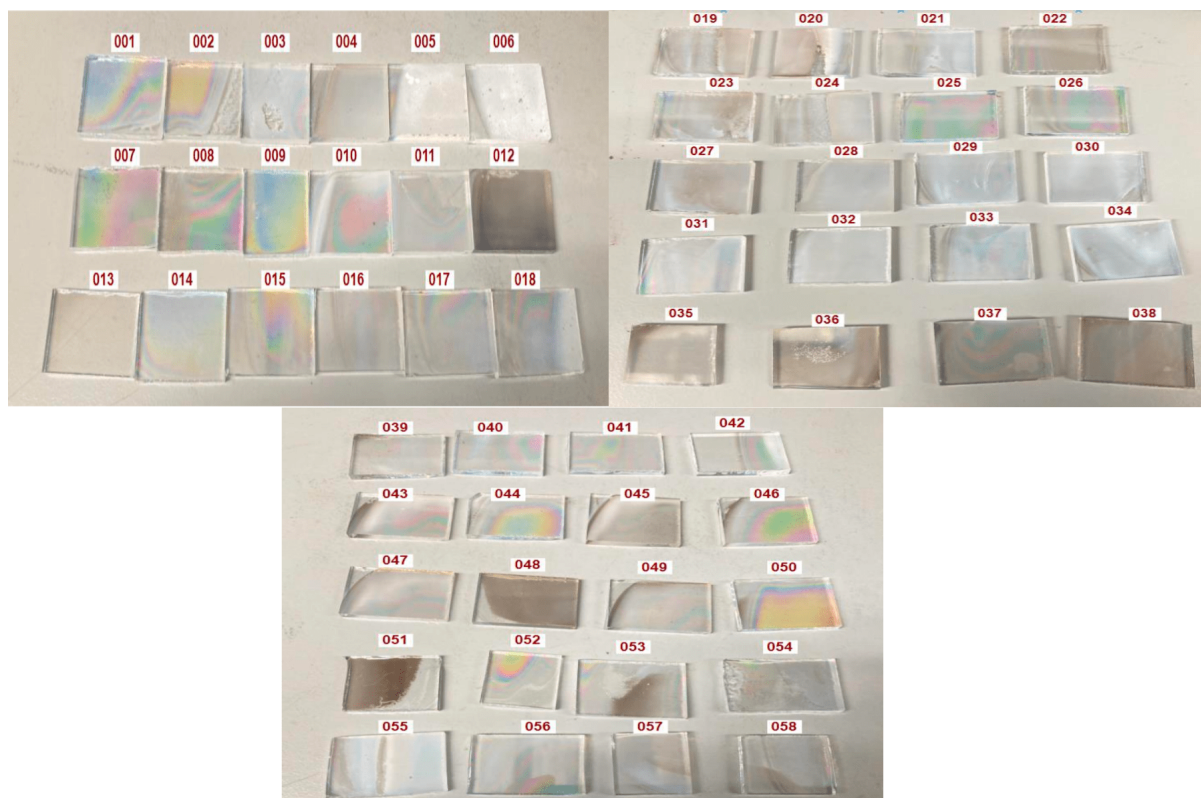
Figure S3: Photographs of all 58 unique \text{TiO}_2 coatings on glass synthesized using APCVD with differing synthesis parameters.
