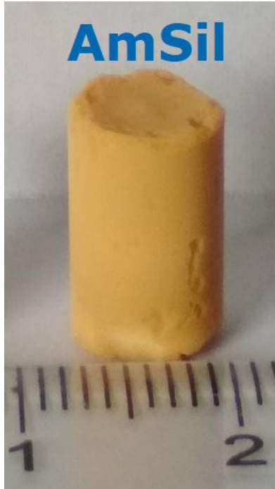
(f) Photographic image of monolithic aerogel obtained after supercritical drying.
