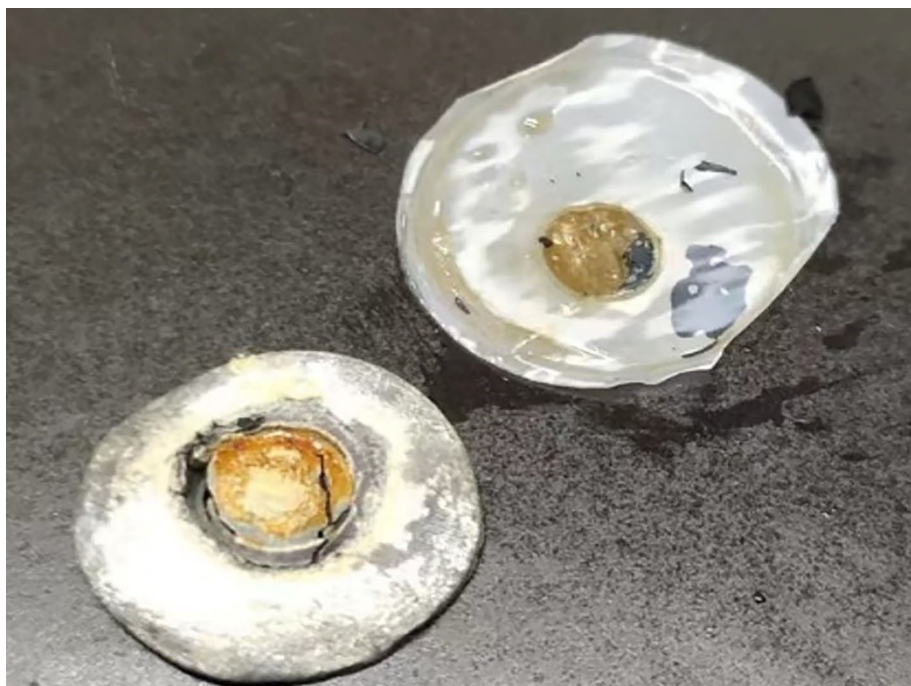
Fig S15. Optical photographs of Li metal anode after 100 cycles of LFP/CNT/TPAE//Li cell with LFP areal mass loading of 34.5 \text{ mg} \cdot \text{cm}^{-2} .
