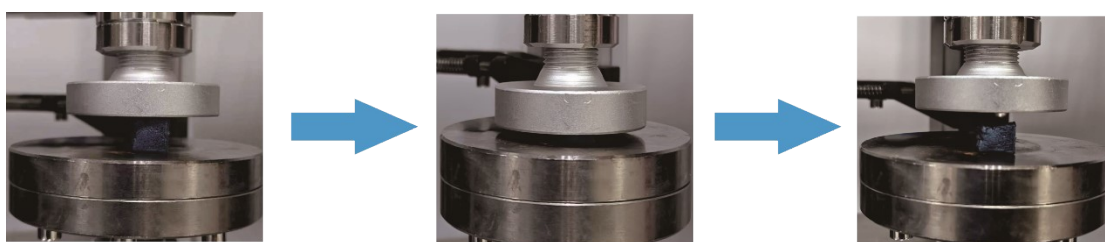
Fig. S8. Photographs of the loading-unloading process of the BLPP foam
