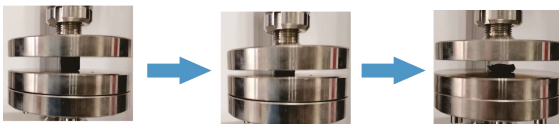
Fig. S7. Photographs of the loading-unloading process of the SBPP foam
