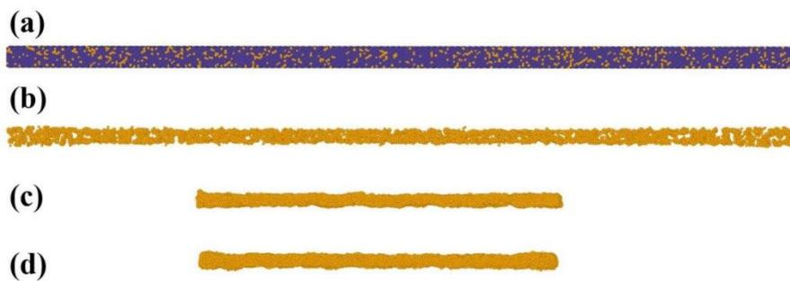
**Figure S3.** Reconstruction of nanowire catalyst. (a) A  $\text{Pt}_{15}\text{Ni}_{85}$  nanowire. (b) Removing all Ni atoms. (c) Nanowire structure after NPT simulation using eam potential. (d) Final nanowire catalyst. The orange and purple beads represent the Pt and Ni atoms, respectively.
