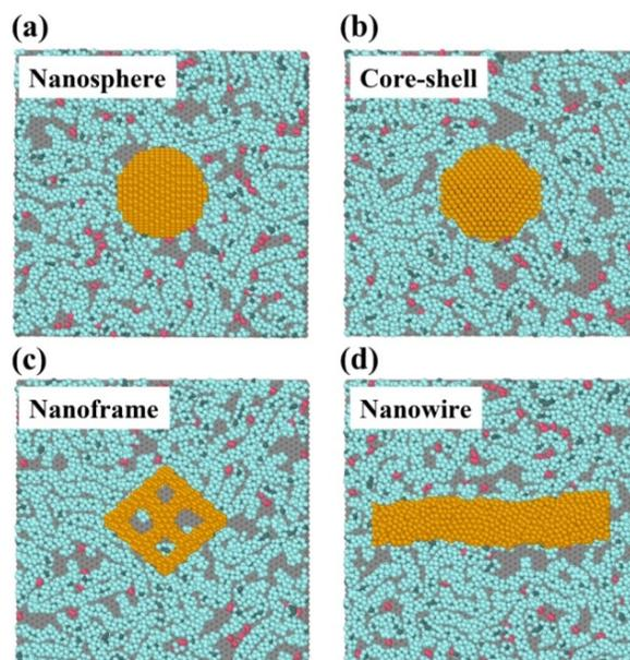
**Figure S7.** Snapshots in the regions within 0.73 nm from the carbon support for (a) nanosphere, (b) core-shell, (c) nanoframe, and (d) nanowire, respectively. The gray, orange, dark green, cyan and pink beads represent the carbon support atoms, Pt atoms, carbon atoms in PFSA, sulfur/oxygen/fluorine atoms in PFSA, oxygen molecules, respectively.
