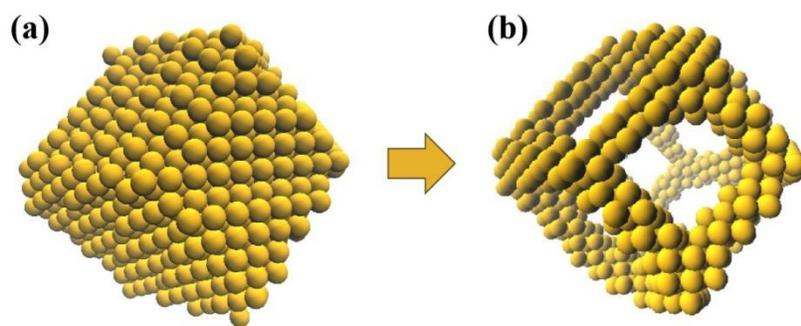
**Figure S2.** Reconstruction of nanoframe catalyst. (a) A rhombic dodecahedron full of Pt atoms with fcc lattices. (b) Nanoframe structure by deleting Pt atoms inside the body and at the center of surfaces.
