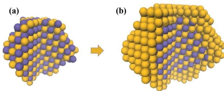
**Figure S1.** Reconstruction of core-shell catalyst. (a) Core of catalyst: Pt-Co alloy with L<sub>10</sub> lattice. (b) Core-shell catalyst. The orange and purple beads represent the Pt and Co atoms, respectively.
