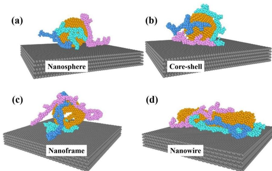
**Figure S6.** PFSA chains around (a) nanosphere, (b) core-shell, (c) nanoframe and (d) nanowire. The yellow beads represent catalysts, while other beads with different colors represent the different PFSA chains.
