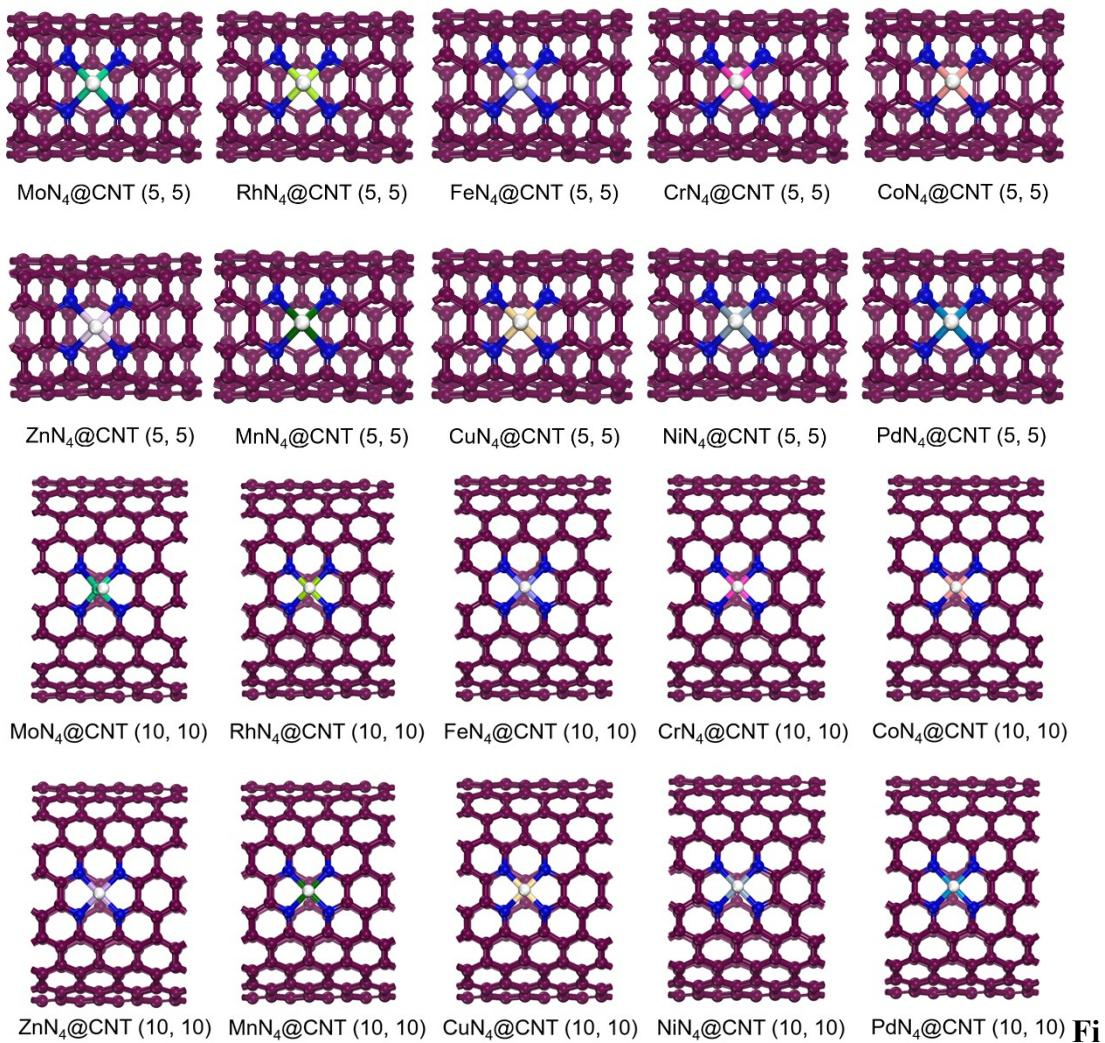
**g. S2** Optimized geometries of H adsorption on TMN<sub>4</sub>@CNTs (n, n) (n=5, 10) (TM=Mo, Rh, Fe, Cr, Co, Zn, Mn, Cu, Ni, Pd). The lattice parameters were set to be 15×15×10 Å<sup>3</sup> for CNTs (5, 5) and 23×23×10 Å<sup>3</sup> for CNTs (10, 10).
