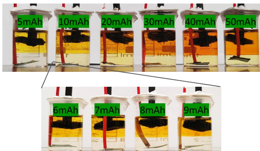
Figure S9. Photographs showing the diffusion of polybrominides in the biphasic ZBBs at different charge capacities.
