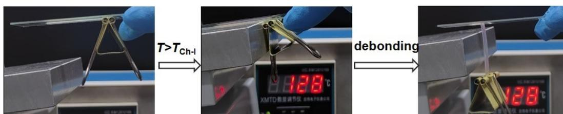
**Fig. S13** Heat-induced peeling. A strip of our LCE ( $RM_{0.5\%}$ - $CLCE_{3.5\%}$ , width:  $w = 7.5$  mm, thickness:  $d = 0.32$  mm, and length of  $\sim 25$  mm) was first adhered on a glass slide where the LCE was in the chiral phase. Then, one side of the strip is pulled at  $90^\circ$  from the substrate under a constant force of 0.2 N, by hanging a weight. The sample was then heated beyond  $T_{Ch-I}$  from the top side, and the debonding and peeling was observed.
