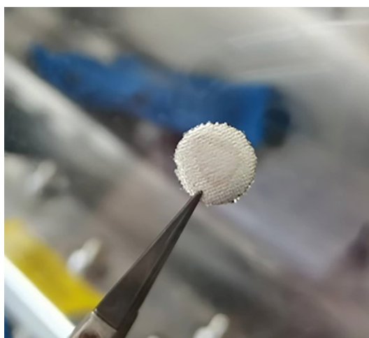
Fig. S14. Digital image of \text{CoS}_2\text{-Co(OH)F/CC} framework for 10 \text{ mAh cm}^{-2} of Li.
