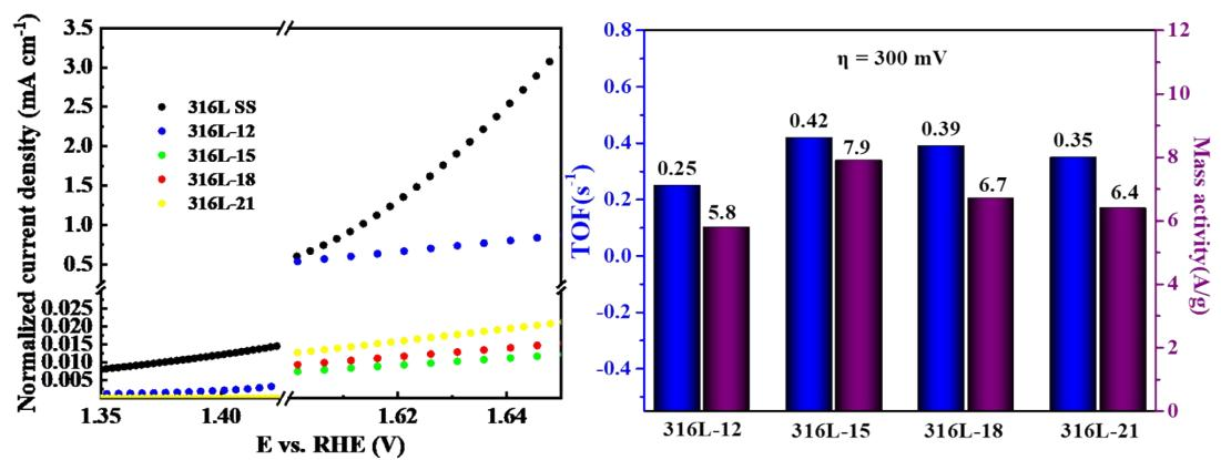
**Fig. S16** (a)Normalized current density by the ECSA and (b)Mass activity and TOF values of the 316L-12, 316L-15, 316L-18 and 316L-21 at the overpotential of 300 mV.
