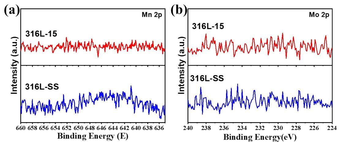
**Fig. S15** High-resolution XPS spectra of (a) Mn 2p and (b) Mo 2p for the 316-SS and 316-15.
