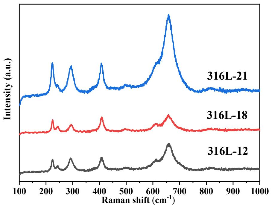
**Fig. S8** Raman spectra of the 316L-12, 316L-18 and 316L-21 sample.
