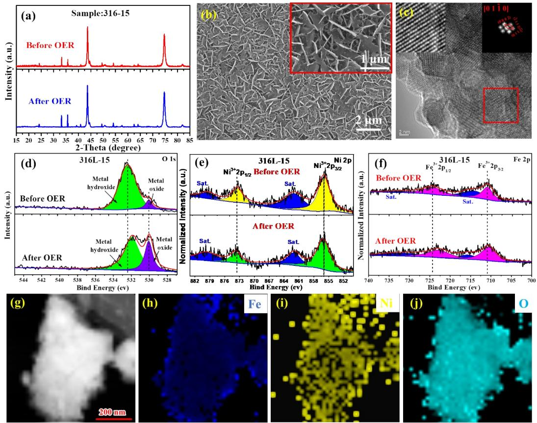
**Fig. S17** (a) XRD patterns of 316L-15 before and after OER. (b) Low and high(inset) magnification SEM images (c) HRTEM images (inset: the corresponding fast Fourier transform (FFT) pattern) of 316L-15 after OER. (d-f) High-resolution of XPS spectra of (d)O 1s, (e)Ni 2p, and (f)Fe 2p of 316L-15 before and after OER. (g-j) EDX element mapping images of 316L-15 after OER.
