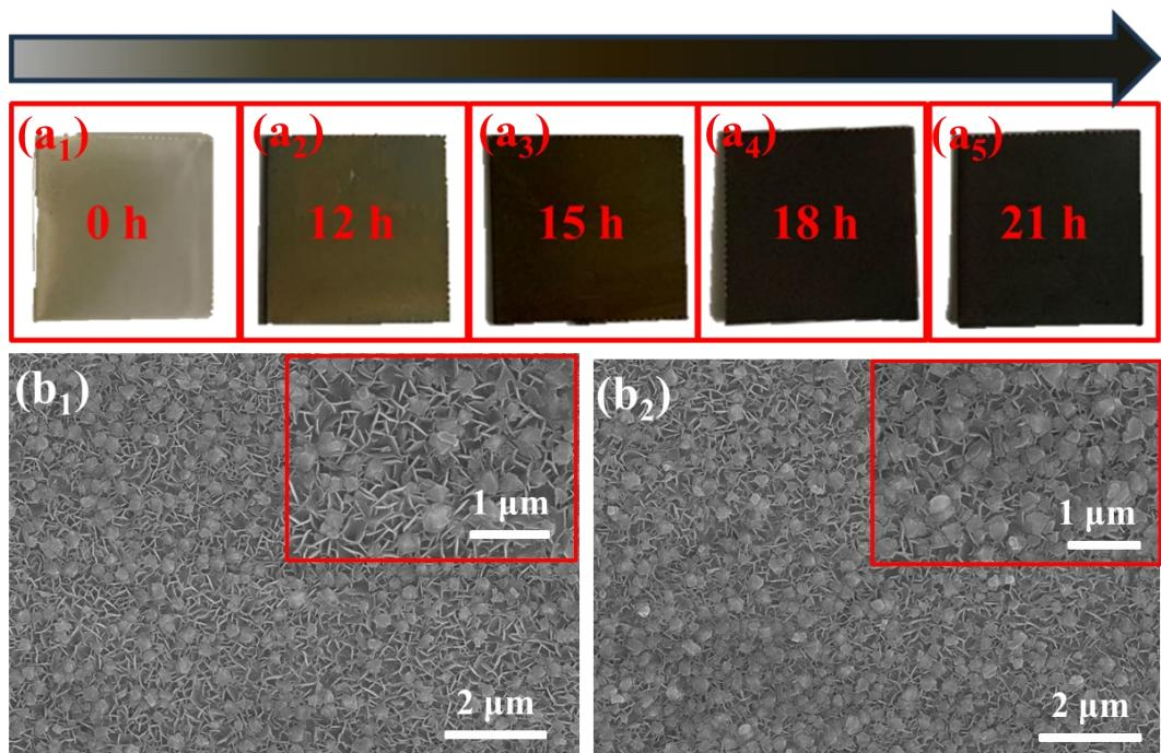
**Fig. S7** (a<sub>1</sub>-a<sub>5</sub>)The digital images of the prepared corrosion electrodes with the hydrothermal time((a<sub>1</sub>)0 h, (a<sub>2</sub>)12 h, (a<sub>3</sub>)15 h, (a<sub>4</sub>)18 h, (a<sub>5</sub>)21 h). (b<sub>1</sub>-b<sub>2</sub>)SEM images of the surface of the prepared corrosion electrodes with the corrosion time( (b<sub>1</sub>)18 h, (b<sub>2</sub>)21 h).
