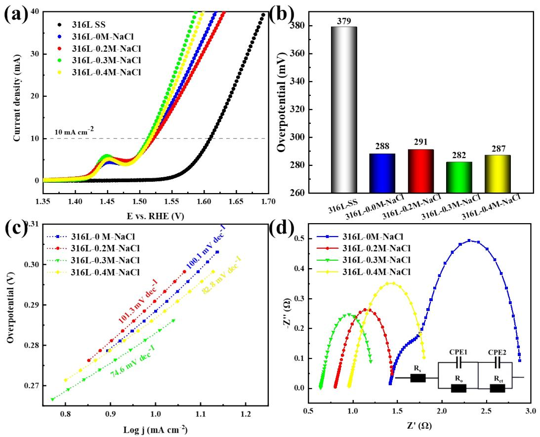
**Fig. S4** (a)LSC curves, (b)Overpotentials at  $10 \text{ mA cm}^{-2}$ , (c)Tafel slopes, (d)EIS curves of the 316L-SS, 316L-0M-NaCl, 316L-0.2M-NaCl, 316L-0.3M-NaCl and 316L-0.4M-NaCl (inset: corresponding equivalent circuit used for fitting the Nyquist plots).
