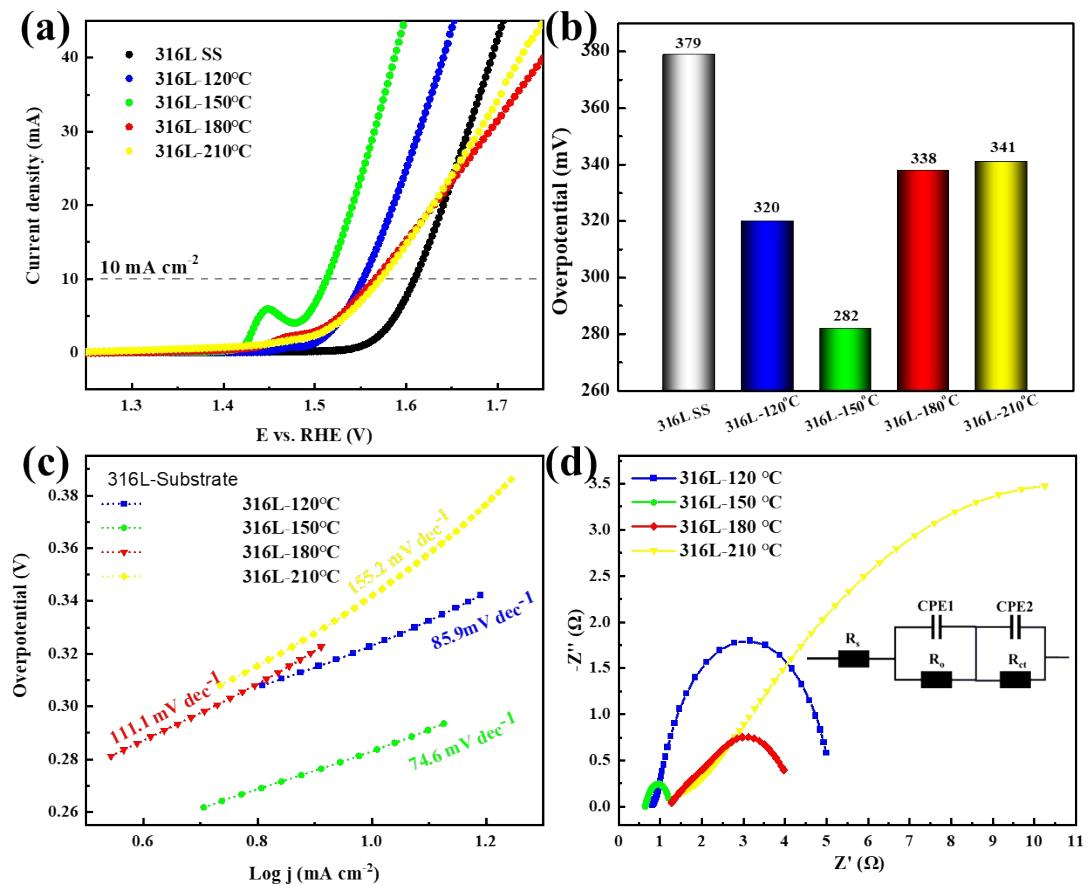
**Fig. 2** (a)LSC curves, (b)Overpotentials at  $10 \text{ mA cm}^{-2}$ , (c)Tafel slopes, (d)EIS curves of the 316L-bank, 316L-120 °C, 316L-150 °C, 316L-180 °C and 316L-210 °C(inset: corresponding equivalent circuit used for fitting the Nyquist plots).
