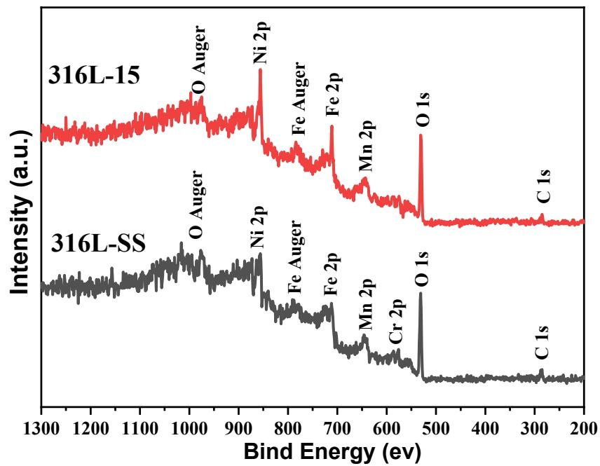
**Fig. S9** XPS survey spectra of 316L-SS and 316L-15 sample
