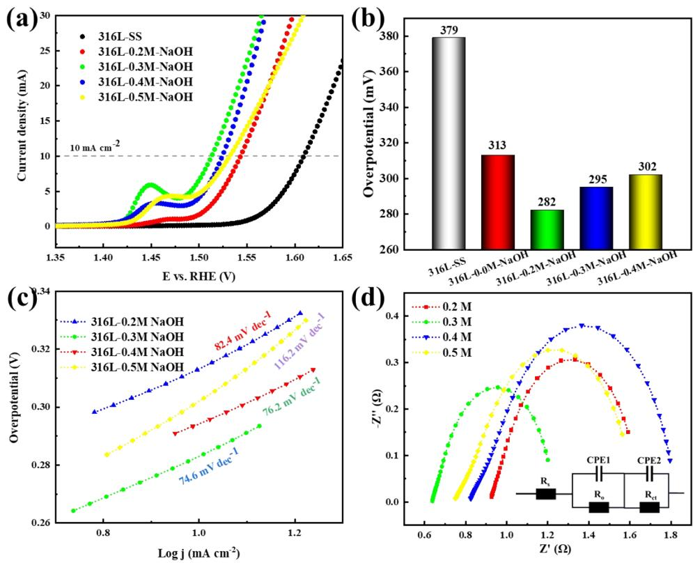
**Fig. S6** (a)LSC curves, (b)Overpotentials at  $10 \text{ mA cm}^{-2}$ , (c)Tafel slopes, (d)EIS curves of the 316L-SS, 316L-0.2M-NaOH, 316L-0.3M-NaOH, 316L-0.4M-NaOH and 316L-0.5M-NaOH(inset: corresponding equivalent circuit used for fitting the Nyquist plots).
