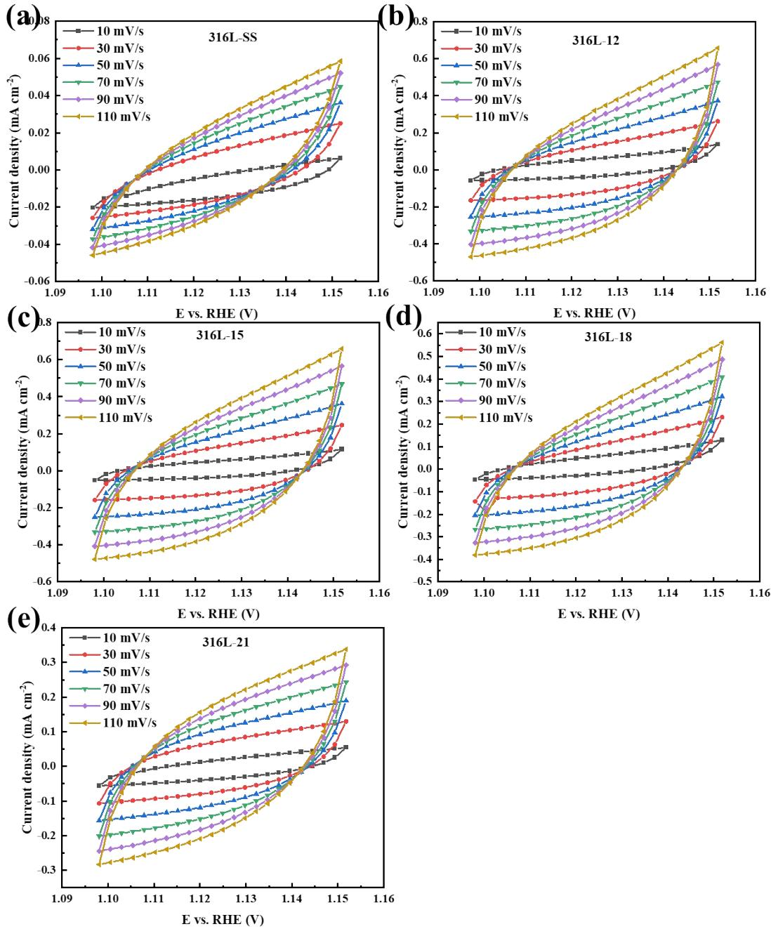
**Fig. S10** Cyclic voltammograms of (a) 316L-SS, (b) 316L-12, (c) 316L-15, (d) 316L-18 and (e) 316L-21 at the scan rate of  $10 \text{ mV s}^{-1}$ ,  $30 \text{ mV s}^{-1}$ ,  $50 \text{ mV s}^{-1}$ ,  $70 \text{ mV s}^{-1}$ ,  $90 \text{ mV s}^{-1}$  and  $110 \text{ mV s}^{-1}$ , respectively.
