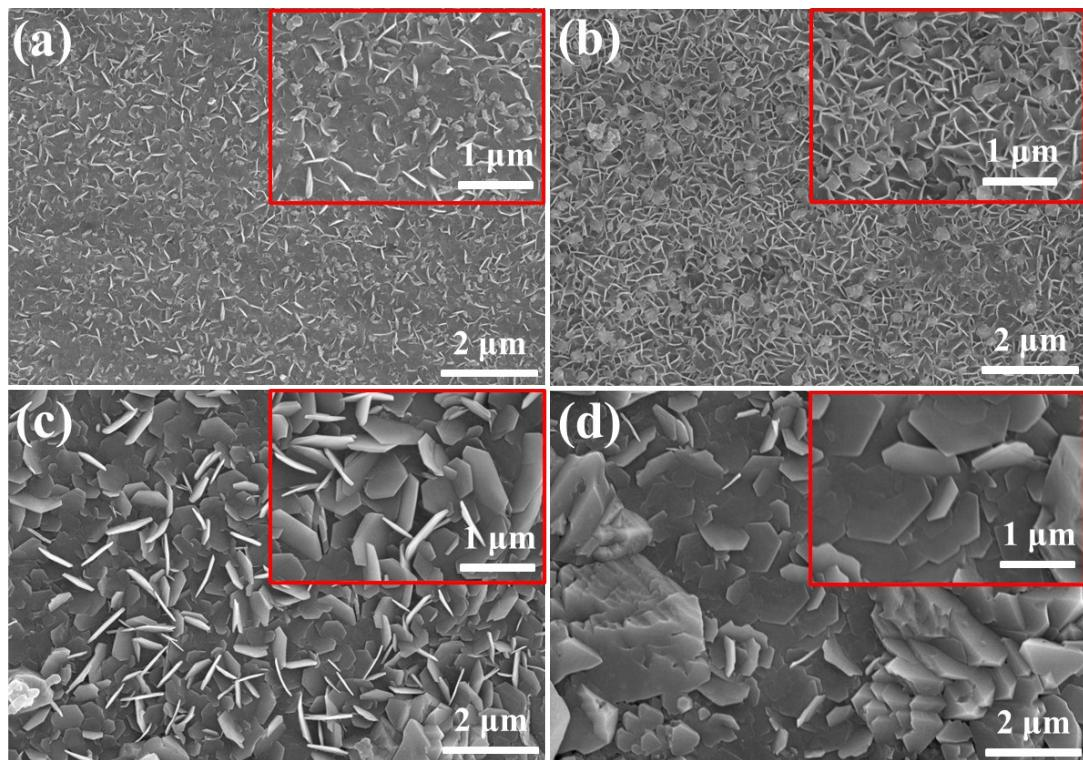
**Fig. S1** SEM images of the surface of the prepared corrosion electrodes with the hydrothermal temperature((a)120 °C, (b)150 °C, (c)180 °C, (d)210 °C).
