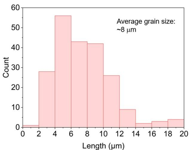
**Figure S1.** The analysis on SEM image to determine the average grain size of cold-pressed LLZTO sample.
