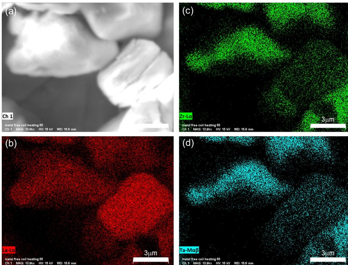
**Figure S3.** (a) Selected region for EDS mapping of aged LLZTO sample. (b-d) EDS mapping results of the selected region for La, Zr, and Ta elements.
