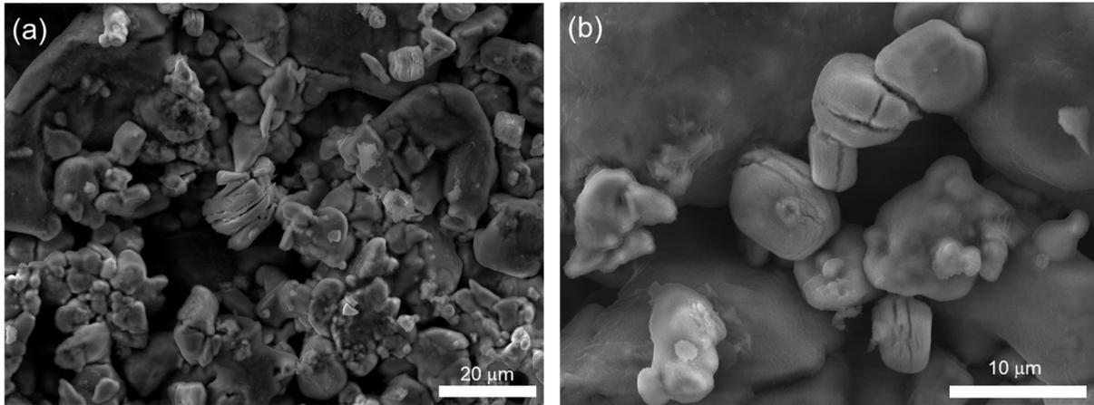
**Figure S2.** Additional SEM images of aged LLZTO sample showing cracked grains.
