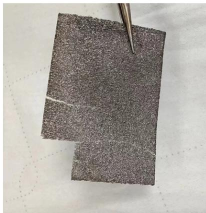
**Figure S2.** Representative photo of the samples subjected to nitridation temperature of 420 °C.
