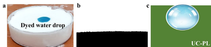
Figure S21. (a) Photograph of a water droplet on UC-PL. (b) Photograph of a water droplet on UC-PL using a contact angle meter. (c) Schematic for a water droplet on UC-PL.
