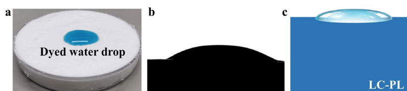
Figure S22. (a) Photograph of a water droplet on LC-PL. (b) Photograph of a water droplet on LC-PL using a contact angle meter. (c) Schematic for a water droplet on LC-PL.
