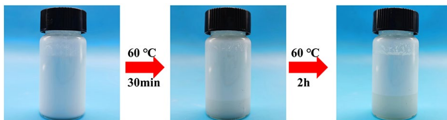
Figure S4. Optical photos of UC-PL without adding XG during 2 hours standing test.
