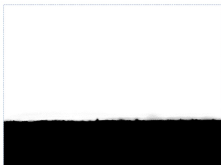
Figure S8. Contact angle of n -hexane on UC-TSG (ca. 0°).
