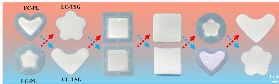
Figure S15. TSG's plastic-like processing capabilities.
