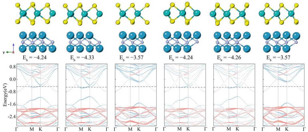
**Fig. S1** The MoS<sub>2</sub>/Ca<sub>2</sub>N heterostructures and their band structures. The red and blue bubbles depict the projected band structure of MoS<sub>2</sub> and Ca<sub>2</sub>N.
