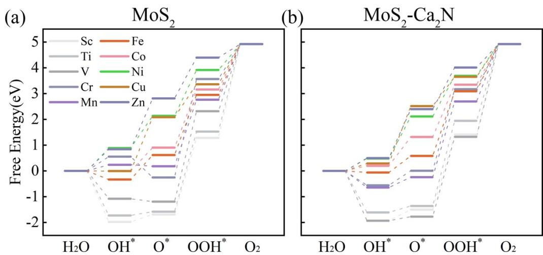
**Fig. S7** Free energy paths of the OER for TM single atom on  $\text{MoS}_2$ , and  $\text{MoS}_2\text{/Ca}_2\text{N}$  at  $U = 0$  V
