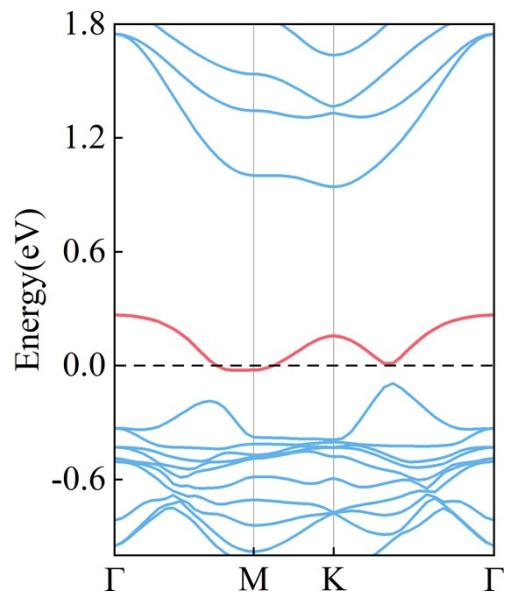
**Fig. S4** The band structure of the MoS<sub>2</sub>/Ca<sub>2</sub>N heterostructure. The red line indicates electron layer related bands at the interface of MoS<sub>2</sub>/Ca<sub>2</sub>N heterostructure.
