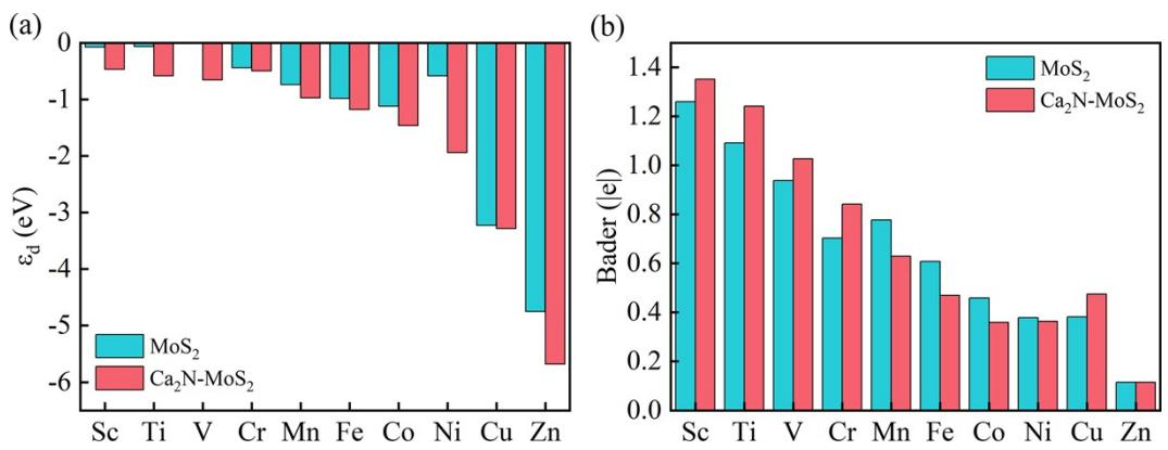
**Fig. S6** (a) The  $d$ -band center and (b) charge transfer of TM atoms in the catalyst.
