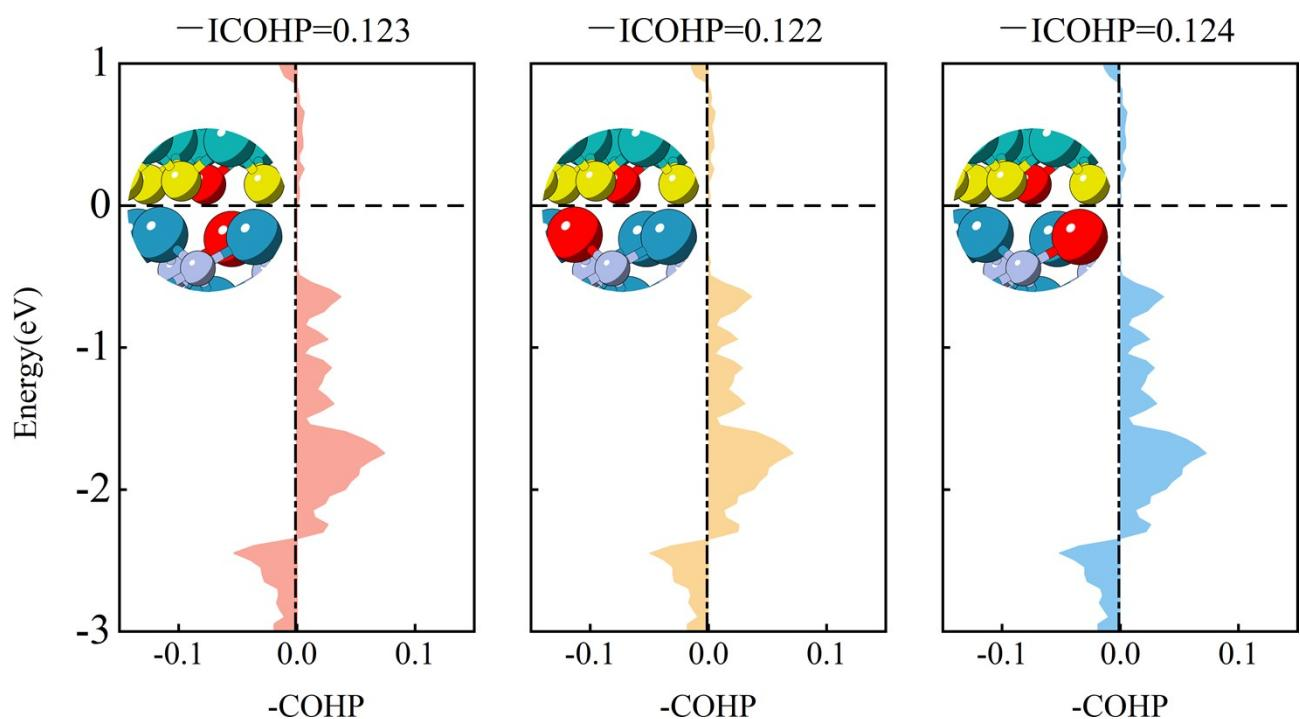
**Fig. S3** The  $-\text{COHP}$  between  $\text{S}$  atom at the interface of  $\text{MoS}_2/\text{Ca}_2\text{N}$  heterojunction and the three closest  $\text{Ca}$  atoms is depicted in red.
