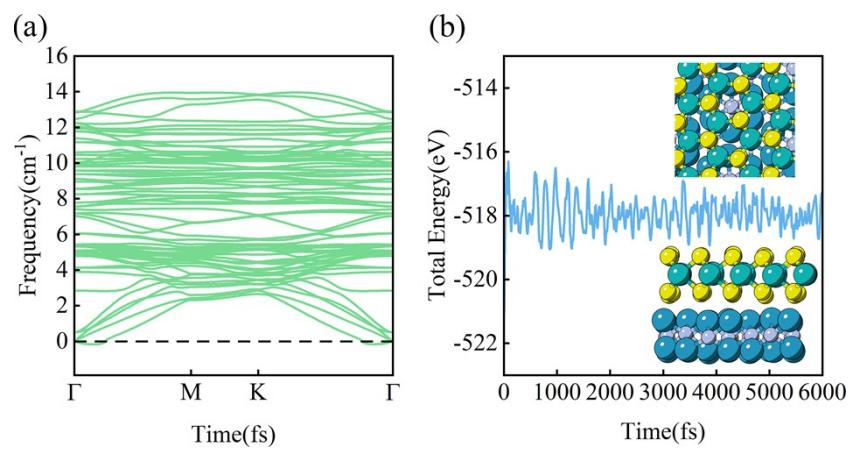
**Fig. S2** (a) Phonon dispersions of MoS<sub>2</sub>/Ca<sub>2</sub>N heterostructure and (b) the fluctuations of energy and the final configuration of MoS<sub>2</sub>/Ca<sub>2</sub>N heterostructure.
