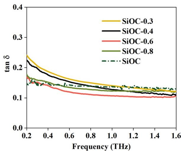
Fig. S7 The loss tangent value of the dielectric constant ( $\tan \delta$ ) of SiOC and  $Ti_3C_2T_x$  MXene/SiOC ceramic composite.
