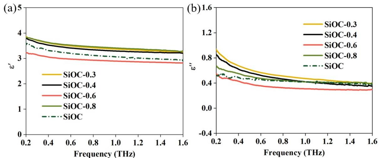
Fig. S6 (a) The real part ( $\epsilon'$ ) and (b) imaginary parts ( $\epsilon''$ ) of dielectric constant of SiOC and  $Ti_3C_2T_x$  MXene/SiOC ceramic composite.
