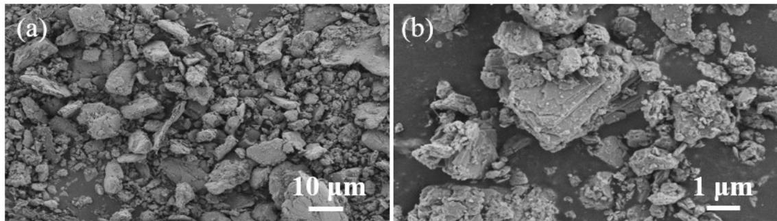
Fig. S1 (a, b) SEM images of  $\text{Ti}_3\text{AlC}_2$ .
