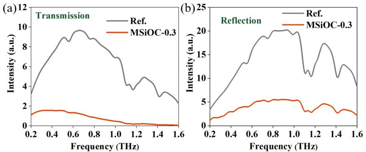
Fig. S4 Frequency-domain spectra of  $\text{Ti}_3\text{C}_2\text{T}_x$  MXene/SiOC-0.3 composite in (a) transmission and (b) reflection mode.
