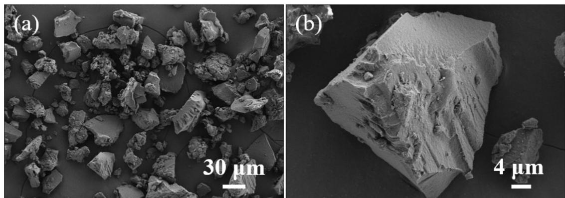
Fig. S2 (a, b) SEM images of the photocured  $\text{Ti}_3\text{C}_2\text{T}_x$  MXene/resin-0.3 composite.
