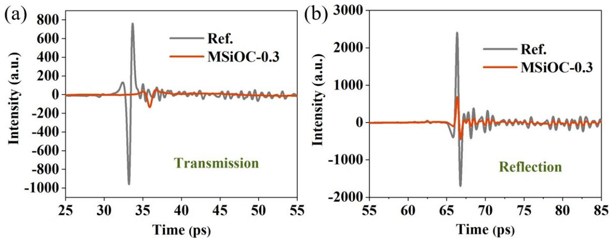
Fig. S3 Time-domain spectra of  $\text{Ti}_3\text{C}_2\text{T}_x$  MXene/SiOC-0.3 composite in (a) transmission and (b) reflection mode.
