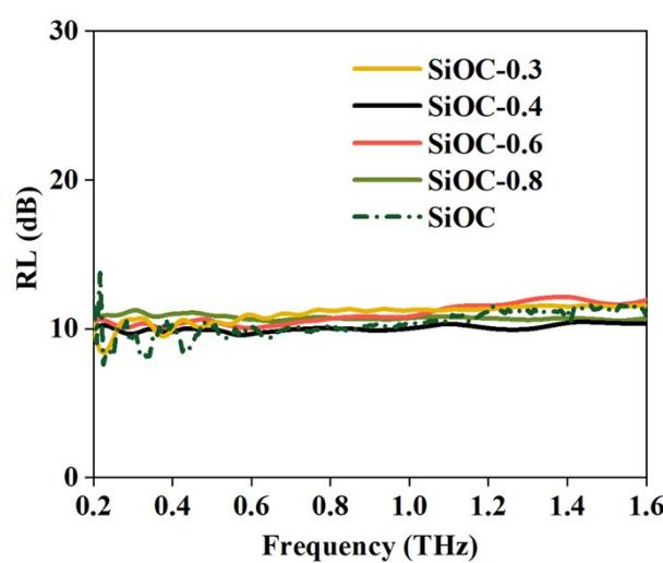
Fig. S5 The reflection loss (RL) of SiOC and Ti<sub>3</sub>C<sub>2</sub>T<sub>x</sub> MXene/SiOC ceramic composite
