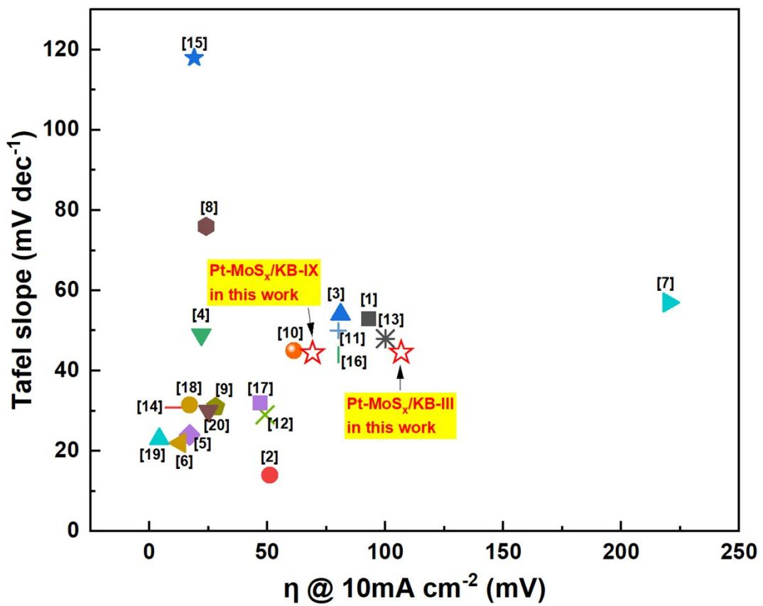
**Fig. S15** The comparison of the  $\eta_{10}$  and the Tafel slope of the as-synthesized Pt-MoS<sub>x</sub>/KB-III, Pt-MoS<sub>x</sub>/KB-IX in this work and the state-of-the-art analogous catalysts reported in recent years.
