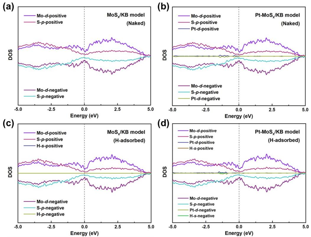
**Fig. S14** The PDOS in Site 1 of (a) naked  $\text{MoS}_x/\text{KB}$ , (b) naked  $\text{Pt}-\text{MoS}_x/\text{KB}$ , (c) H-adsorbed  $\text{MoS}_x/\text{KB}$  and (d) H-adsorbed  $\text{Pt}-\text{MoS}_x/\text{KB}$  models.
