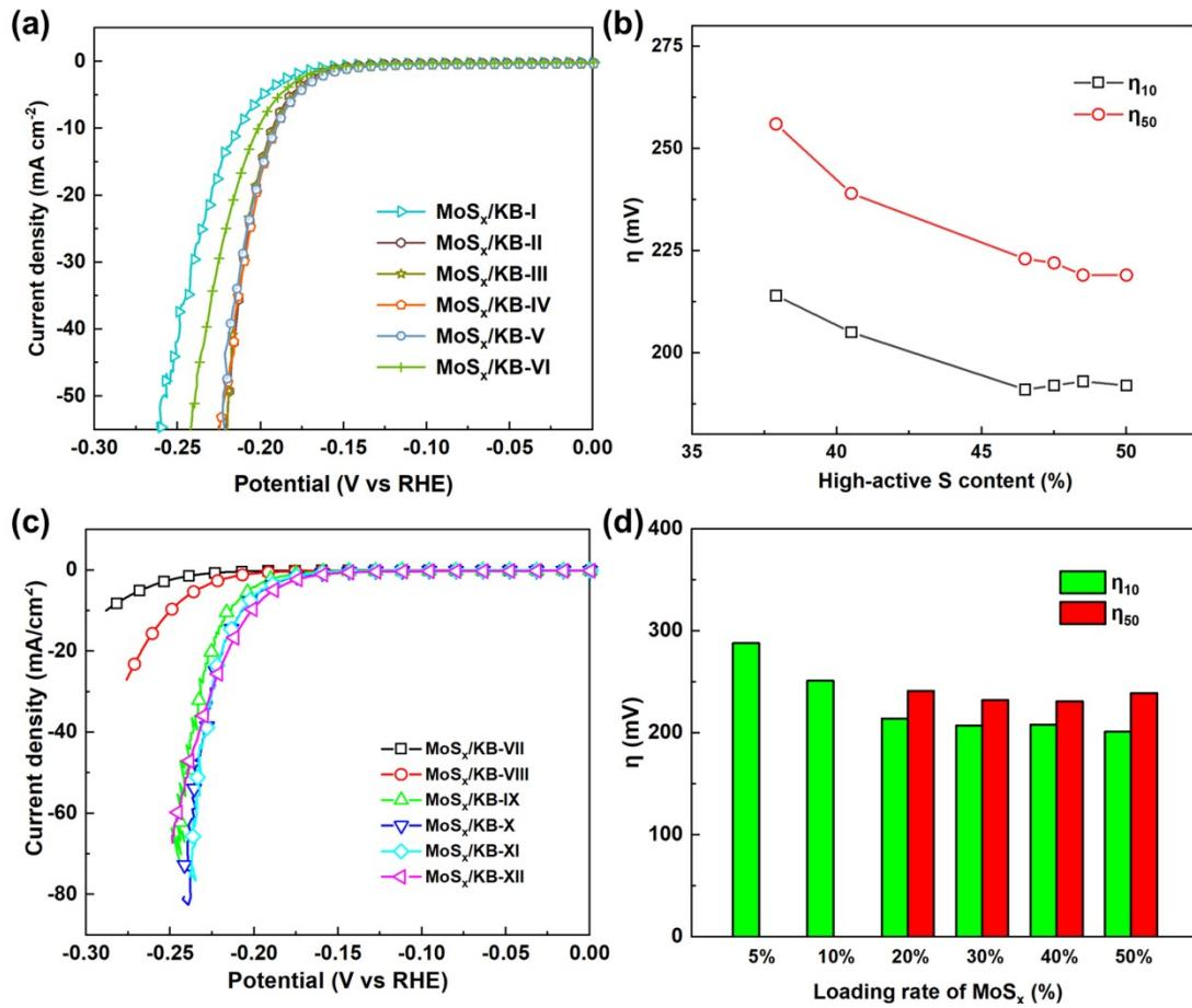
**Fig. S7** (a) LSV curves of the  $\text{MoS}_x/\text{KB}$ s with different high-active S contents and (b) their corresponding  $\eta$  values; (c) LSV curves of the  $\text{MoS}_x/\text{KB}$ s with different  $\text{MoS}_x$  loading rates and (d) their corresponding  $\eta$  values.
