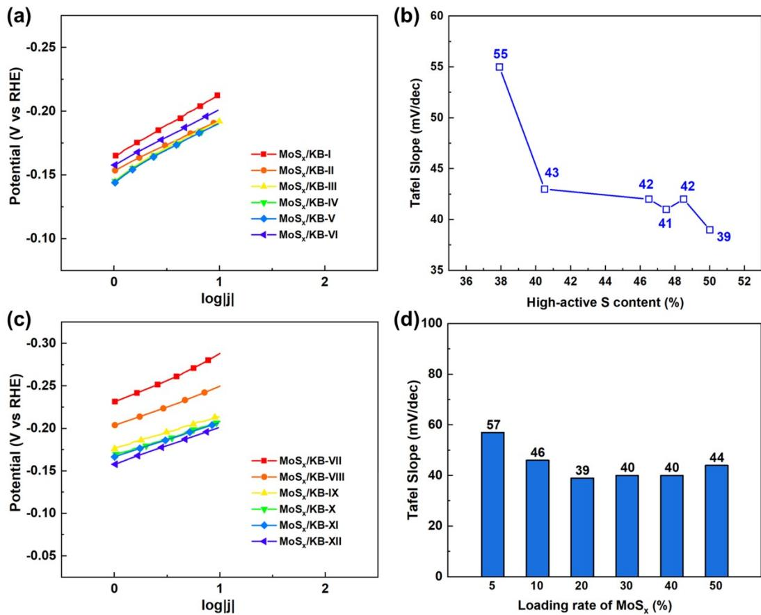
**Fig. S8** (a) Tafel curves of  $\text{MoS}_x/\text{KBs}$  with different high-active S contents and (b) their corresponding Tafel slope values; (c) Tafel curves of  $\text{MoS}_x/\text{KBs}$  with different  $\text{MoS}_x$  loading rates and (d) their corresponding Tafel slope values.
