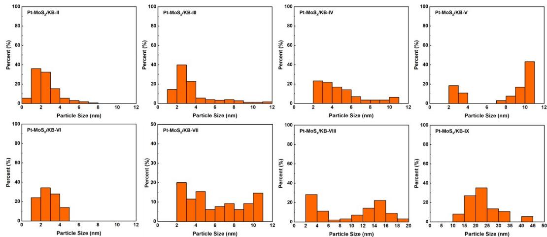
**Fig. S5** The particle size distribution of Pt NPs in the as-synthesized Pt-MoS<sub>x</sub>/KBs, which is calculated from their corresponding TEM images.
