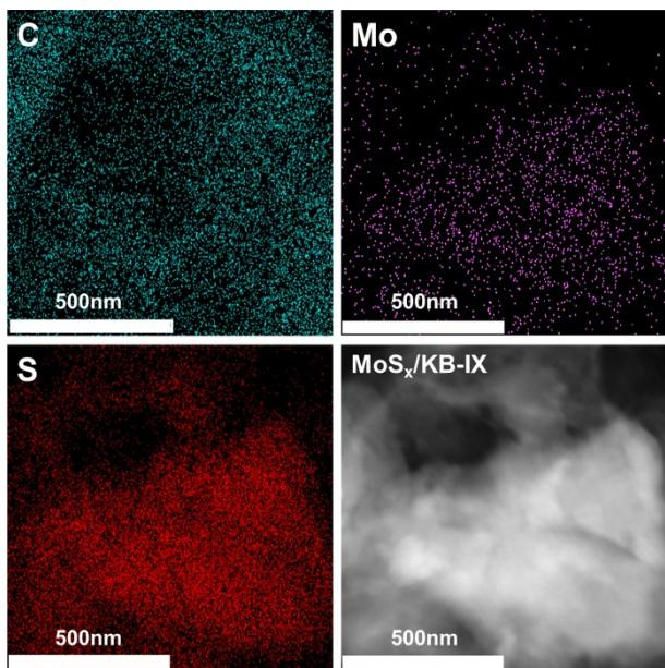
**Fig. S3** the STEM-EDS mapping image of  $\text{MoS}_x/\text{KB-IX}$ .
