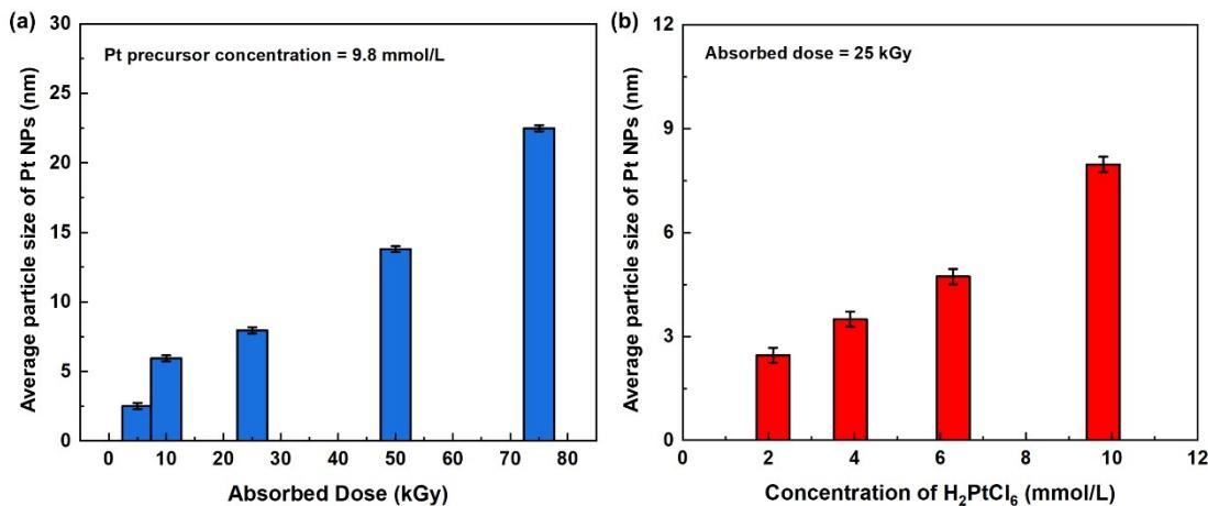
**Fig. S6** The average-particle size of Pt NPs in the as-synthesized Pt-MoS<sub>x</sub>/KBs under different absorbed doses (a) and different concentrations of H<sub>2</sub>PtCl<sub>6</sub> precursor (b).
