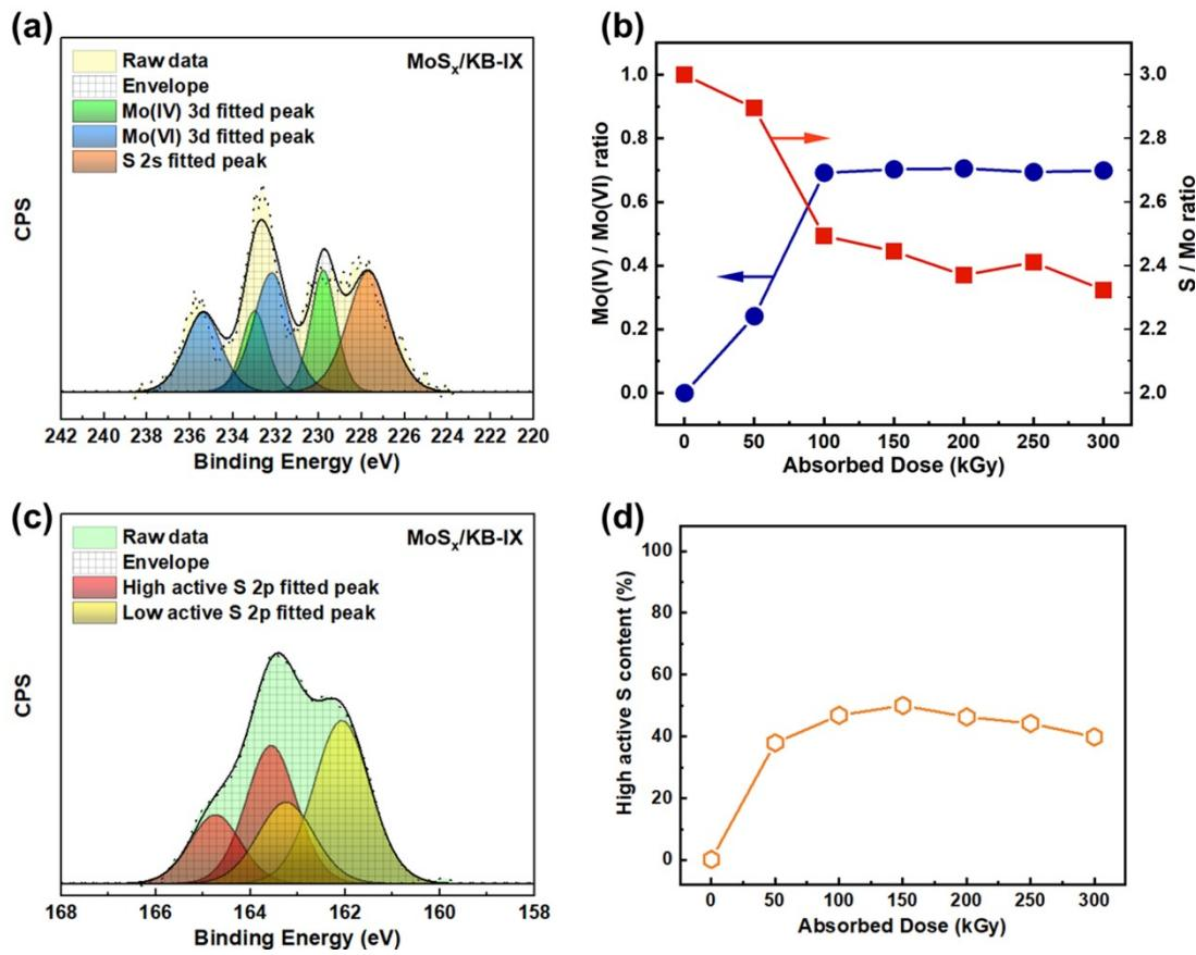
**Fig. S1** (a) The deconvoluted Mo 3d high-resolution X-ray photoelectron spectrum of  $\text{MoS}_x/\text{KB-IX}$ ; (b) The relationship curve of the Mo(IV)/Mo(VI) ratio and S/Mo ratio of  $\text{MoS}_x/\text{KB}$  catalysts with absorbed dose; (c) The deconvoluted S 2p high-resolution X-ray photoelectron spectrum of  $\text{MoS}_x/\text{KB-IX}$ ; (d) The relationship curve of the high active S content of  $\text{MoS}_x/\text{KB}$  catalysts with absorbed dose.
