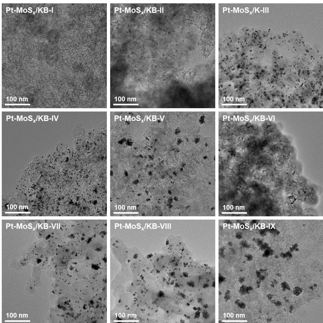
**Fig. S4** The TEM image comparison of the as-synthesized  $\text{Pt}-\text{MoS}_x/\text{KBs}$ .
