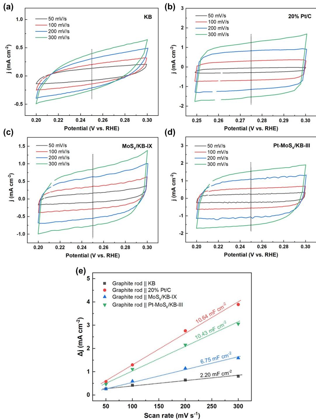
**Fig. S9** CV curves of (a) KB, (b) 20% Pt/C, (c)  $\text{MoS}_x/\text{KB-IX}$ , and (d)  $\text{Pt-MoS}_x/\text{KB-III}$  catalysts measured at different scan rates. (e) Current density differences plotted against scan rates.
