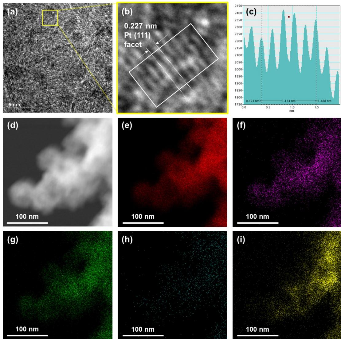
**Fig. S11** (a) HR-TEM image of Pt-MoS<sub>x</sub>/KB-III after 48h HER running at current density of 20 mA cm<sup>-2</sup>. (b) The selected area for statistical crystal facet parameter of platinum and (c) the statistical result in (a). (d) STEM image and EDS mapping of (e) C, (f) Pt, (g) S, (h) Mo, and (i) F elements of Pt-MoS<sub>x</sub>/KB-III after 48h HER running at current density of 20 mA cm<sup>-2</sup>.
