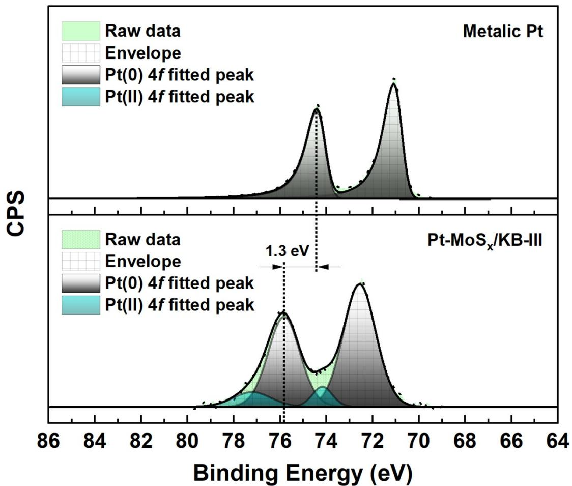
**Fig. S2** Comparison of deconvoluted Pt 4f high-resolution XPS spectra of metallic Pt and Pt-MoS<sub>x</sub>/KB-III.
