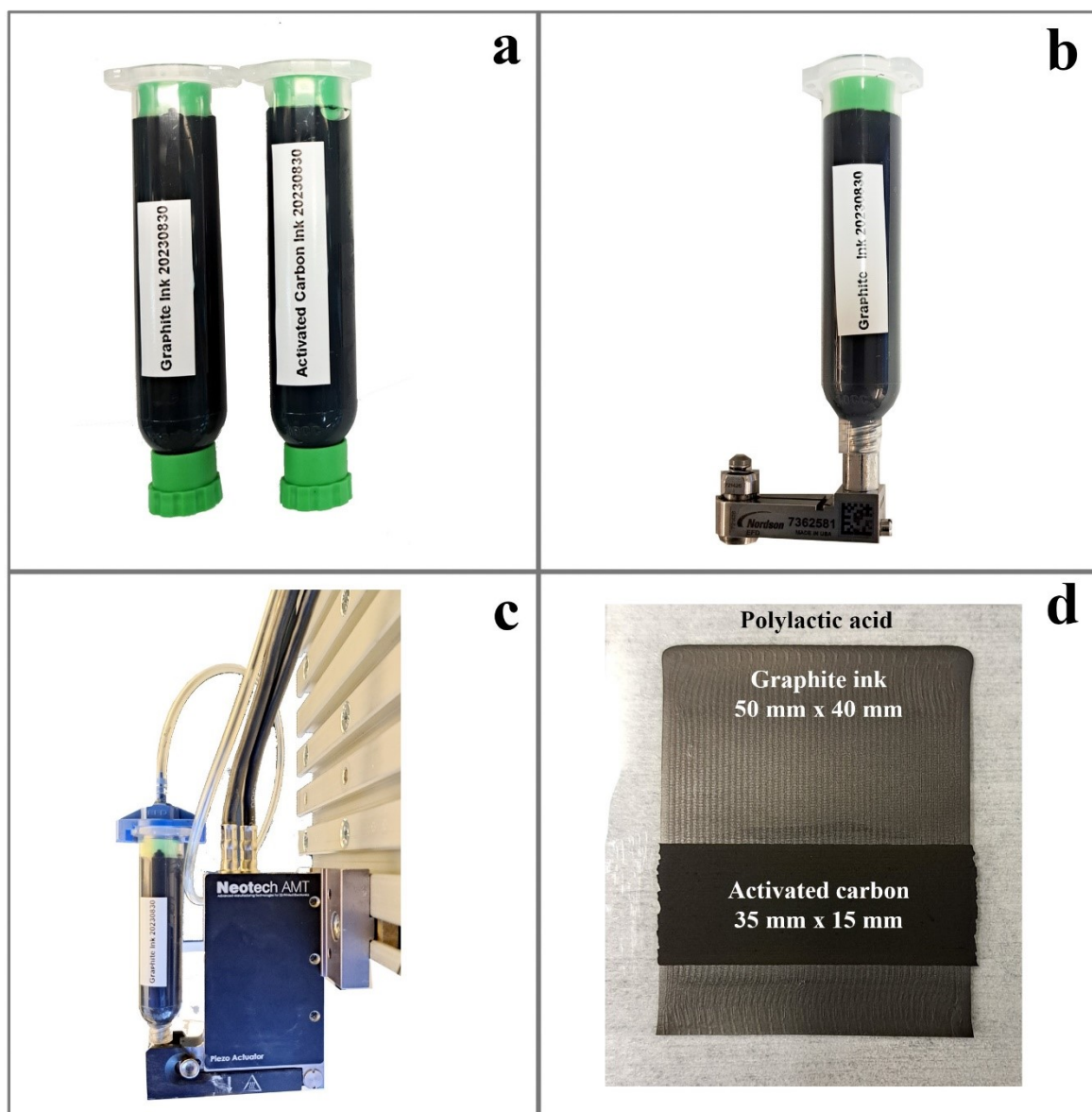
Fig. S2 Images of (a) graphite and activated carbon inks, (b) ink with a fluid body, (c) Piezo jet module fitted with ink, (d) printed graphite ink (current collector) and printed DPBAC (electrode) on polylactic acid (substrate)
