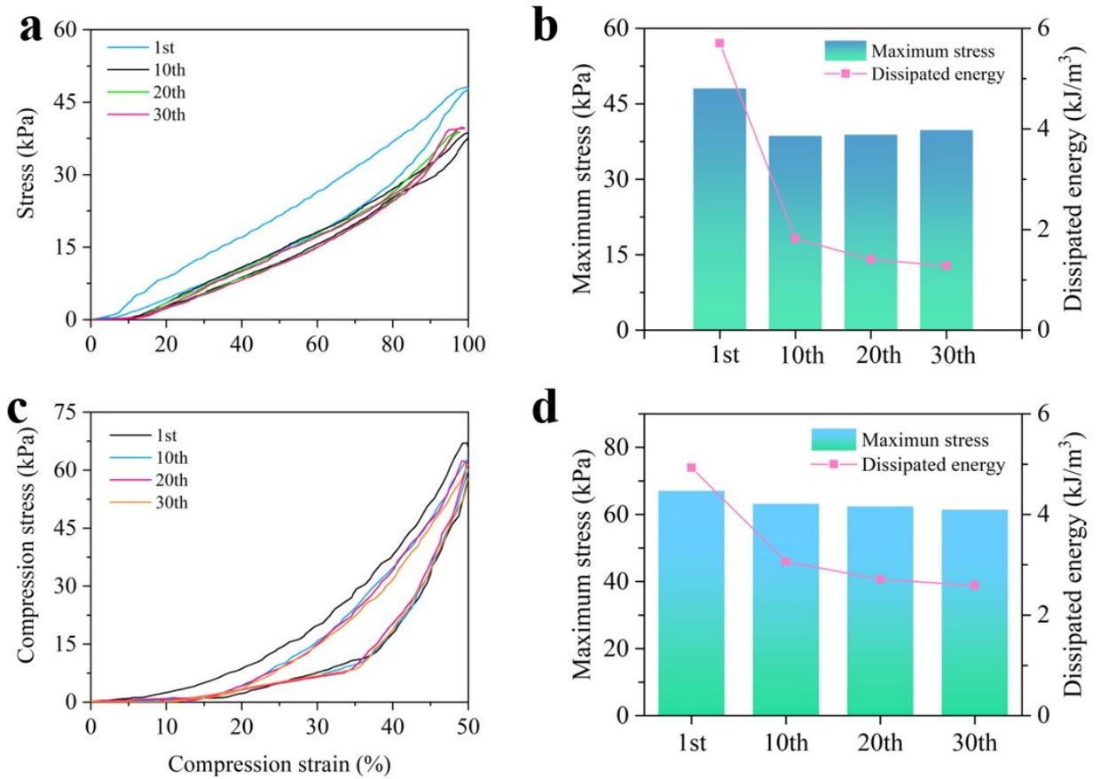
**Figure S1.** (a) Loading/unloading curves of hydrogel at 100% tensile strain for 30 consecutive cycles. (b) Cyclic loading/unloading energy dissipation at 100% tensile strain. (c) Loading/unloading curves of hydrogel at 50% compressive strain for 30 consecutive cycles. (d) Loading/unloading energy dissipation at 50% compressive strain.
