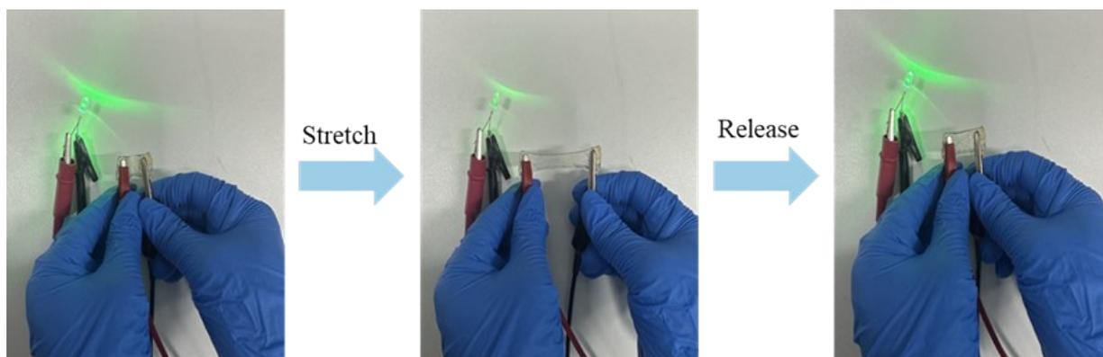
**Figure S4.** Schematic diagram of the effect of hydrogel stretching on the brightness variation of LED bulbs.
