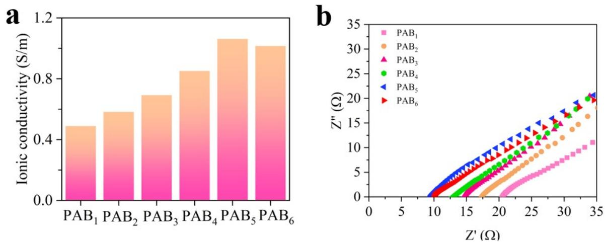
**Figure S2.** (a) Ionic conductivity of hydrogels with different SBMA contents. (b) Electrochemical impedance spectroscopy (EIS) of hydrogels with different SBMA contents.
