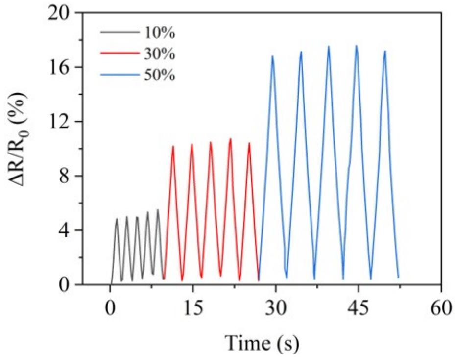
**Figure S3.** Repeated response curves of PABC strain sensor under different strains.
