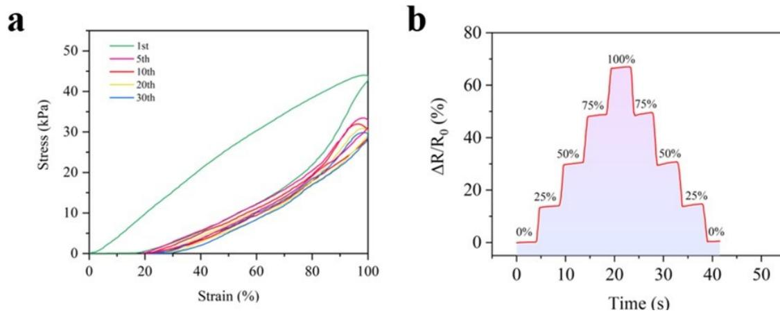
**Figure S6.** (a) Loading/unloading curves of hydrogels immersed for five days at 100% tensile strain for 30 consecutive cycles. (b) Tensile release response curves of hydrogels in the 0-100% strain range after five days of immersion.
