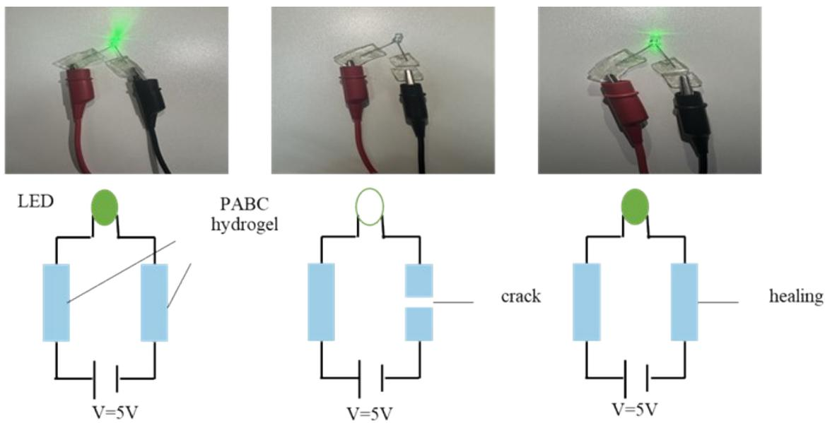
**Figure S5.** Brightness change of LED bulb after cutting and self-healing hydrogel connected to a circuit.
