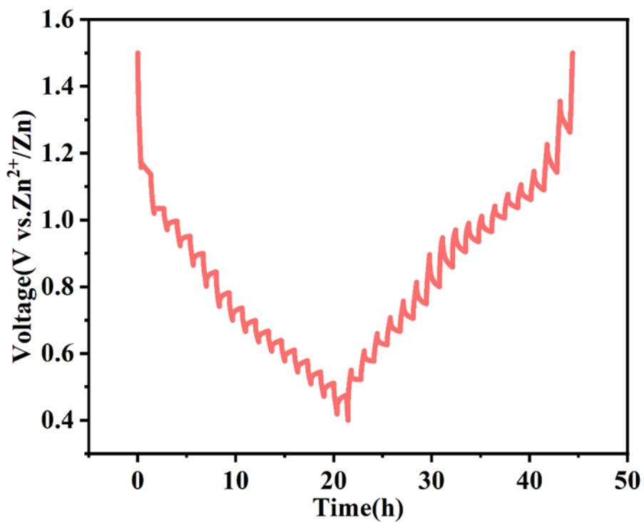
**Fig. S6** Charge-discharge GITT profiles of SNVO.
