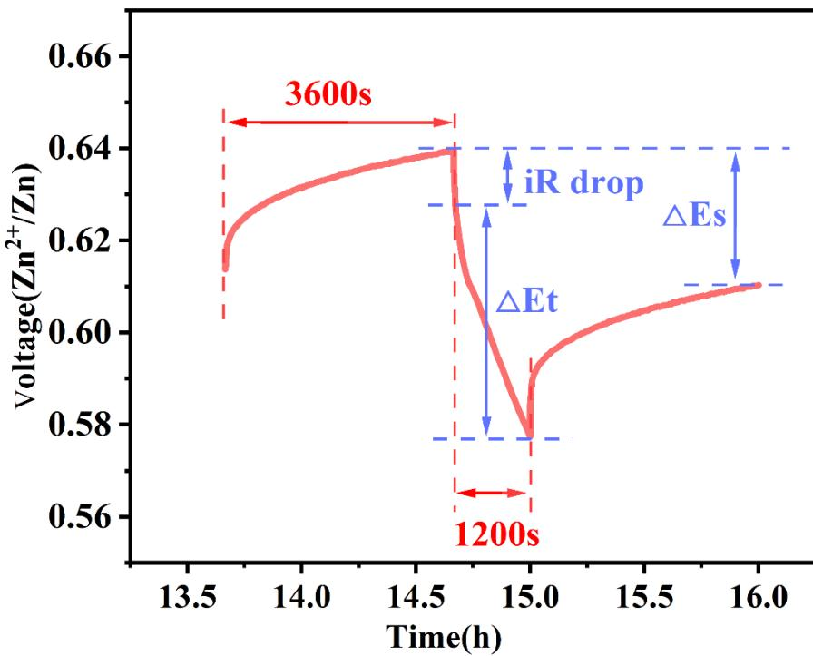
**Fig. S7** Local diagram of GITT discharge curve of SNVO electrode.
