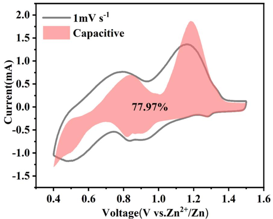
**Fig. S5 Capacitance contribution at  $1 \text{ mV s}^{-1}$  of SNVO.**
