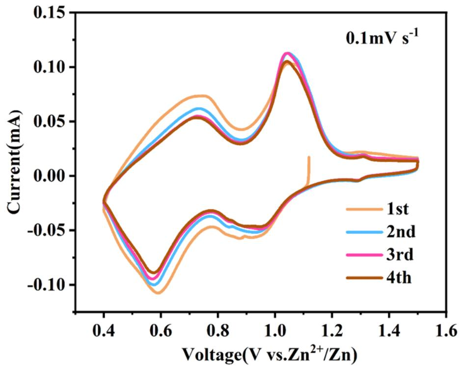
**Fig. S2** CV curves of NVO cathode at 0.1 mV s<sup>-1</sup>.
