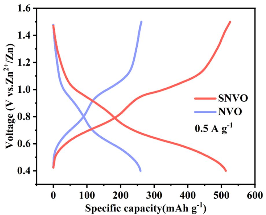
**Fig. S3** Curves of galvanostatic charge/discharge at 0.5 A g<sup>-1</sup>.
