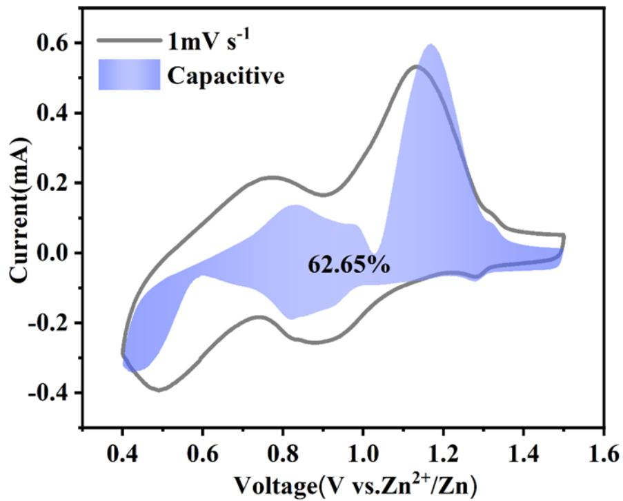
**Fig. S4** Capacitance contribution at  $1 \text{ mV s}^{-1}$  of NVO.
