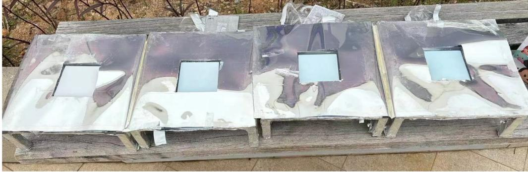
Figure S6 Photographs of the apparatus for outdoor tests of radiative cooling performance.
