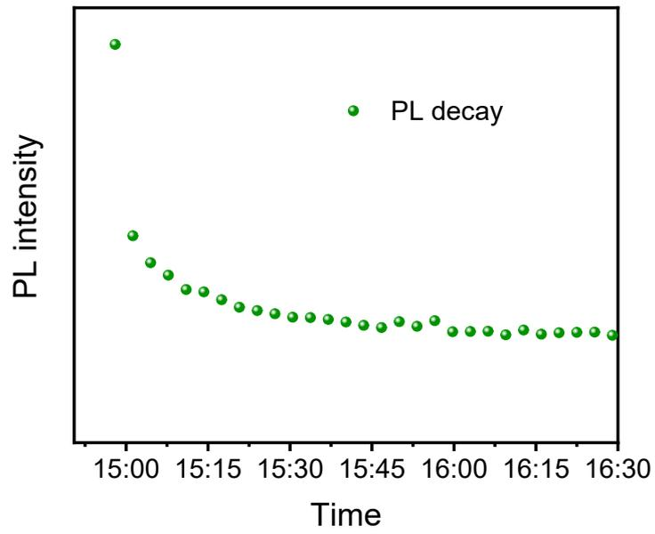
Figure S5 The photoluminescent lifetime of the SrO·Al<sub>2</sub>O<sub>3</sub>: Eu phosphor.
