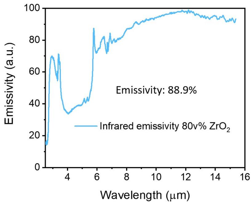
Figure S4 Infrared emissivity of the white coating with ZrO<sub>2</sub> volume fraction of 80v%.
