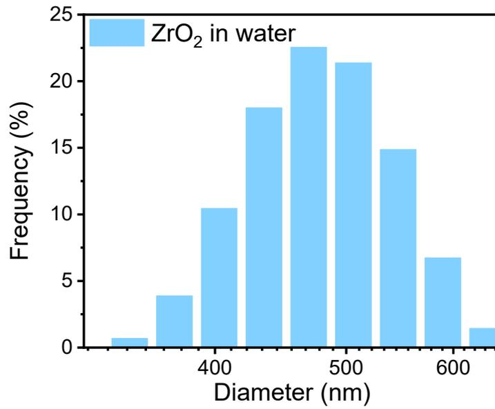
Figure S3 Size distribution of ZrO<sub>2</sub> nanoparticles monodispersed in water.
