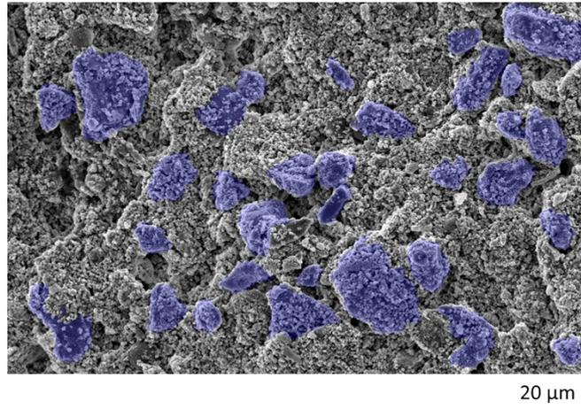
Figure S1 SEM image of the top layer in the light-blue coating.
