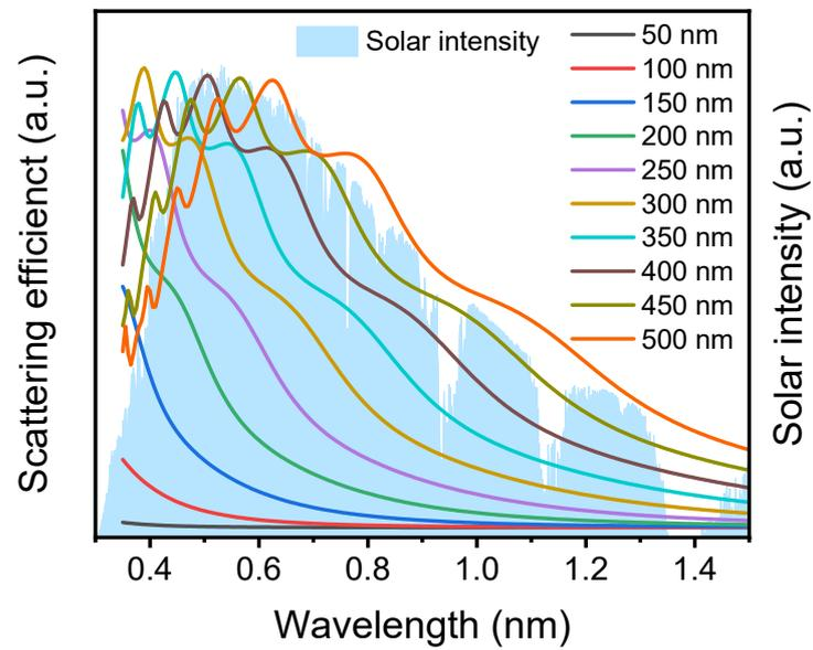
Figure S2 Stimulated scattering spectra of ZrO<sub>2</sub> nanoparticles with varied diameters and solar intensity spectrum.
