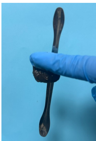
Fig. S2. The photograph of eutectogel adhering to steel after multiple cycles
