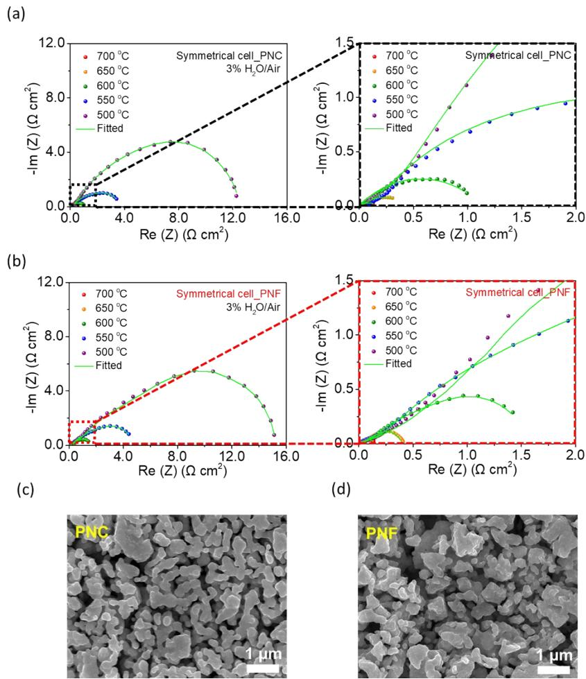
**Fig. S5.** EIS and fitted spectra of the BZCYYb4411-based symmetrical cells with the (a) PNC and (b) PNF air electrodes under open circuit voltage in temperature ranges of 500 to 700 °C in wet air ( $p_{\text{H}_2\text{O}}=0.03$  atm). Microstructures of the (c) PNC and (d) PNF air electrodes after sintering at 950 °C for 4 h in air atmosphere.
