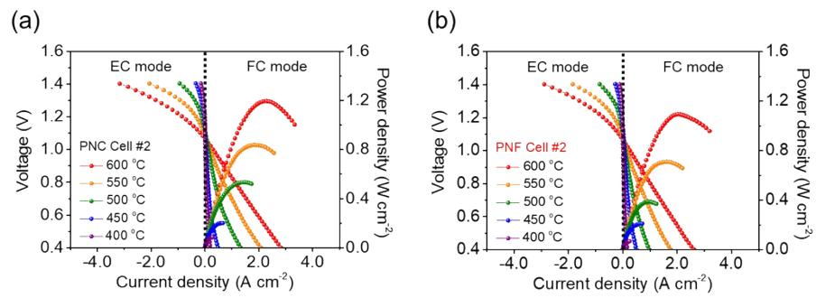
**Fig. S8.**  $I$ - $V$  and  $I$ - $P$  curves of the R-PCC single cells for #2 with (a) PNC and (b) PNF. Good reproducibility is obtained across the duplicate cells.
