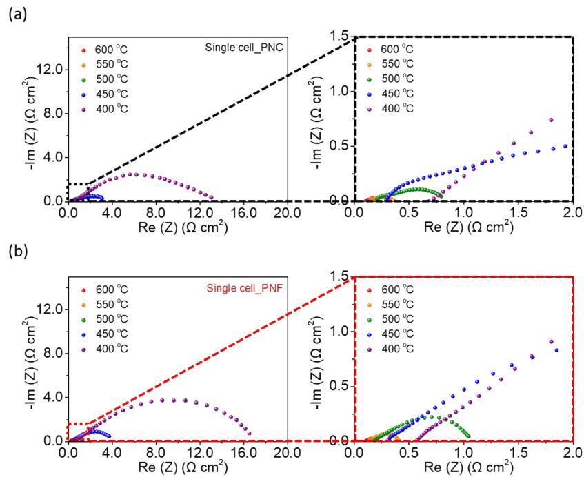
**Fig. S7.** EIS of the single cells with the (a) PNC and (b) PNF air electrodes under open circuit voltage in temperature ranges of 400 to 600 °C.
