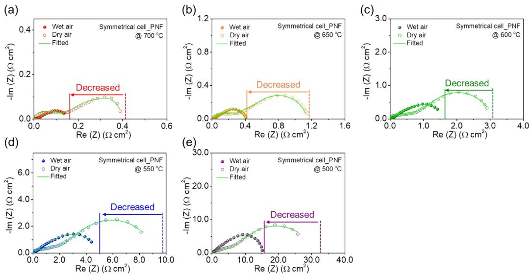
**Fig. S6.** EIS of the BZCYYb4411-based symmetrical cells with the PNF air electrode under open circuit voltage in temperature ranges of 500 to 700 °C in dry and wet air ( $p\text{H}_2\text{O}=0.03$  atm).
