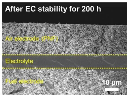
**Fig. S9.** Cross-sectional SEM images of PNF air electrode based R-PCC single cell following the EC stability for 200 h. No discernible microstructural changes were observed in R-PCC with the PNF air electrode before (**Fig. 5a**) and after EC stability measurement, particularly at the interfaces between the electrode and electrolyte.
