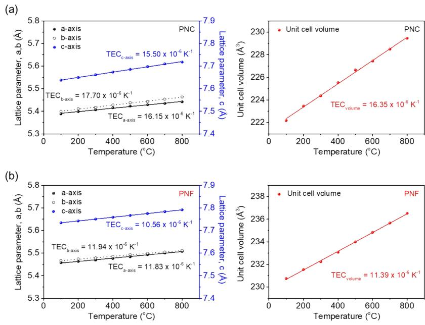
**Fig. S3.** (a) Lattice parameter changes and calculated TEC values of the PNC air electrode (b) Lattice parameter changes and calculated TEC values of the PNF air electrode at temperatures ranging from 100 to 800 °C.
