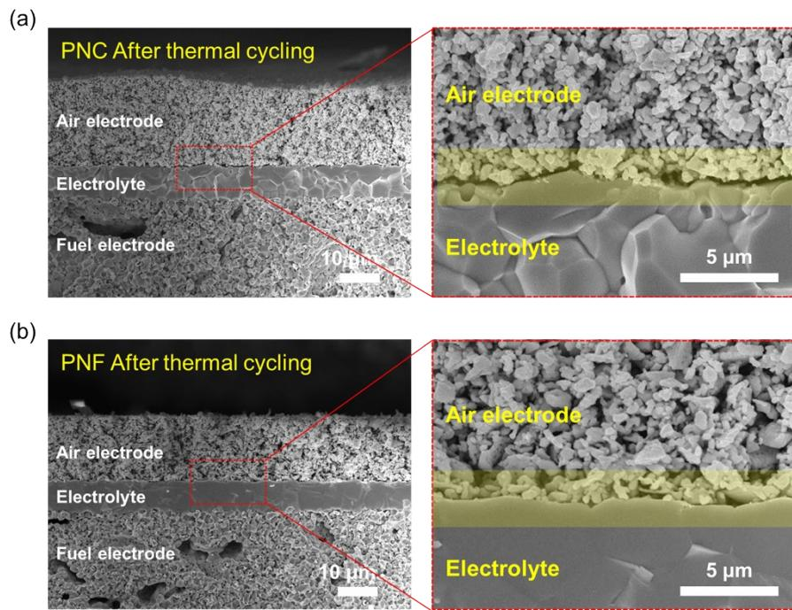
**Fig. S11.** After thermal cycling stability of single cells with the (a) PNC and (b) PNF air electrode.
