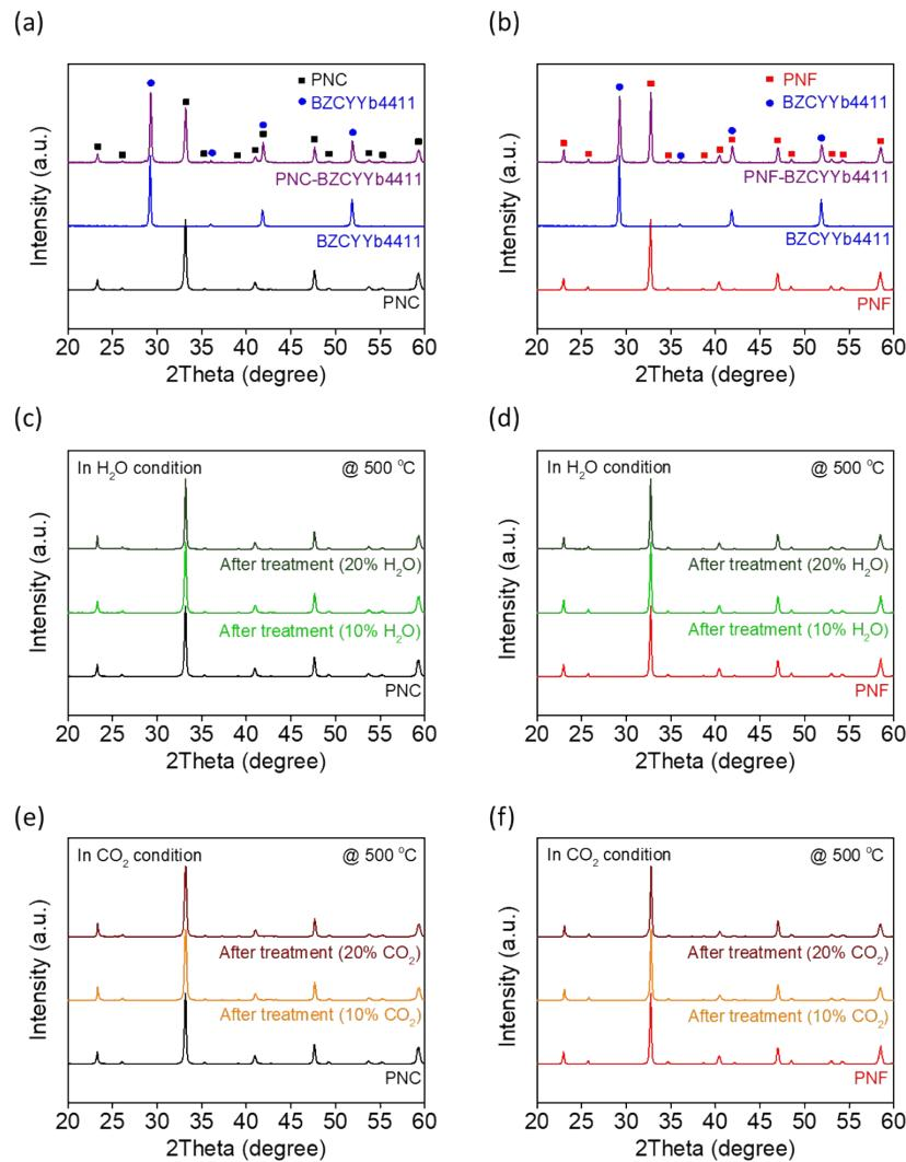
**Fig. S1.** Chemical compatibility between the (a) PNC and (b) PNF air electrode and BZCYYb4411 electrolyte after annealing at 950 °C for 4 h in air atmosphere. Post-treated the (c) PNC and (d) PNF air electrode after exposing to 10 and 20% H<sub>2</sub>O. Post-treated the (e) PNC and (f) PNF air electrode after exposing to 10 and 20% CO<sub>2</sub> at 500 °C for 24 h.
