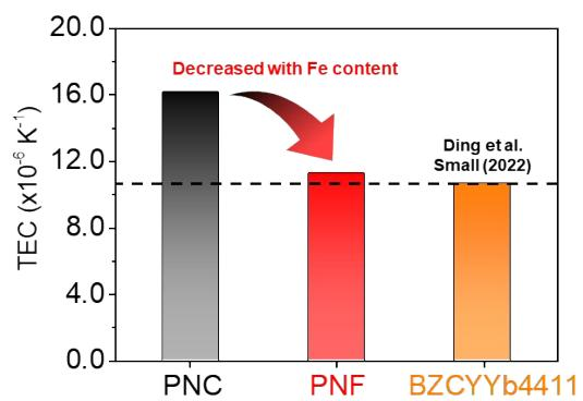
**Fig. S10.** Calculated TEC values of the PNC and PNF air electrodes from 200 to 900 °C and BZCYYb4411 electrolyte from 100 to 1000 °C.
