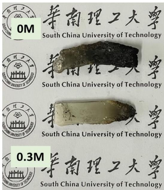
**Figure S5.** Photograph of the comparison of residues of PAA-PEO-0M and PAA-PEO-0.3M ionic hydrogels after vertical combustion.
