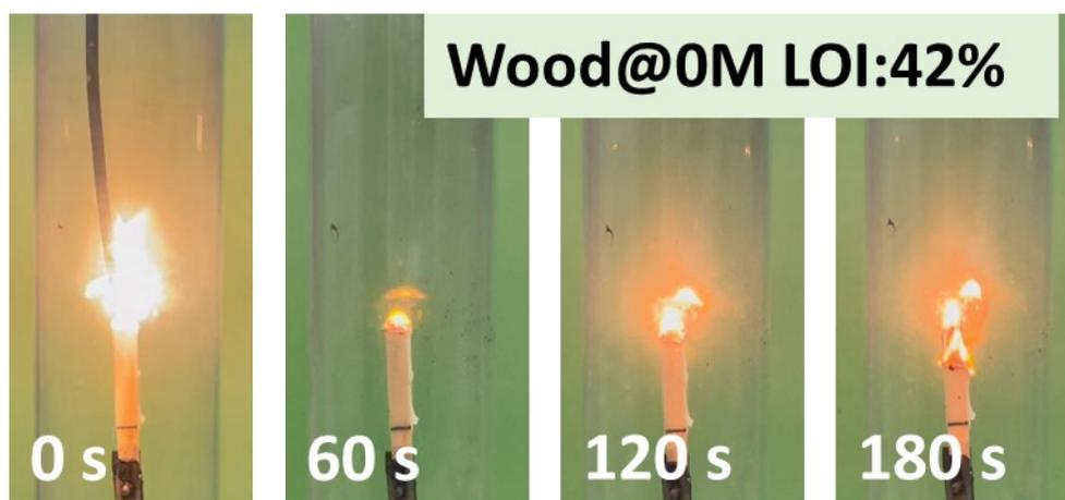
**Figure S6.** The screenshots from a video of wood@0M burning in an atmosphere with 42% oxygen.
