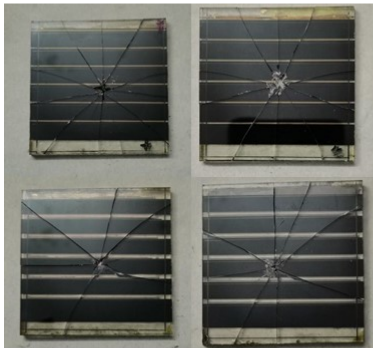
Figure S8 Photographs of damaged devices in lead leakage test.
