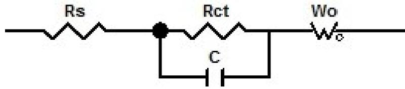
**Fig. S2** The electrical equivalent circuit for the calculation of the resistances.
