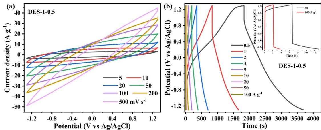
**Fig. S9** (a) CV curves at different scan rates and (b) GCD curves at different current density of the three-electrode system using DES-1-0.5 electrolyte.
