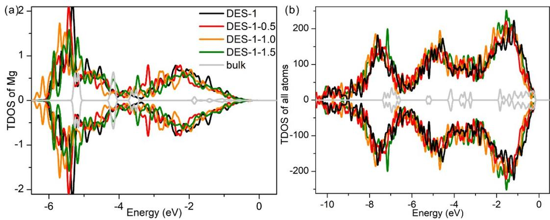
**Fig. S7.** The total density of states (TDOS). (a) TDOS of all Mg atoms, and (b) TDOS of all atoms in DES-1, DES-1-0.5, DES-1-1.0 and DES-1-1.5.
