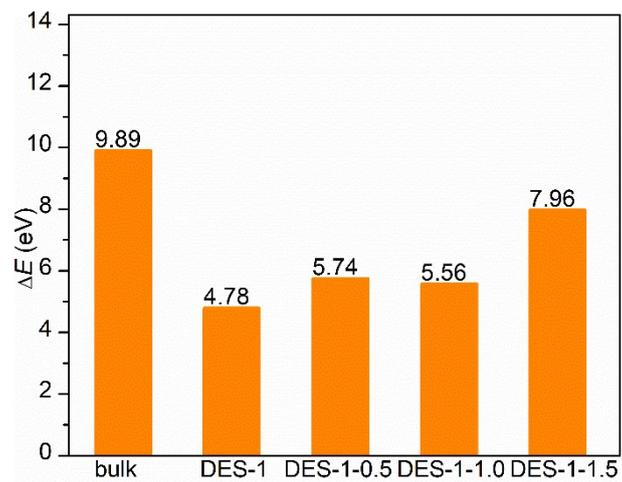
**Fig. S8.** The energy required to remove the  $\text{MgCl}_2$  unit in DES-1, DES-1-0.5, DES-1-1.0 and DES-1-1.5.
