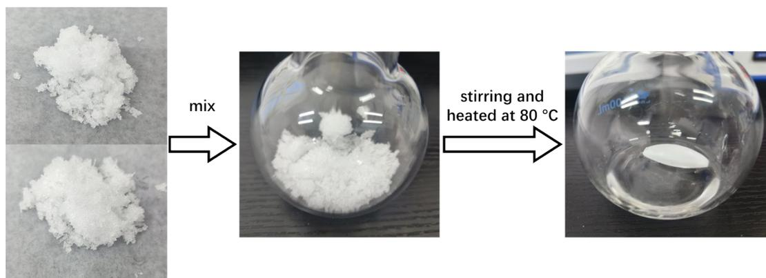
**Fig. S3** Schematic illustration of the synthesis processes of DES electrolytes.
