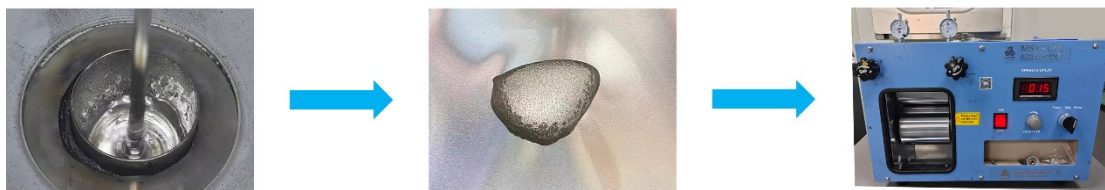
Figure S2 Digital photographs of the process of preparing Li-Ag alloy foil.
