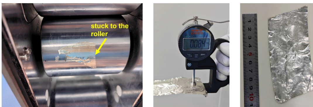
Figure S4 (a) Digital photographs of Li-Ag alloy foil with different thicknesses. (b) Digital photographs of bare Li foil stuck to the stainless-steel roller with a thickness below 100 \mu\text{m} .
