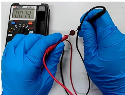
**Fig. S5.** Resistance test of Ag-CuNW/MWCNT@MF.
