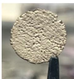
**Fig. S6.** Ag-CuNW/MWCNT@MF electrode after deposition of  $90 \text{ mAh cm}^{-2}$  Li.
