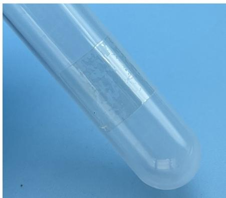
**Fig. S5** Photograph of the cross-linked silk film conformably attached to a curved surface.
