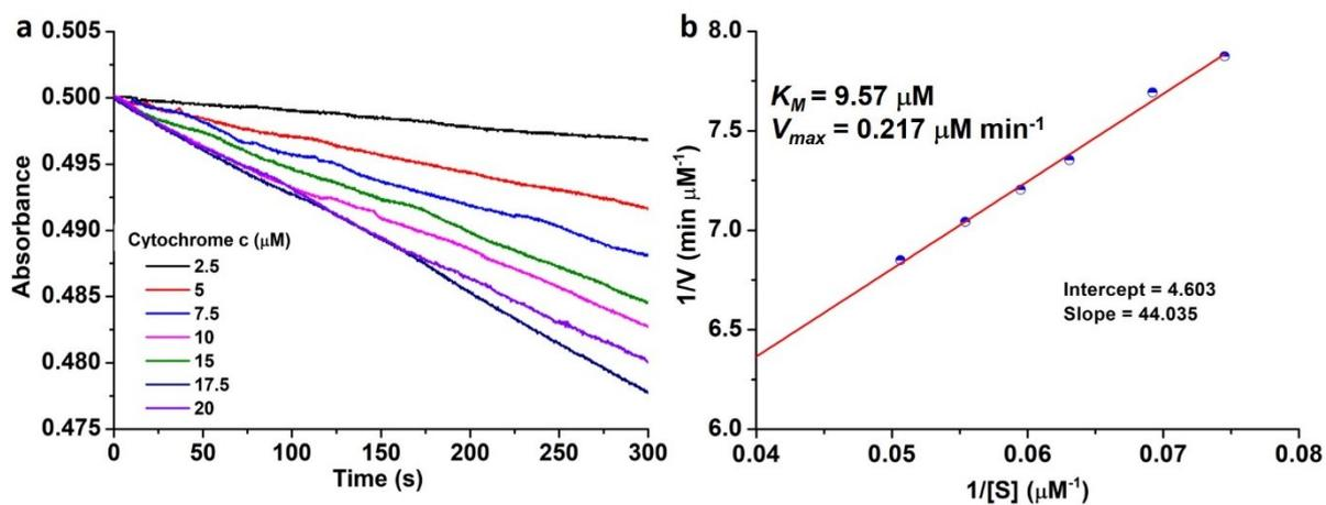
**Figure S4.** a) Time-dependent absorbance spectra for the CcO-like activity of Cu-Phen at different concentrations of cyt c; b) Lineweaver-Burk plot obtained by plotting  $1/V$  versus  $1/\text{cyt c}$  concentration.
