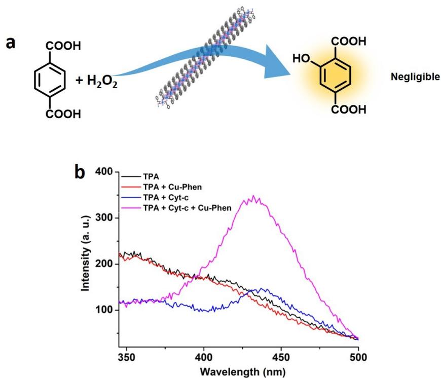
**Figure S9.** **a)** Scheme showing the reaction of terephthalic acid with the hydroxyl radical generated during the CcO-like activity of Cu-Phen to form fluorescent product, hydroxy terephthalic acid; **b)** Fluorescence spectra showing the formation of hydroxy terephthalic acid during the CcO-like activity of Cu-Phen.
