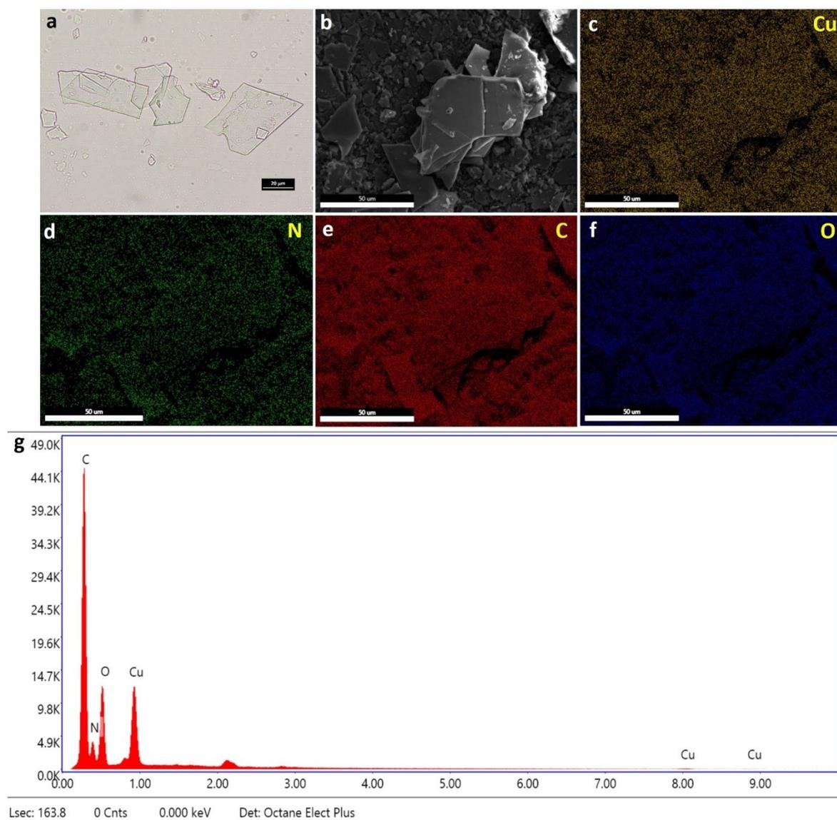
**Figure S1.** **a)** Optical microscope image of Cu-Phen; **b)** SEM image of Cu-Phen showing the area used for elemental X-ray mapping of; **c-f)** Cu, N, C and, O; **g)** EDX spectrum of Cu-Phen.
