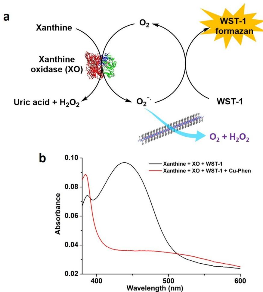
**Figure S12.** **a)** Scheme showing the assay conditions used for monitoring superoxide scavenging activity of Cu-Phen; **b)** Absorbance spectra showing the production of WST-1 formazan upon reaction with superoxide radical, and inhibition of WST-1 formazan production due to superoxide scavenging activity of Cu-phen.
