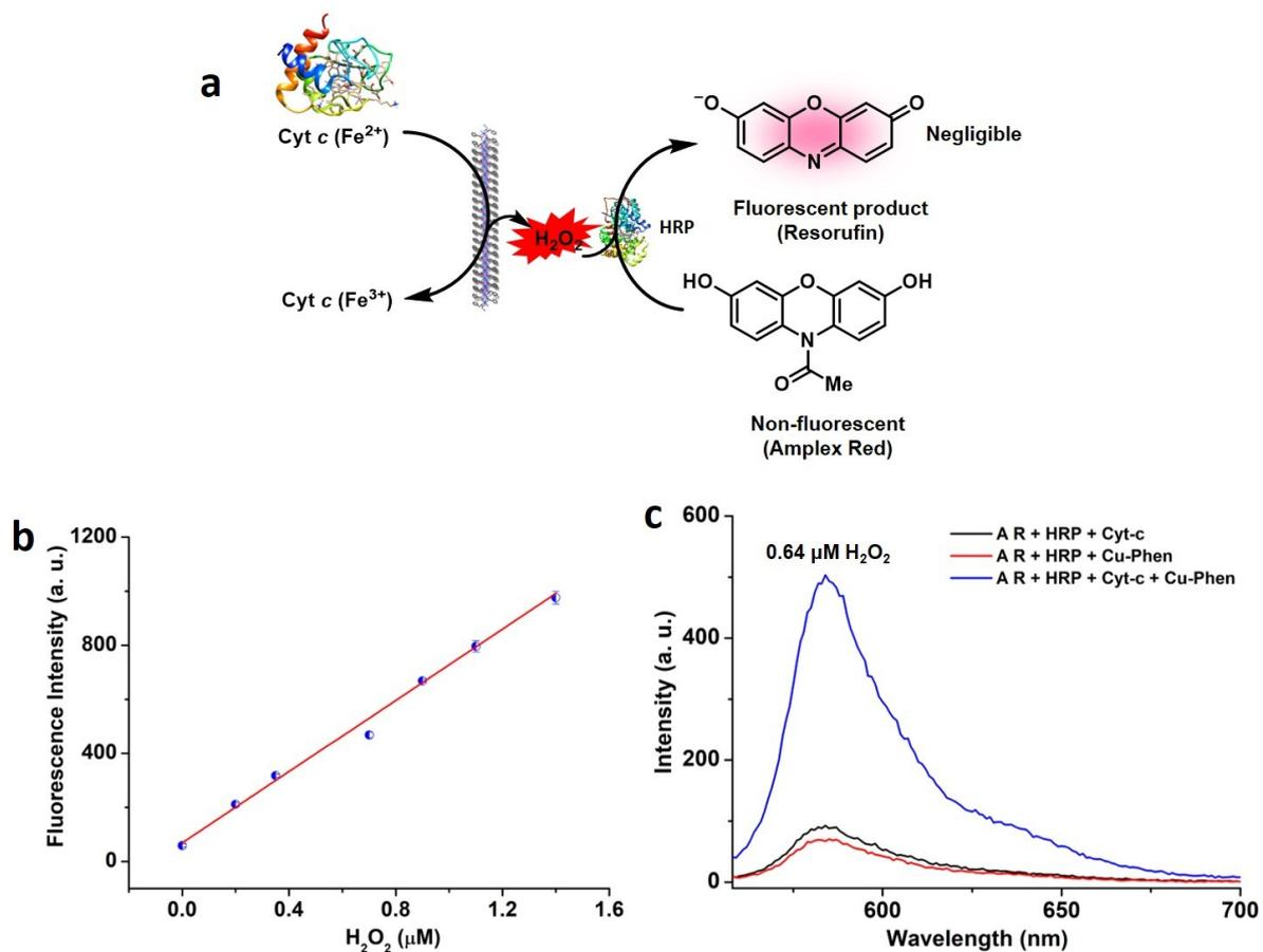
**Figure S8. a)** Scheme showing the production of H<sub>2</sub>O<sub>2</sub> during the CcO-like activity of Cu-Phen, and its detection by amplex red; **b)** Calibration curve for finding the concentration of H<sub>2</sub>O<sub>2</sub> produced during the CcO-like activity of Cu-Phen; **c)** Fluorescence spectra for detection of H<sub>2</sub>O<sub>2</sub> using amplex red assay.
