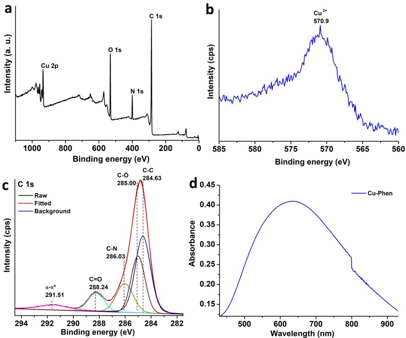
**Figure S2.** a) Survey XPS spectrum of Cu-Phen; b) Cu-LMM spectrum; c) C1s XPS spectra of Cu-Phen; d) Solid state UV-DRS spectrum of Cu-Phen.
