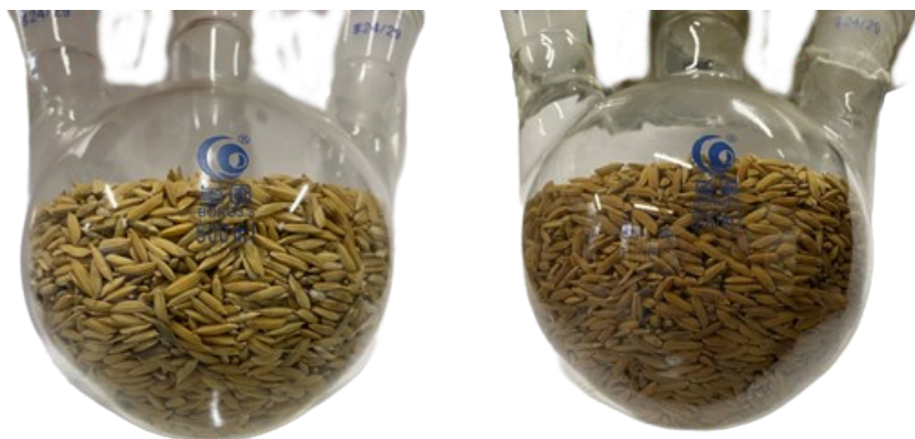
Figure S4 The external physical map of rice before smoldering, uncarbonized (left); External physical map of rice after smoldering, carbonization (right).
