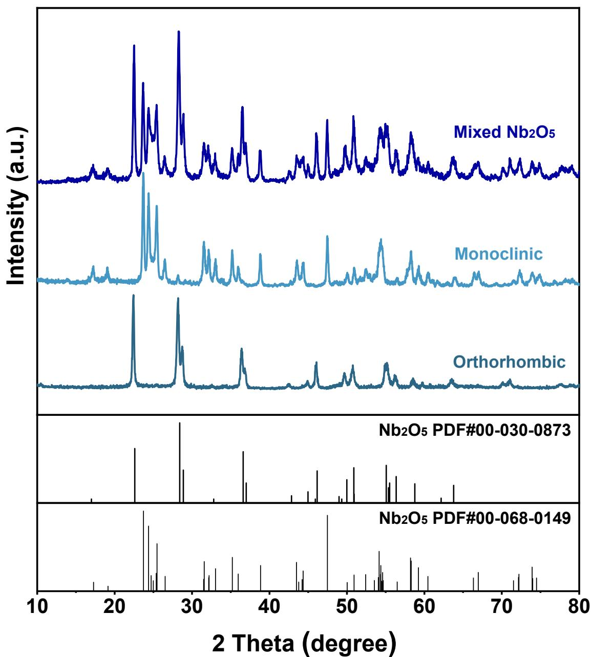
**Figure S1.** XRD patterns of synthesized  $\text{Nb}_2\text{O}_5$  with monoclinic, orthorhombic, and mixed monoclinic-orthorhombic phases.
