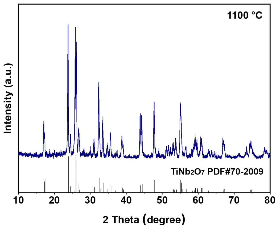
**Figure S4.** XRD patterns of the  $\text{TiNb}_2\text{O}_7$  synthesized from the  $\text{Nb}_2\text{O}_5$  precursor with mixed monoclinic-orthorhombic phases at the synthesis temperatures of  $1100\text{ }^\circ\text{C}$ .
