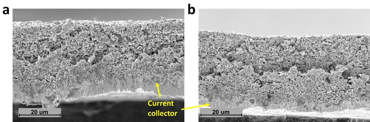
**Figure S9.** Cross-sectional SEM images of OD-TNO electrodes with (a) PVDF and (b) Li-PAA binders coated on copper current collector.
