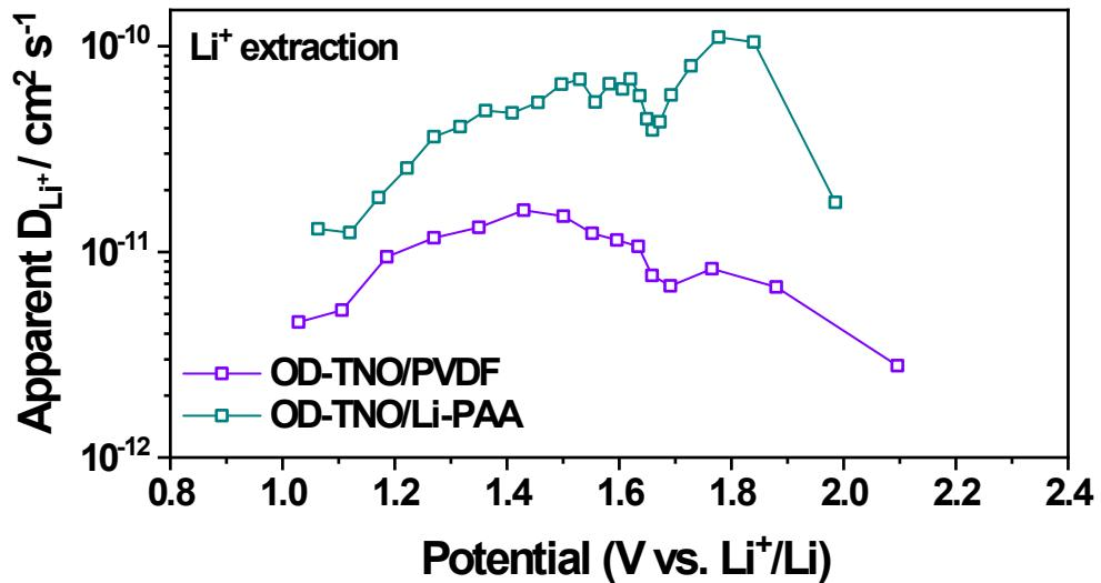
**Figure S14.** Lithium diffusion coefficients during delithiation process in OD-TNO/PVDF and OD-TNO/Li-PAA.
