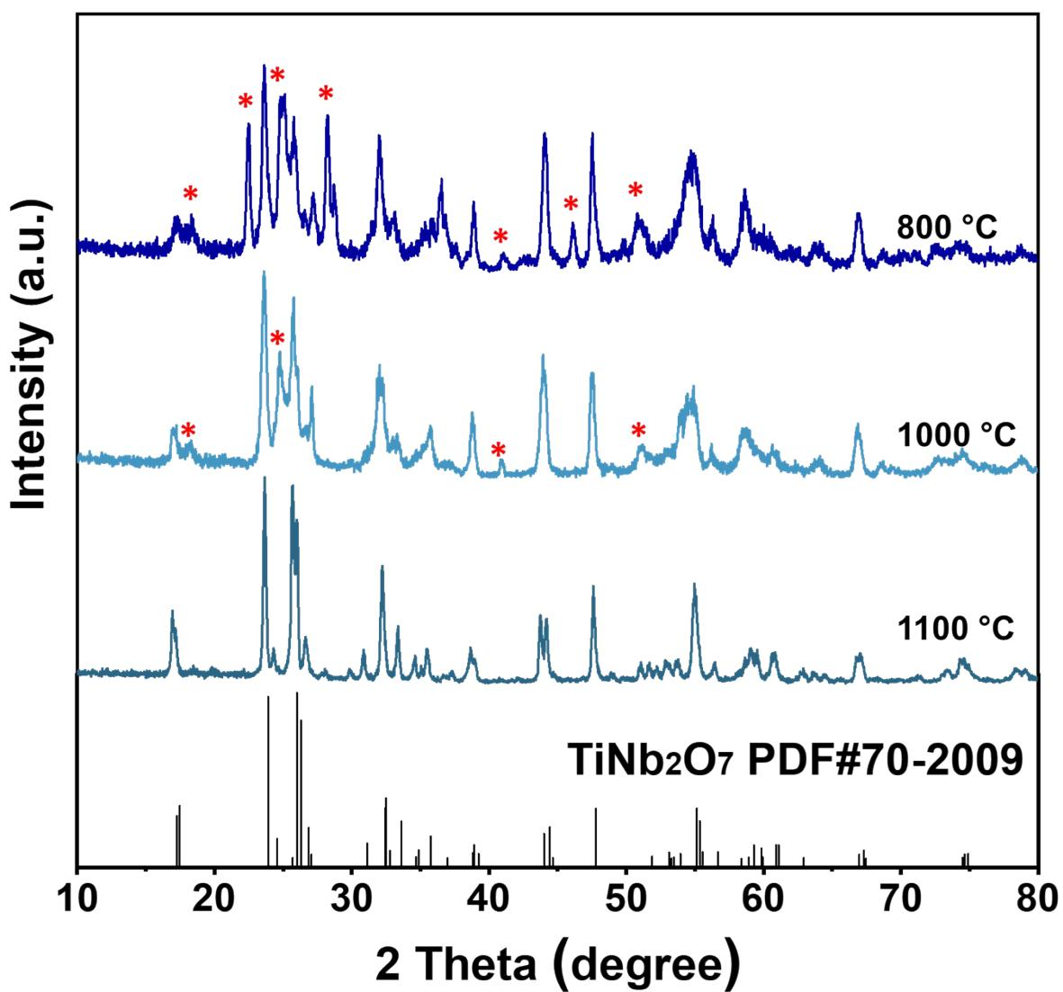
**Figure S2.** XRD patterns of the  $\text{TiNb}_2\text{O}_7$  synthesized from the orthorhombic  $\text{Nb}_2\text{O}_5$  precursor at synthesis temperatures of 800, 1000, 1100 °C, with impurities marked with red asterisks.
