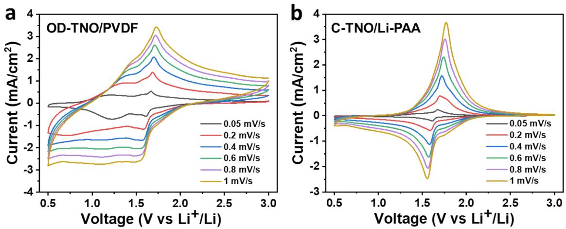
**Figure S15.** CV curves for a) OD-TNO/PVDF and b) C-TNO/Li-PAA at different scan rates.
