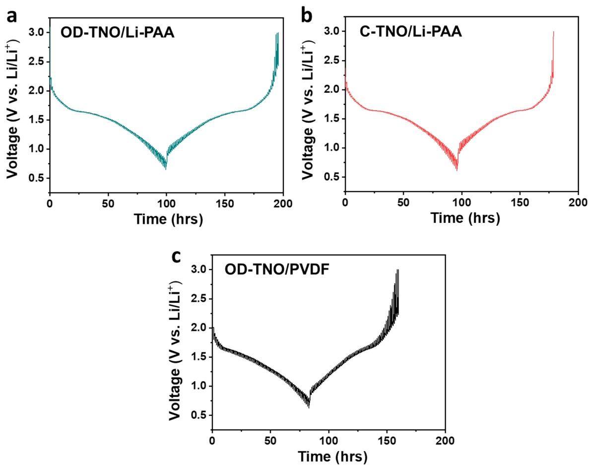
**Figure S13.** The GITT curves for a) OD-TNO/Li<sub>50%</sub>-PAA, b) C-TNO/Li<sub>50%</sub>-PAA, and c) OD-TNO/PVDF.
