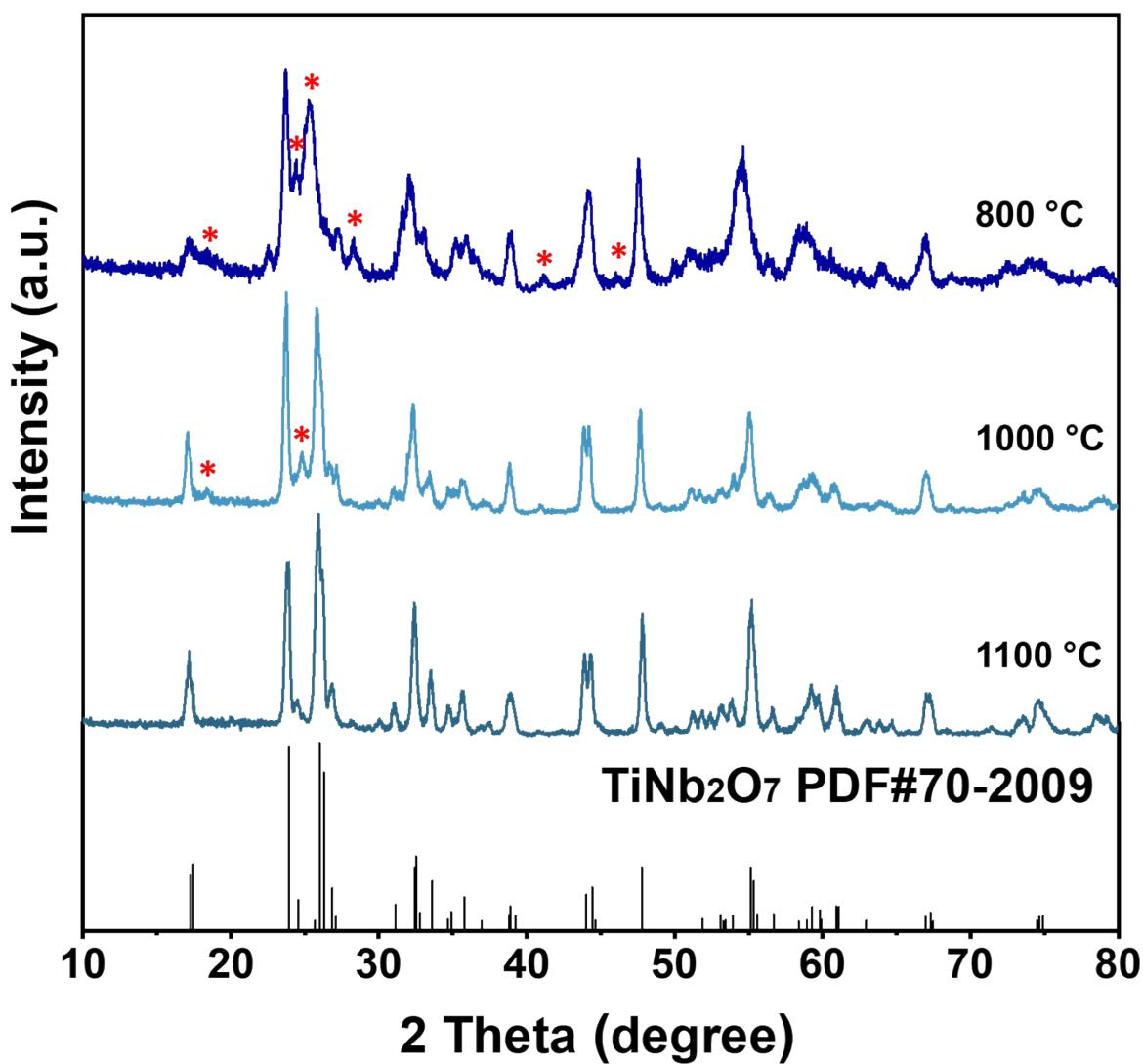
**Figure S3.** XRD patterns of the  $\text{TiNb}_2\text{O}_7$  synthesized from the monoclinic  $\text{Nb}_2\text{O}_5$  precursor at synthesis temperatures of 800, 1000, 1100 °C, with impurities marked with red asterisks.
