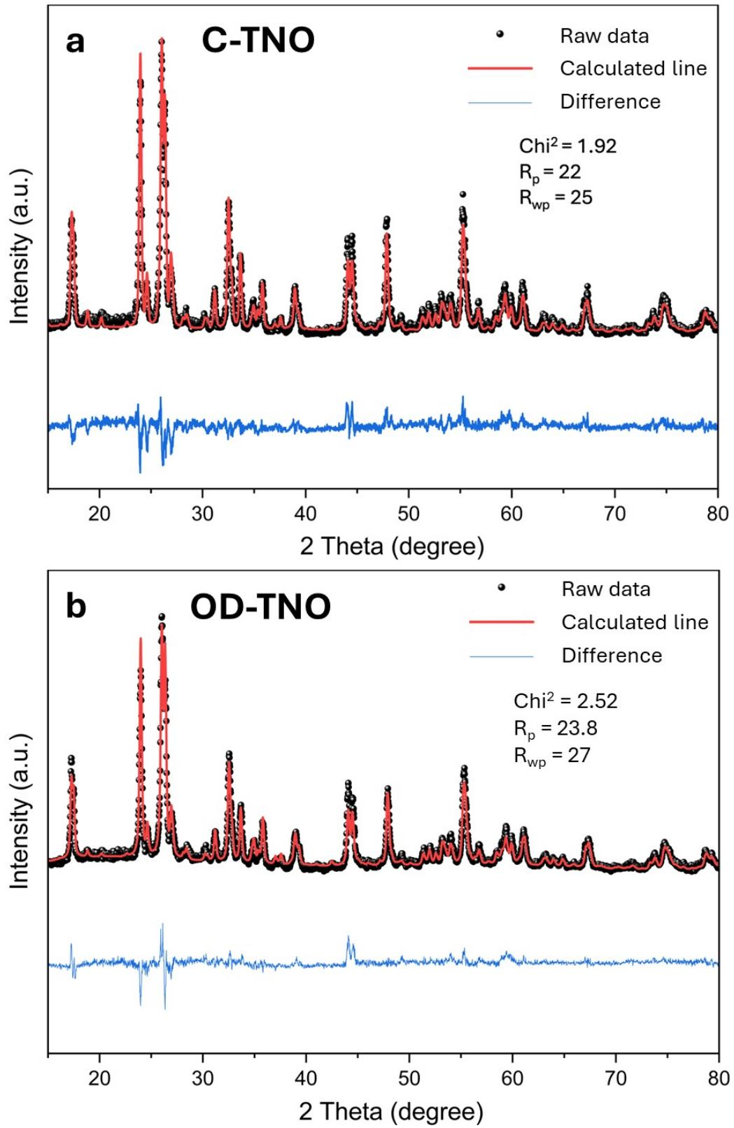
**Figure S5.** Rietveld refinement of the XRD patterns for C-TNO and OD-TNO.
