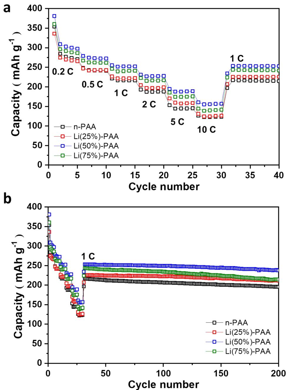
**Figure S8.** The comparison of (a) rate capability and (b) cycling performance for OD-TNO with different PAA-based binders (PAA, Li<sub>25%</sub>-PAA, Li<sub>50%</sub>-PAA, and Li<sub>75%</sub>-PAA).
