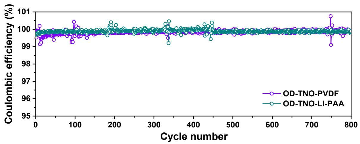
**Figure S10.** Coulombic efficiency of OD-TNO with PVDF and Li-PAA binders. Cells were subjected to 10 formation cycles that are not shown here.
