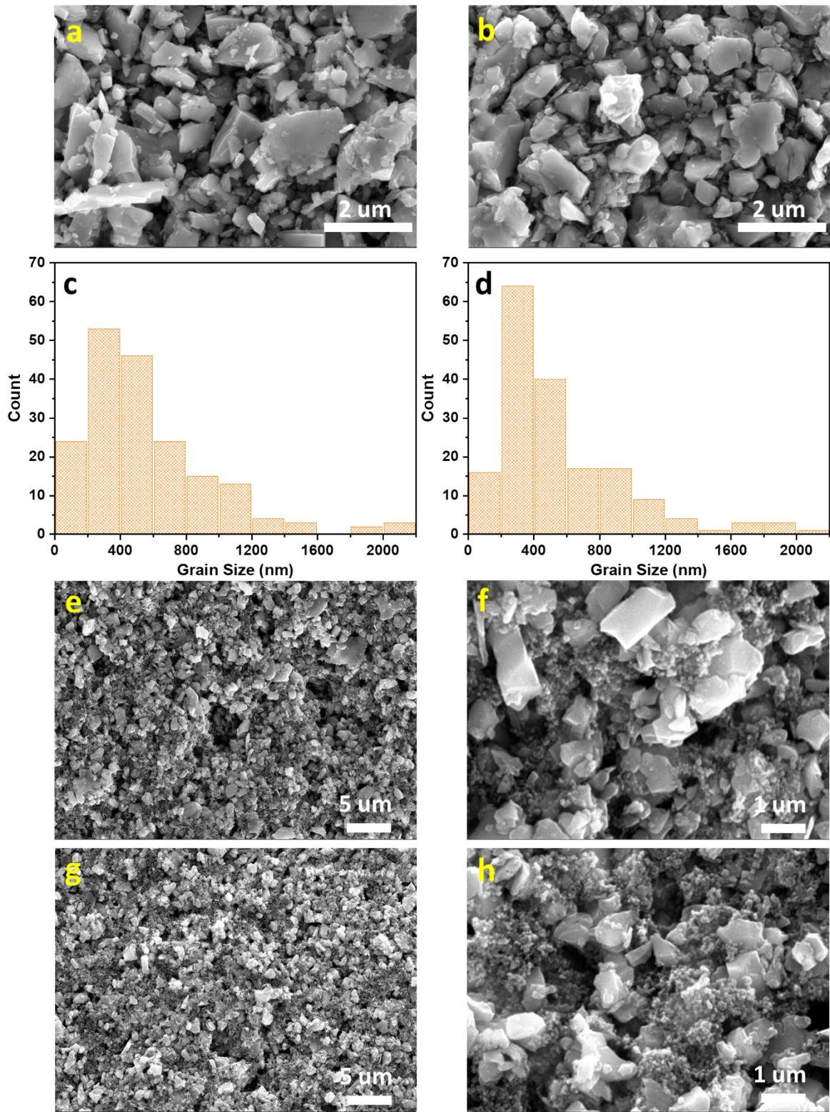
**Figure S7.** SEM images of ball-milled (a) C-TNO and (b) OD-TNO samples, with their size distribution shown in (c) and (d) respectively. SEM images of (e and f) C-TNO@Super P and (g and h) OD-TNO@Super P.
