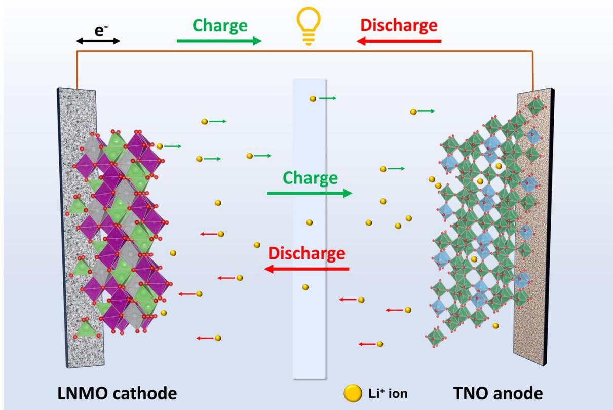
**Figure S16.** Schematic configuration of  $\text{LiNi}_{0.5}\text{Mn}_{1.5}\text{O}_4$ //OD-TNO/Li-PAA full cell battery.
