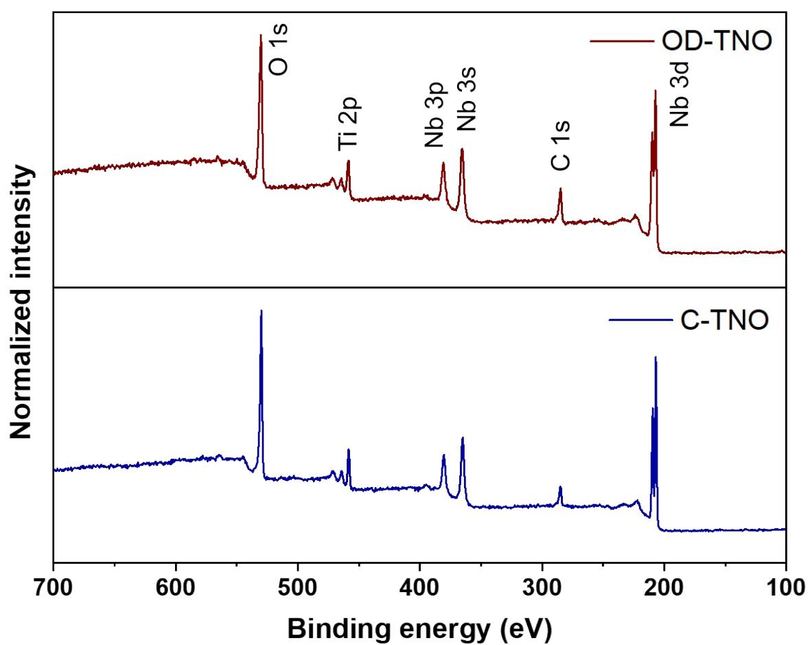
**Figure S6.** XPS survey spectra of C-TNO and OD-TNO.
