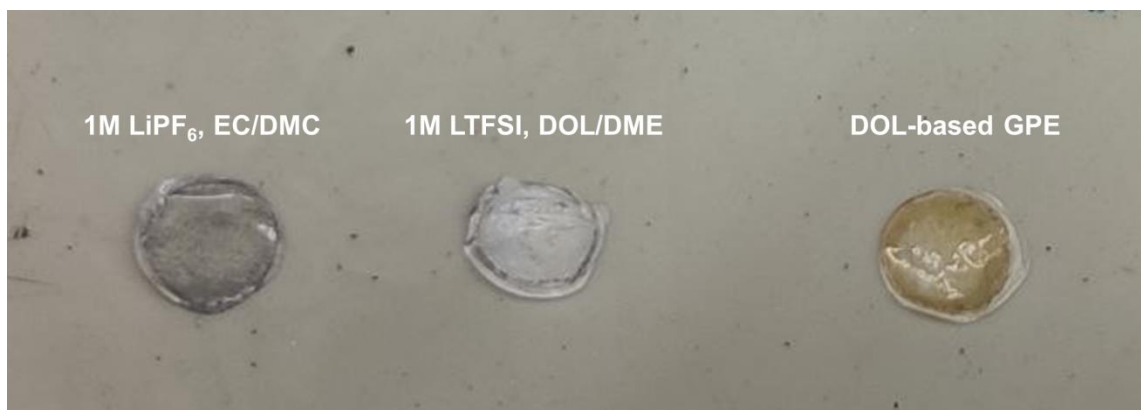
Figure S7. Photographs of the separators extracted from the Li/electrolyte/ PTPQ cells cycled with different electrolytes (for the liquid electrolytes, traces of dissolved PTPQ cathode material are visible (black coloration), and for GPE-based cells, yellowish color is for the polymer electrolyte attached to the separator).
