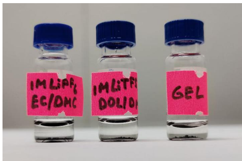
Figure S7. Photographs of the separators extracted from the Li/electrolyte/ PTPQ cells cycled with different electrolytes (for the liquid electrolytes, traces of dissolved PTPQ cathode material are visible (black coloration), and for GPE-based cells, yellowish color is for the polymer electrolyte attached to the separator).
