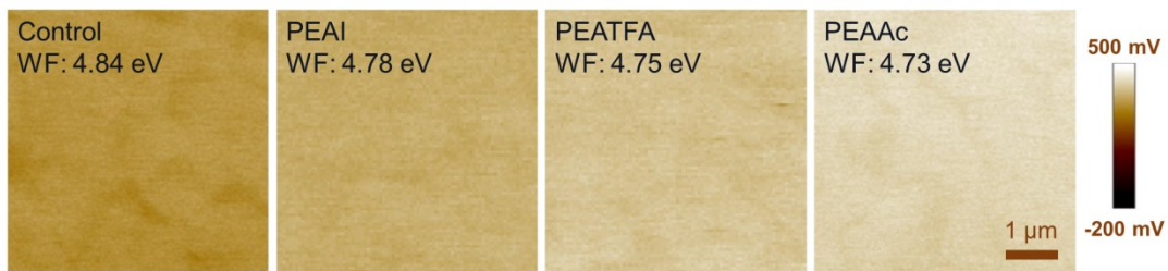
Fig. S34. The surface potential distribution and work function (WF) of control and PEAX-treated perovskite films characterized by KPFM.
