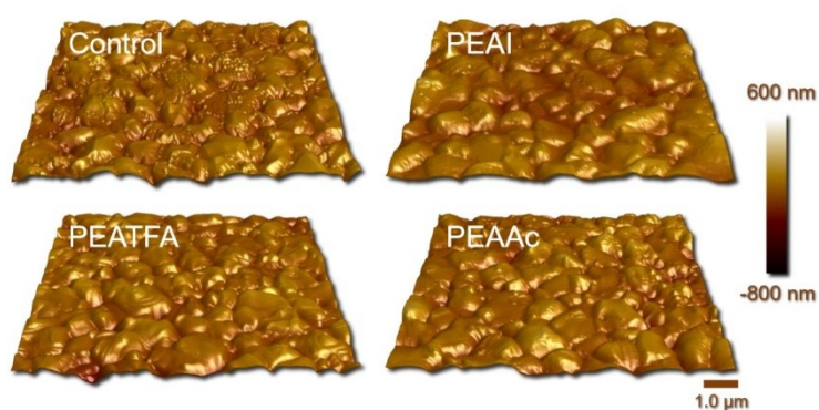
Fig. S28. The morphology of the control and PEAX-modified perovskite films as revealed by atomic force microscopy (AFM). The root mean square (RMS) roughness of the control, PEAI-, PEATFA- and PEAAc-modified perovskite films are 50.1, 51.5, 49.3 and 49.5 nm, respectively.
