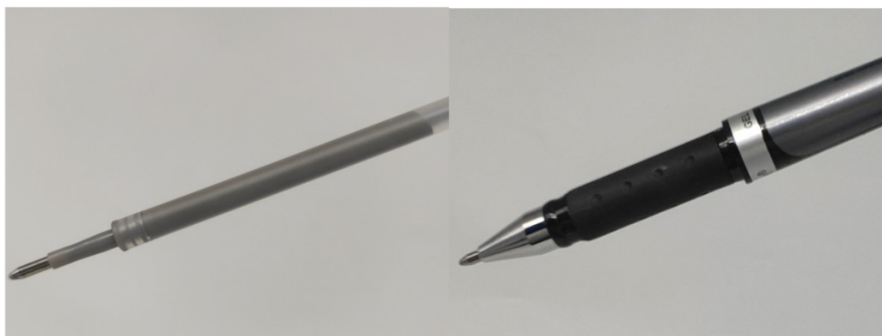
Figure S3. Digital photo of a ballpoint pen filled with OPC/EGaIn NPs inks.
