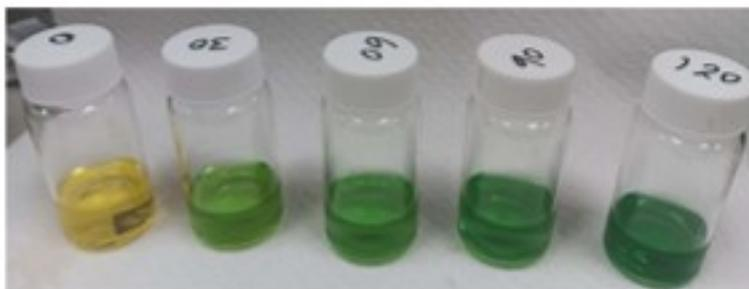
**Fig. S9.** UV-vis absorption spectroscopy for eNRR  $\text{NH}_3$  for the VCuMnBi(2:3:2) catalyst to show the colors every 30 min after being tested by the IPB method.
