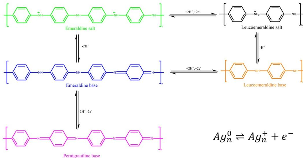
**Fig. S7.** Schematic diagram of redox transformation of polyaniline and Ag
