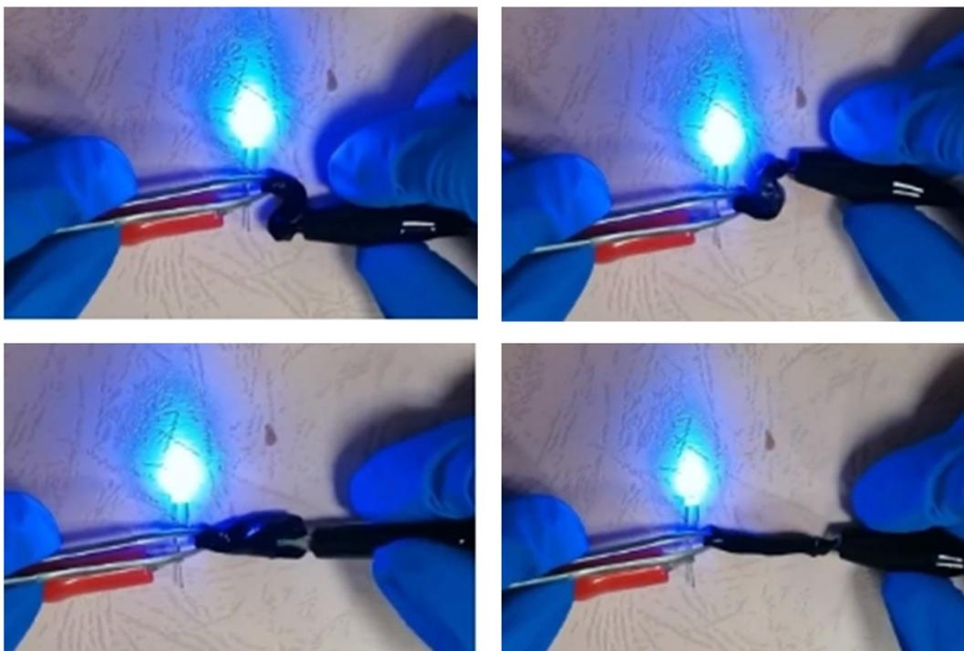
**Fig. S5.** Digital photos of PPA-Ag15 hydrogel as a conductor to light a LED.
