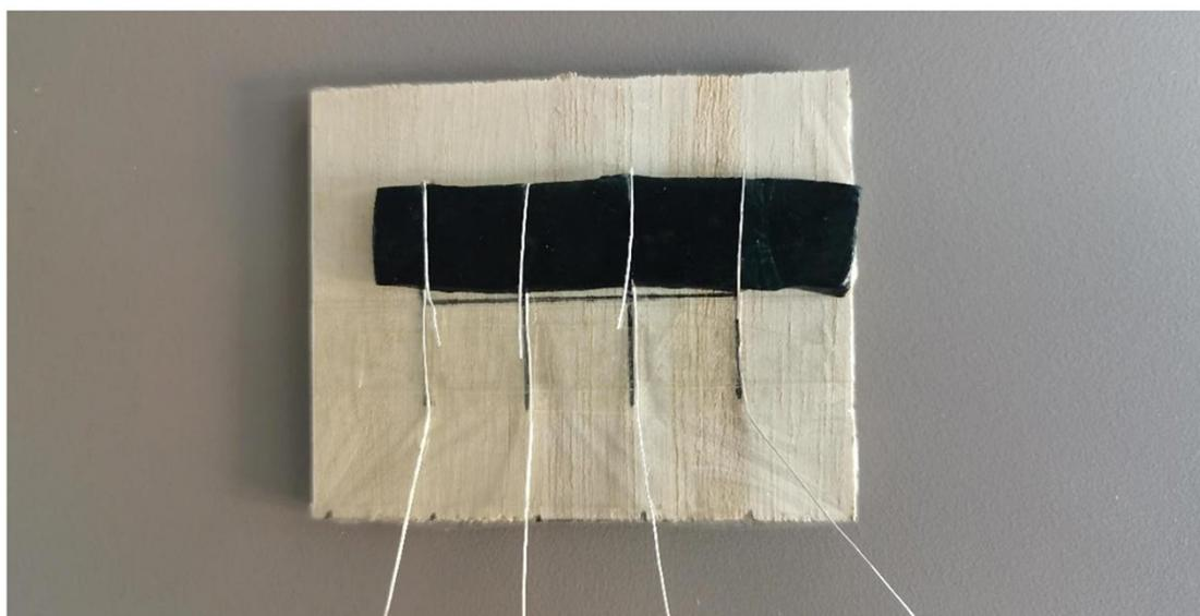
**Fig. S4.** Physical image of a four probe test gel sample
