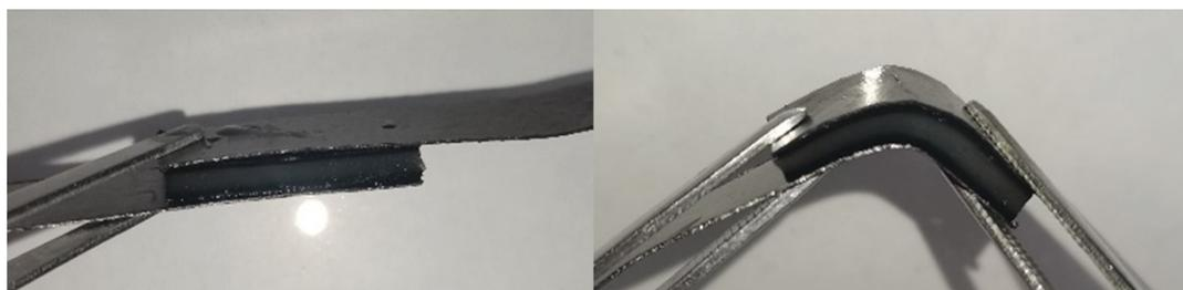
**Fig. S9.** Digital photographs of PPA-Ag hydrogel-based FSCs.
