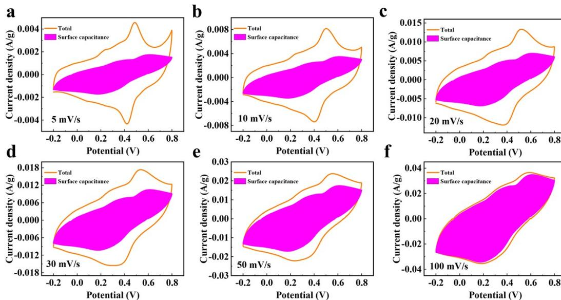
**Fig. S6.** CV curves of PPA-Ag15 hydrogel electrode measured at different scan rates, in which the shadowed area is the surface capacitive contribution.
