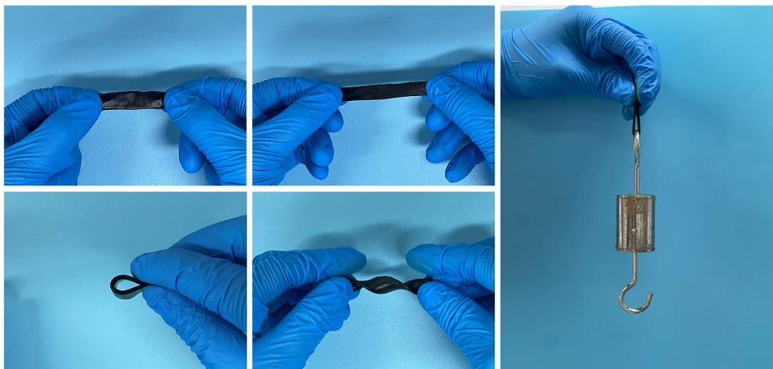
**Fig. S8.** Digital photos of PPA-Ag15 hydrogel under bending, twisting and holding a weight of 200 g.
