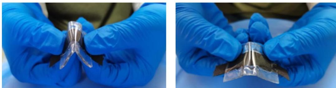
**Fig. S10.** Digital photographs of bent PPA-Ag hydrogel-based FSCs.
