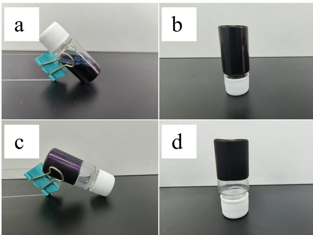
**Fig. S1.** Digital photos of PPA-Ag hydrogel (a) (b) before and (c) (d) after gelation.
