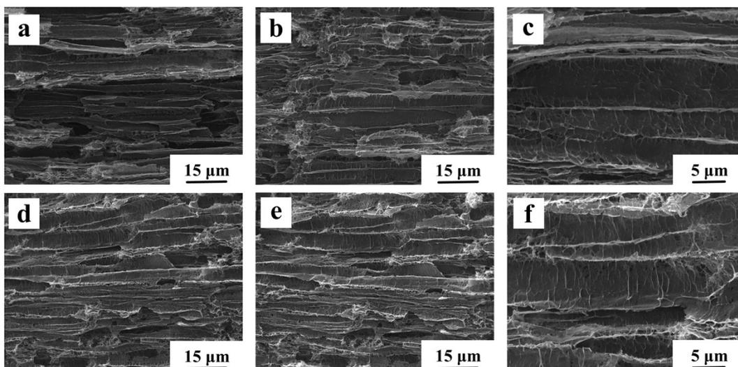
**Fig. S3.** SEM images from another cross-section that was perpendicular to the 3D porous-like cross-section: (a-c) PPA hydrogel; (d-f) PPA-Ag15 hydrogels.
