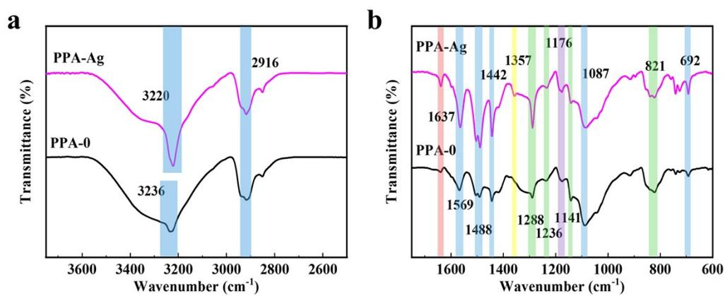
**Fig. S2.** FTIR spectra of PPA-0 and PPA-Ag composite hydrogels
