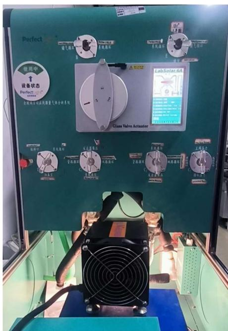
**Figure S17.** Photograph of the photocatalytic online analytical system (LabsolarI-6A, Beijing Perfectlight Technology Co., Ltd).
