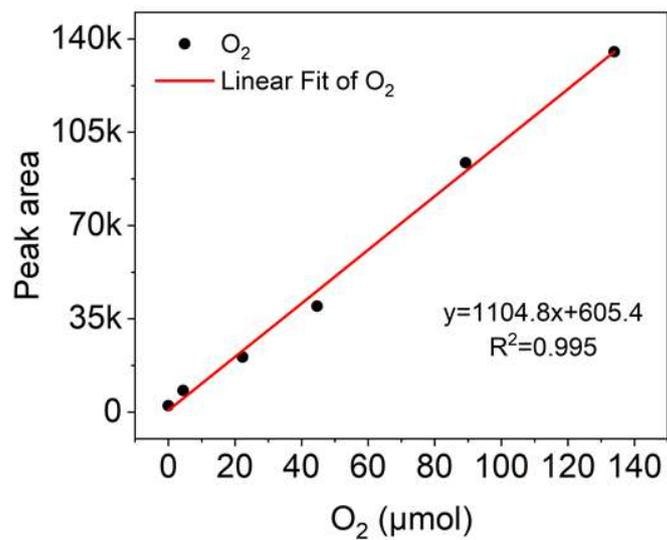
**Figure S18.** The calibrated standard curve of O<sub>2</sub> in gas chromatograph with TCD.
