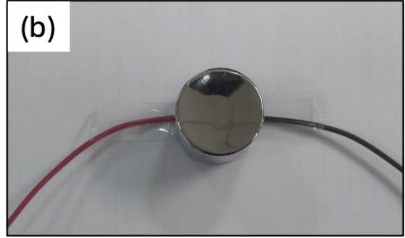
Figure S10. Nanocomposite sensor sealed with Scotch tape.
