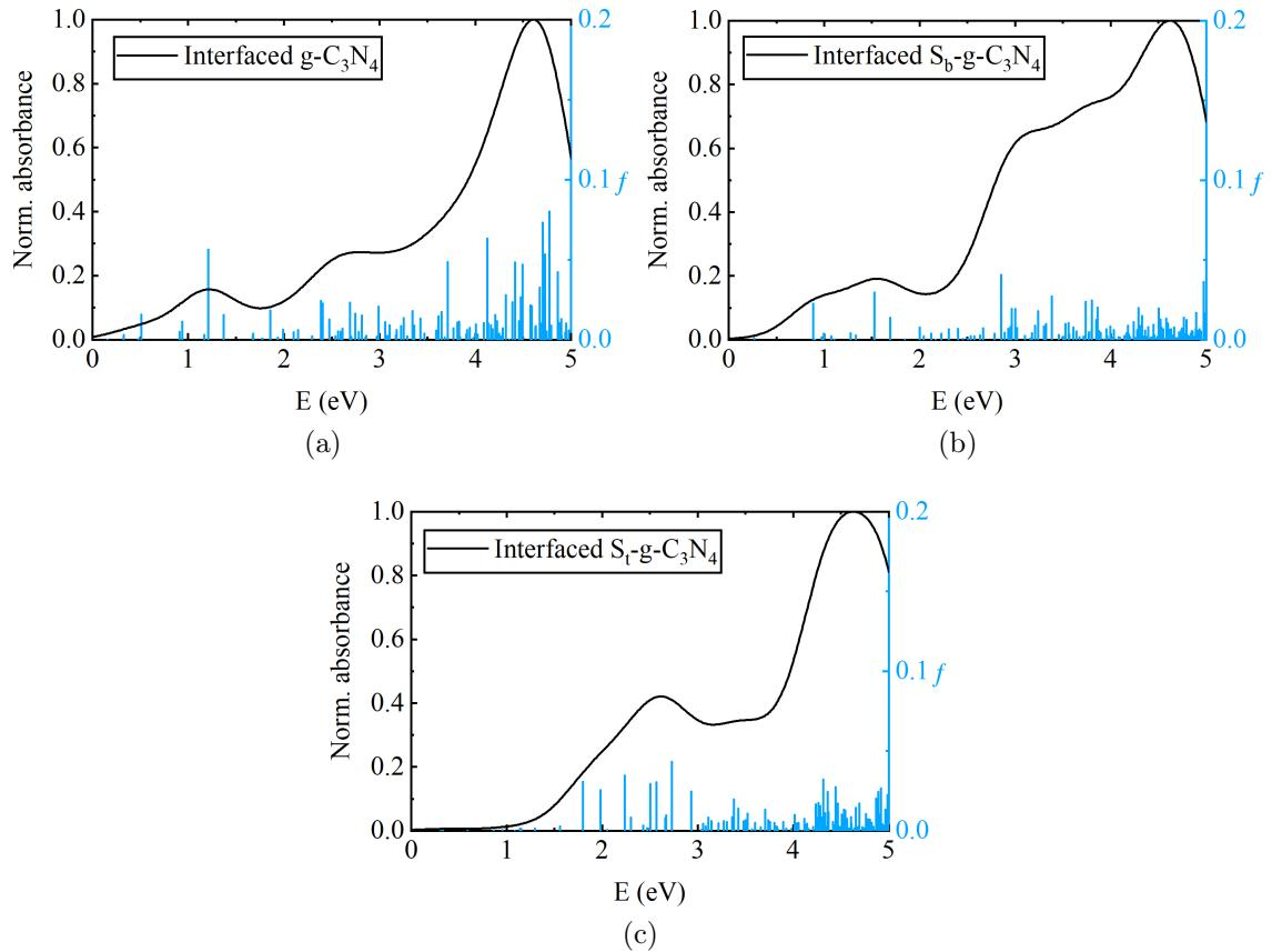
Figure S5: Simulated UV-Vis. spectra of interfaced (a)  $g\text{-C}_3\text{N}_4$ , (b)  $S_b\text{-}g\text{-C}_3\text{N}_4$  and (c)  $S_t\text{-}g\text{-C}_3\text{N}_4$  along with the computed stick spectrum (in blue) with heights corresponding to the computed oscillator strengths of the electronic transitions.
