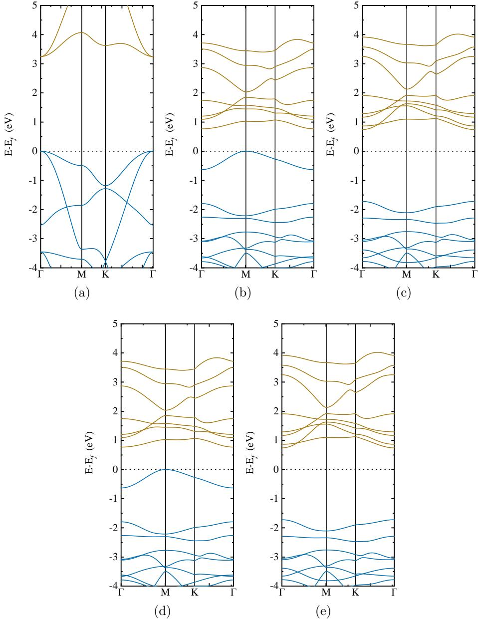
Figure S3: Band structures of freestanding (a)  $g\text{-C}_3\text{N}_4$ , (b)  $\alpha \text{S}_b\text{-}g\text{-C}_3\text{N}_4$ , (c)  $\beta \text{S}_b\text{-}g\text{-C}_3\text{N}_4$ , (d)  $\alpha \text{S}_t\text{-}g\text{-C}_3\text{N}_4$ , and (e)  $\beta \text{S}_t\text{-}g\text{-C}_3\text{N}_4$ . All data obtained at the HSE06-D2 level.
