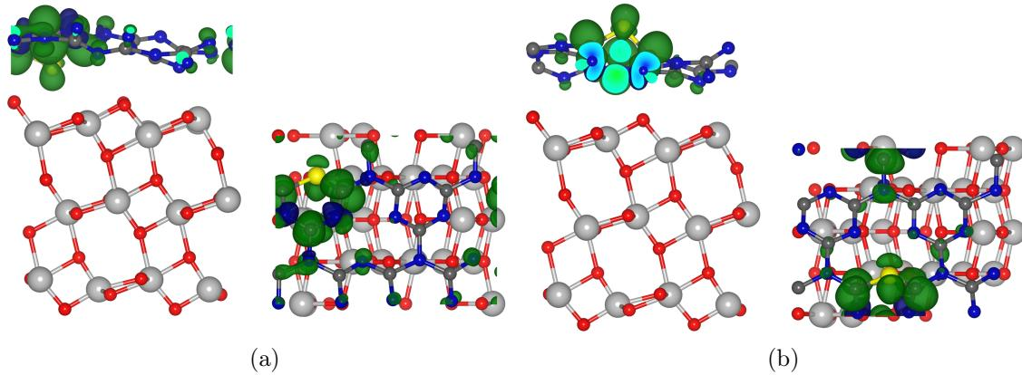
Figure S2: Spin densities of the (a)  $S_b$ -g- $C_3N_4/TiO_2$  and (b)  $S_t$ -g- $C_3N_4/TiO_2$  composite models in a doublet spin state. C, N, S, Ti and O shown as brown, blue, yellow, grey and red spheres, respectively. Isosurface values of  $|0.0025| \text{ e.bohr}^{-3}$ .
