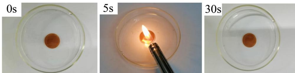
Fig. S2 thermal stability test of  $\text{Na}_2\text{ZrCl}_6$ -PAN composite solid electrolyte
