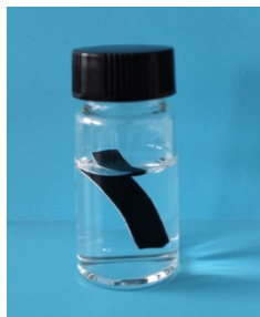
Fig. S22 Photograph illustrating the FRHH electrode was soaked and stirred in water for different durations, after which the liquid was extracted for subsequent ICP test.
