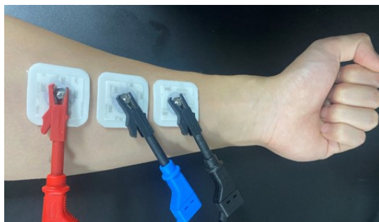
Fig. S25 Photographs of the three-electrode system AC impedance test conducted on human skin, where the red electrode serves as the working electrode, the blue electrode acts as the reference electrode, and the black electrode functions as the counter electrode.
