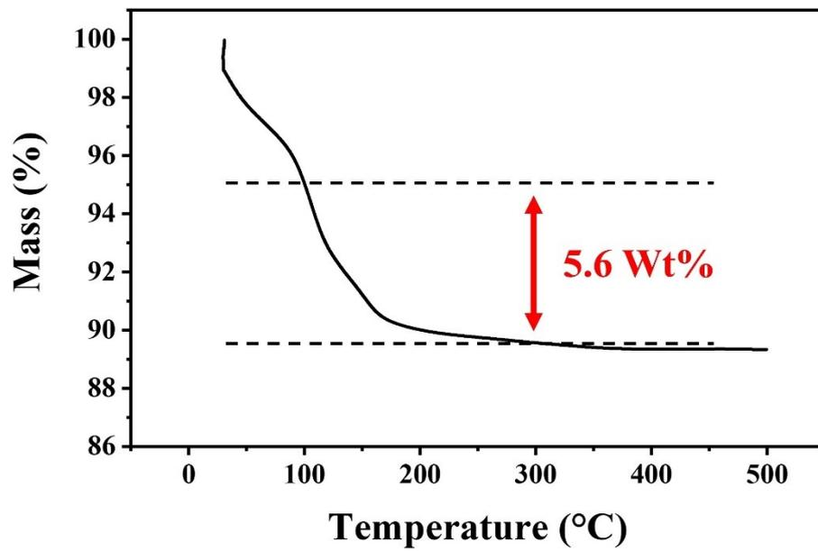
Figure. S1 TGA curve of NaVO
