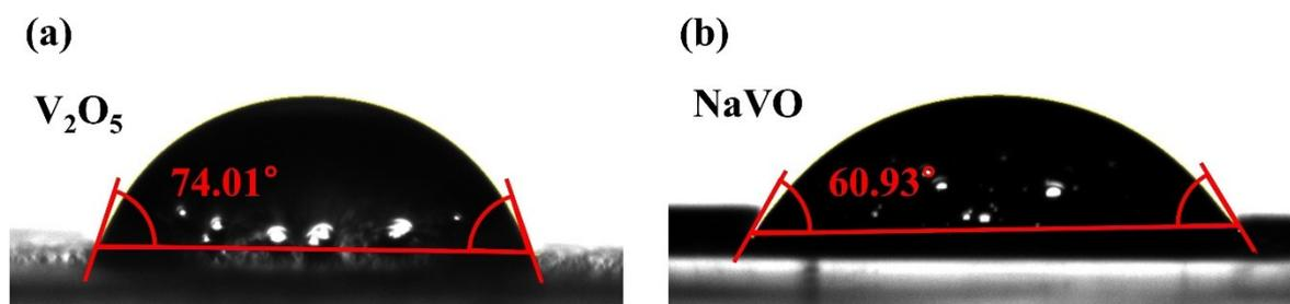
**Figure. S6** The contact angles of electrolyte on (a) V<sub>2</sub>O<sub>5</sub> and (b) NaVO cathode.
