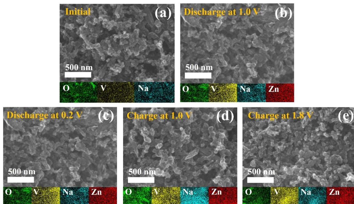
**Figure. S10** SEM images and EDS mapping of NaVO (a) Initial (b) Discharge at 1.0 V (c) Discharge at 0.2 V (d) Charge at 1.0 V and (e) Charge at 0.2 V.
