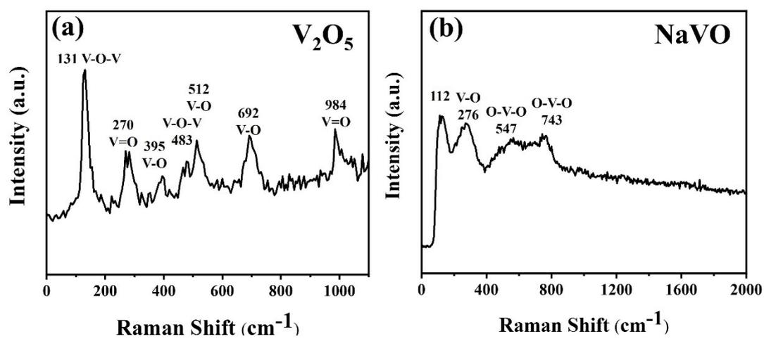
Fig. S3. Raman spectra of (a)  $V_2O_5$  and (b) NaVO
