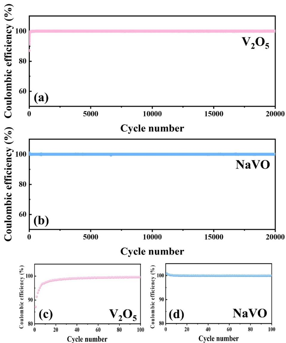
**Figure. S8** Coulombic efficiency of (a) NaVO and (b)  $V_2O_5$  for 10000 cycles. Coulombic efficiency of (c) NaVO and (d)  $V_2O_5$  for 100 cycles.
