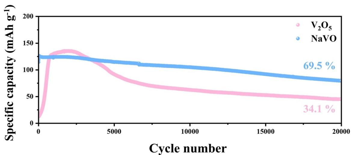
**Figure. S7** Cycling performance of NaVO//Zn and V<sub>2</sub>O<sub>5</sub>//Zn at 10A g<sup>-1</sup>.
