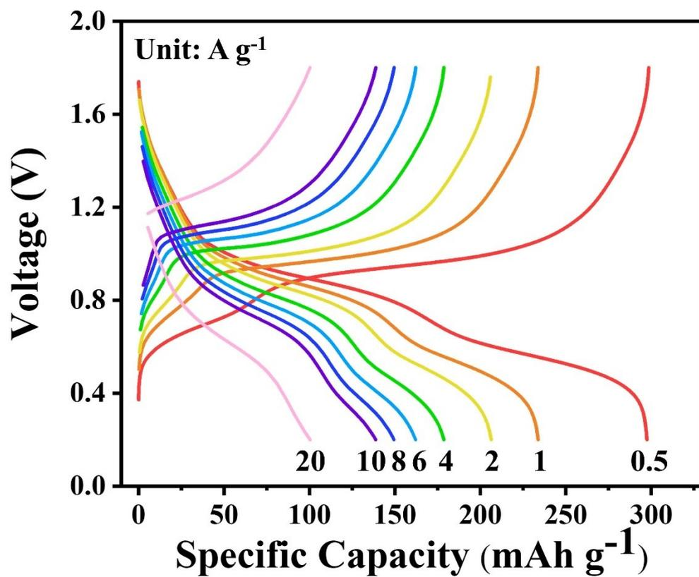
**Figure. S5** Charge/Discharge curve of NaVO//Zn at 0.5, 1, 2, 4, 6, 8, 10 and 20 A g<sup>-1</sup> respectively.
