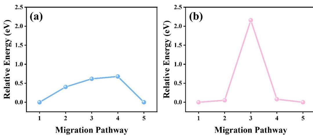
**Figure. S12** Relative energy for Zn ion migration between equivalent sites in (a) NaVO and (b) V<sub>2</sub>O<sub>5</sub> cathodes along the pathway.
