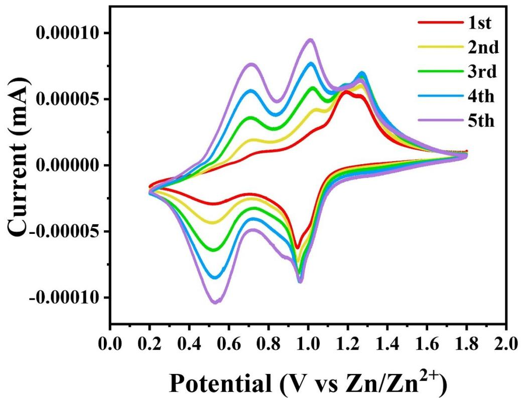
**Figure. S9** CV curves of  $V_2O_5//Zn$  for 5 cycles at scan rates from  $0.1 \text{ mV s}^{-1}$ .
