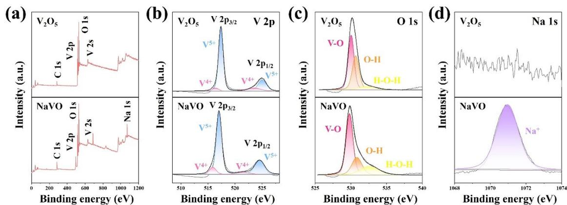
**Figure. S4** Characteristics of the  $V_2O_5$  and NaVO from XPS spectra. (a) The wide survey scan of  $V_2O_5$  and NaVO. A narrow scan data and fitted curves of V 2p, O 1s, and Na 1s are shown in (b), (c), and (d), respectively.
