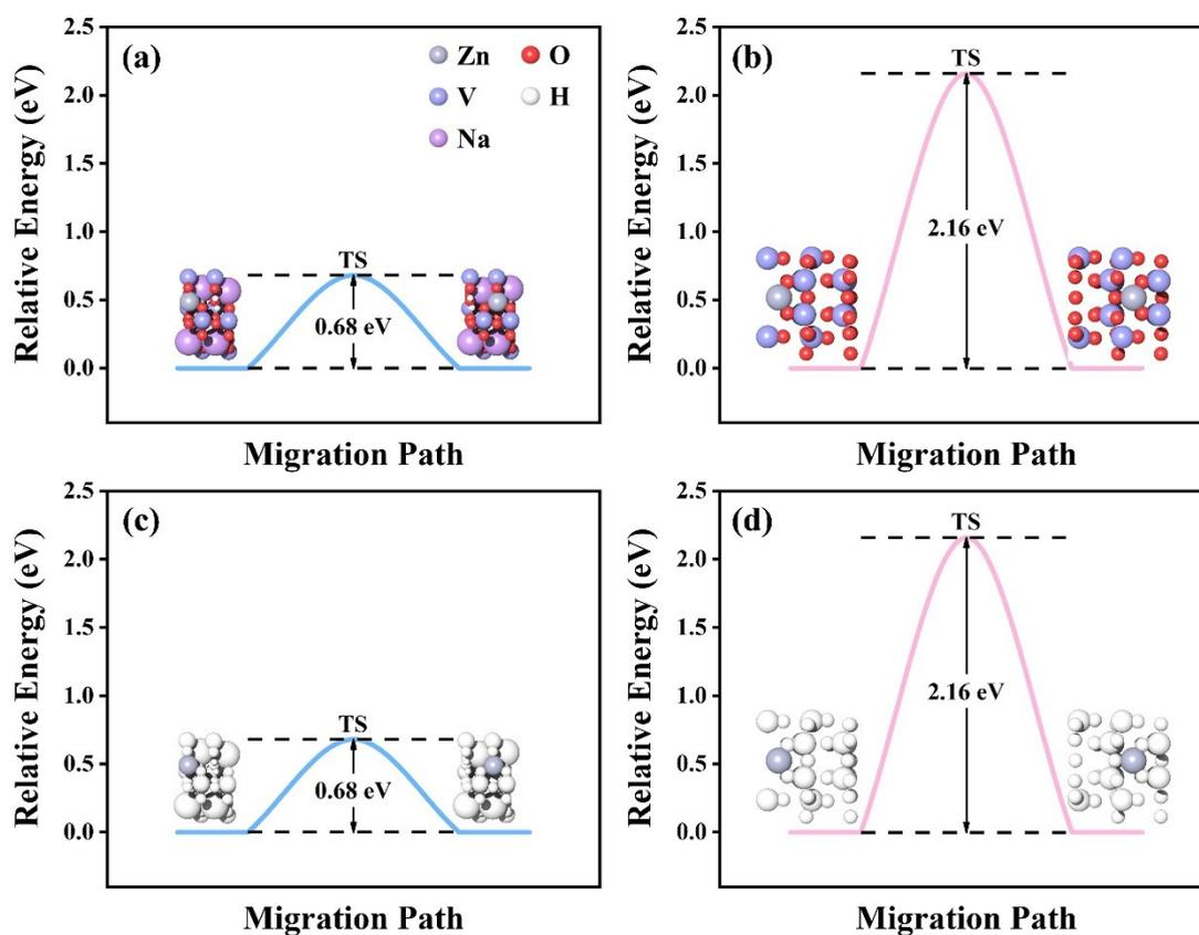
**Figure. S13** Relative energy plot of initial, transition and final state during Zn migration between equivalent sites in (a), (c) NaVO and (b), (d) V<sub>2</sub>O<sub>5</sub> cathodes. (Zn: gray, V: blue, Na: violet, O: red, H: white)
