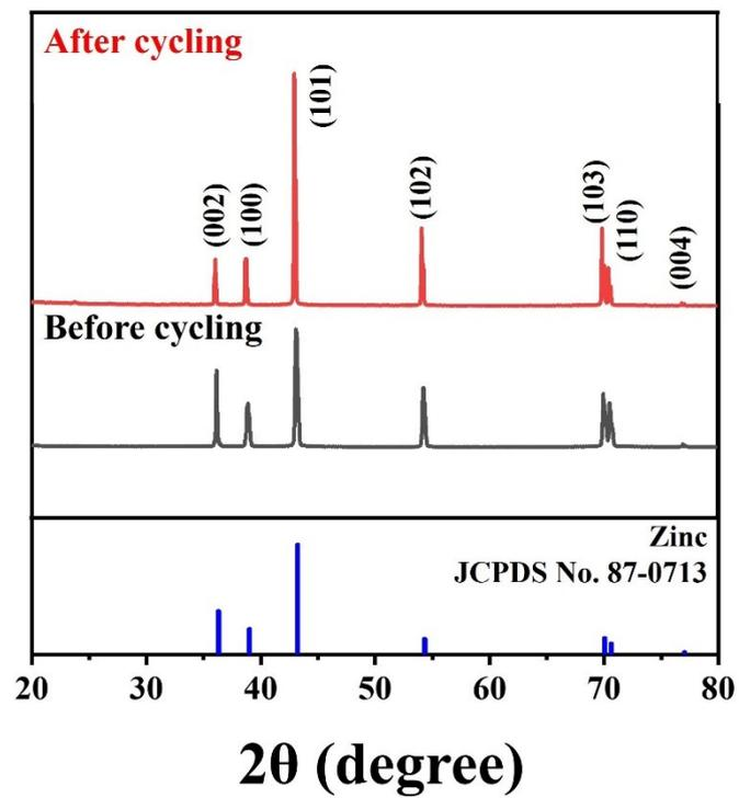
**Figure. S16** The XRD patterns of Zinc Anode before and after cycling.
