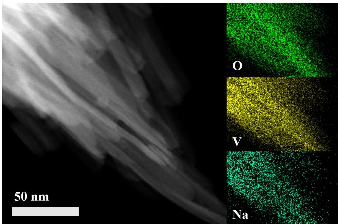
Figure. S2 TEM image and EDX mapping of NaVO
