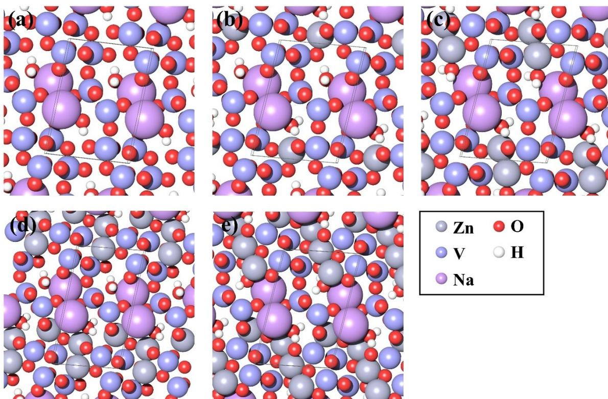
**Figure. S11** Optimized structural configurations of NaVO with Zn intercalation at concentrations of (a) 0, (b) 1, (c) 2, (d) 3, and (e) 4 Zn ions. (Zn: gray, V: blue, Na: violet, O: red, H: white)
