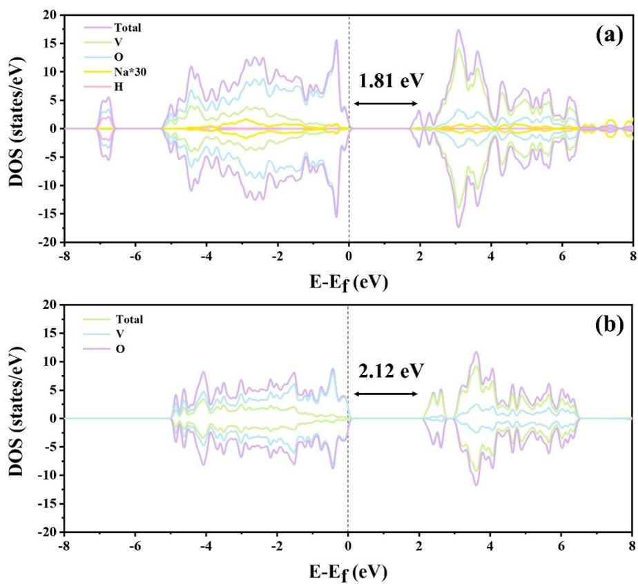
**Figure. S15** Electronic density of states for (a) NaVO and (b) V<sub>2</sub>O<sub>5</sub>
