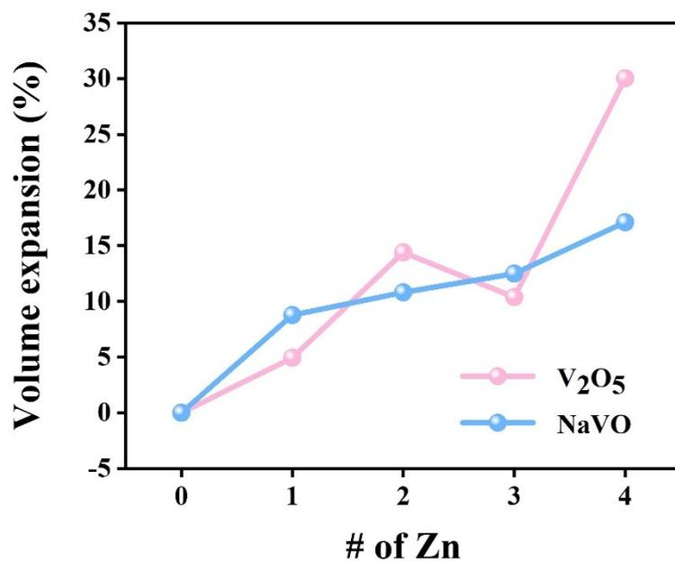
**Figure. S14** Comparison of volume expansion ratio in NaVO and  $V_2O_5$  cathodes during Zn intercalation.
