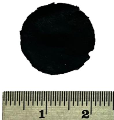
**Fig. S14.** Photograph of a large-scale MXA composite membrane in centimeter scale.
