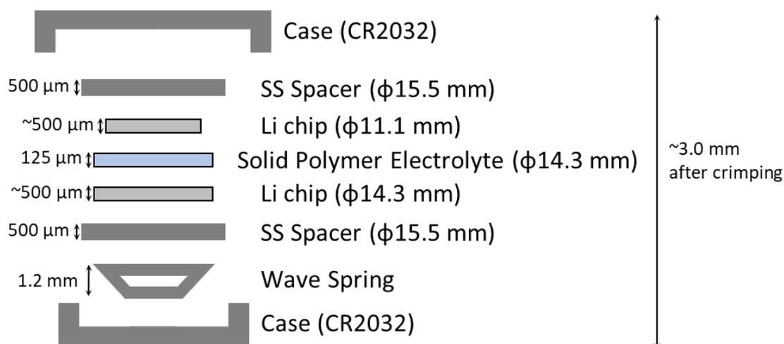
**Figure S2.** Coin cell stack used for electrochemical impedance spectroscopy and Li symmetric cycling experiments.
