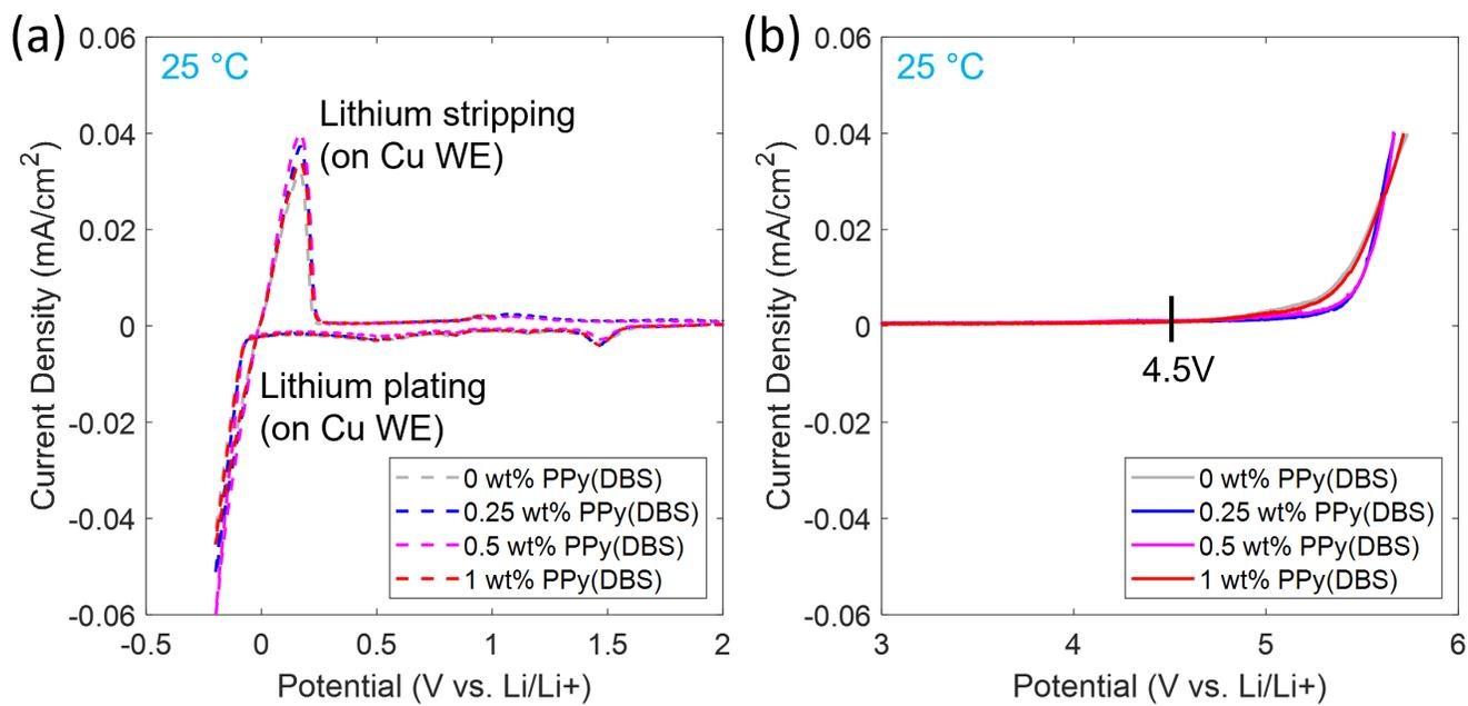
**Figure S10.** Zoomed-in plots of (a) the cathodic CVs and (b) the anodic LSV for determining ESW of the polymer electrolyte compositions with 0-1 wt% PPy(DBS).
