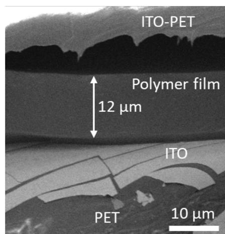
**Figure S1.** SEM cross-section of thin polymer film (targeting ~10 μm thick) between indium tin oxide (ITO) coated polyethylene terephthalate (PET) sheets. Cross-section obtained by shearing with titanium coated blade. SEM micrograph obtained with backscatter electron mode at an accelerating voltage of 2 kV and beam current of 13 pA.
