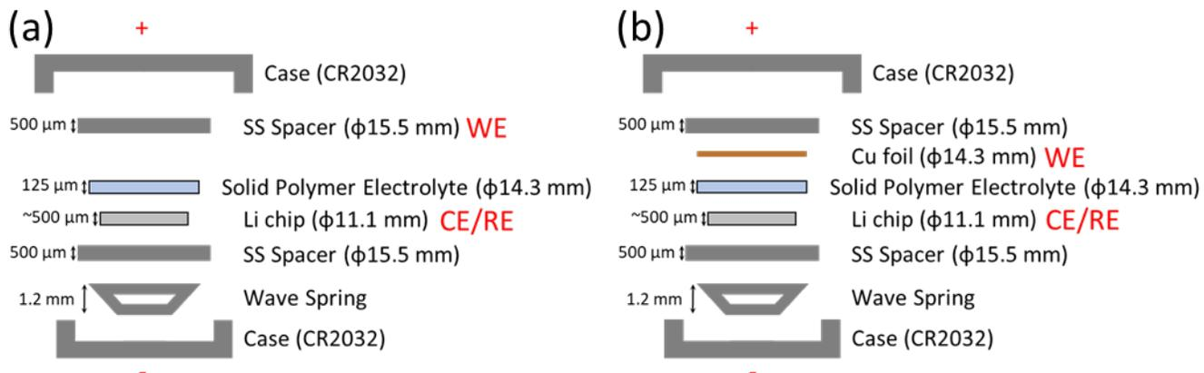
**Figure S3.** Coin cell stack used for electrochemical stability window experiments with Li-metal as the counter/reference electrode (CE/RE) for (a) anodic scan with 304SS as the working electrode (WE) and (b) cathodic scan with Cu as the WE.
