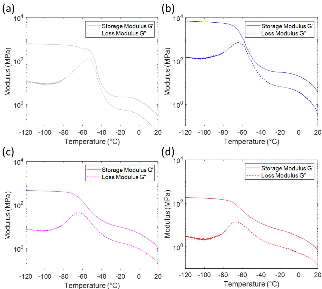
**Figure S6.** DMA storage ( $G'$ ) and loss modulus ( $G''$ ) profiles for (a) 0 wt% PPy(DBS), (b) 0.25 wt% PPy(DBS), (c) 0.5 wt% PPy(DBS), and (d) 1 wt% PPy(DBS).
