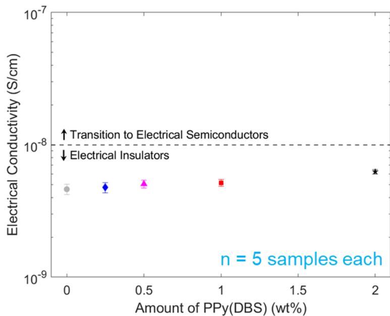
**Figure S5.** Electrical conductivity measurements of the polymer films with varying amounts of PPy(DBS). Markers indicate average values and error bars indicate standard deviations.
