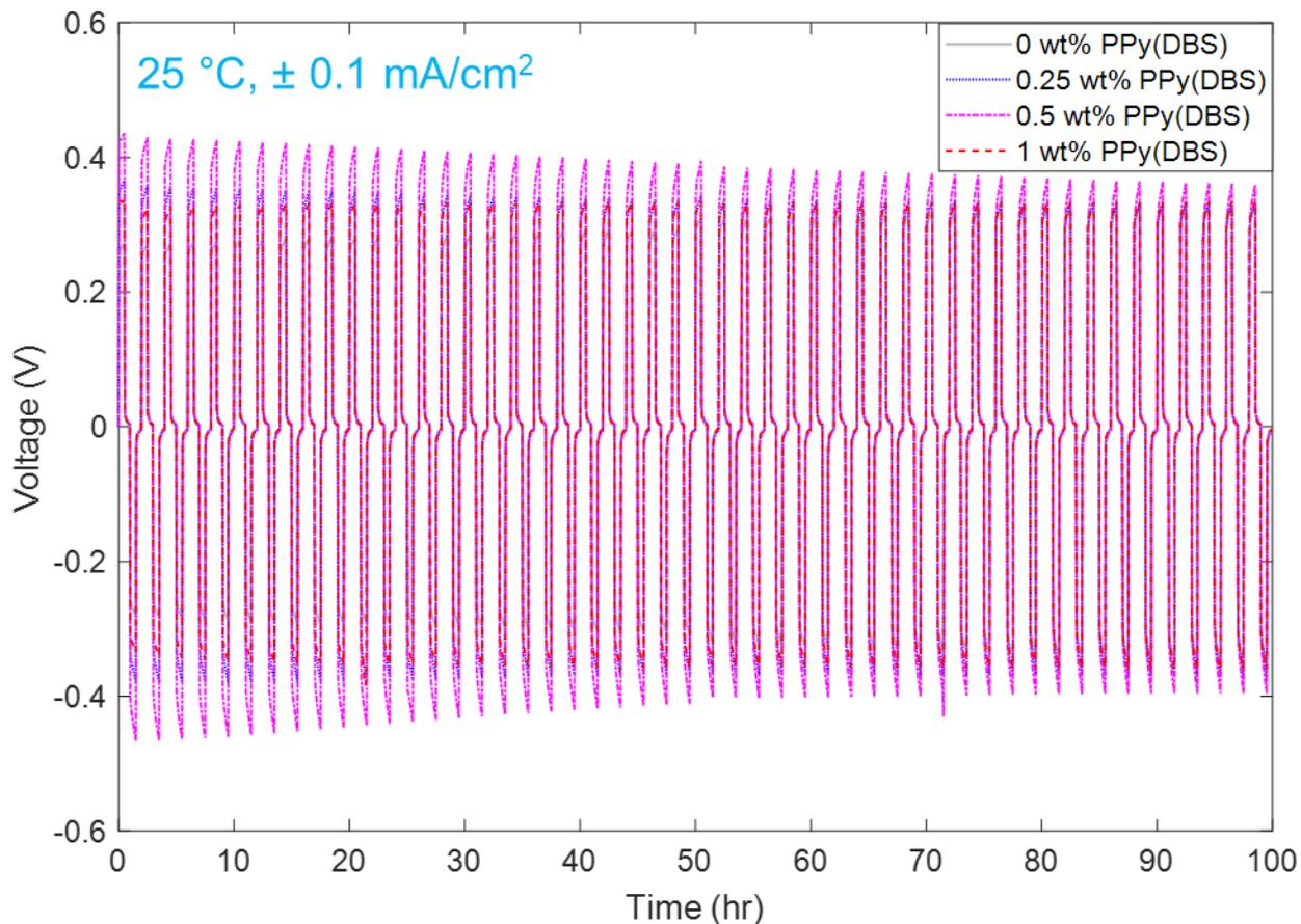
**Figure S8.** Li symmetric cycling overpotentials for a representative Li/polymer/Li coin cell from each composition at 25 °C under  $\pm 0.1 \text{ mA/cm}^2$  for 30 min each direction with 30 min rests for 50 cycles.
