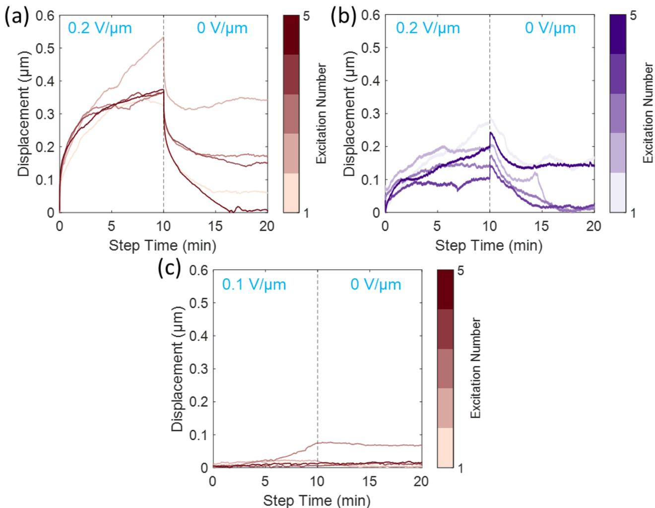
**Figure S7.** AFM continuous point measurement of polymer film under 0.1-0.2  $\text{V}/\mu\text{m}$  followed by 0  $\text{V}/\mu\text{m}$  electric field strength for (a) 1 wt% PPy(DBS) with 0.2  $\text{V}/\mu\text{m}$  excitations, (b) 0.5 wt% PPy(DBS) with 0.2  $\text{V}/\mu\text{m}$  excitations, and (c) 1 wt% PPy(DBS) with 0.1  $\text{V}/\mu\text{m}$  excitations.
