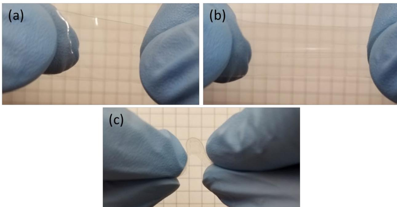
**Figure S4.** Demonstrating the as produced free-standing polymer electrolyte film for 0 wt% PPy(DBS) composition. (a) Unstretched film, (b) stretching the film and (c) bending the film. Grid size 5 mm.
