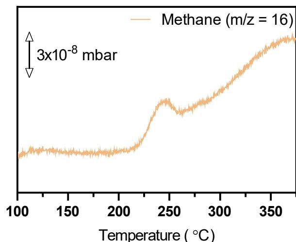
**Figure S7.** MS analysis of methane ( $m/z = 16$ ) obtained by reduction of  $\text{RuO}_2/\text{SiO}_2$  with ethanol.
