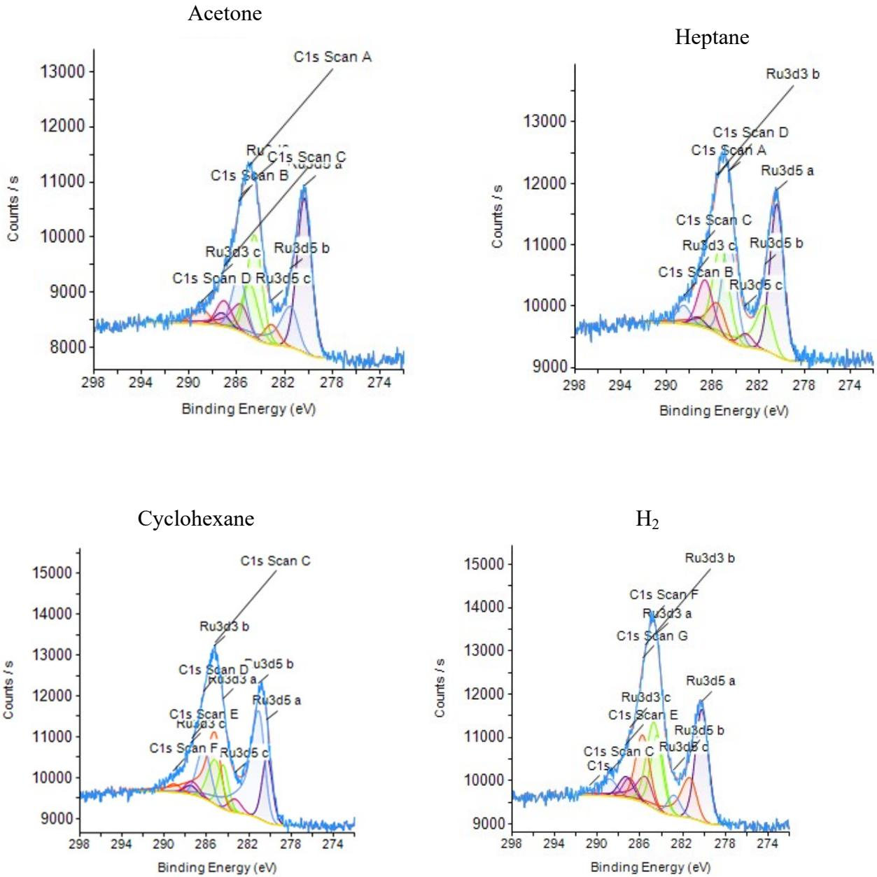
**Figure S12.** The C1s and Ru3d XPS spectra of  $\text{RuO}_2/\text{SiO}_2$  and after reduction with different reducing agents.
