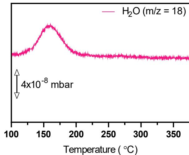
**Figure S3.** MS analysis of  $\text{H}_2\text{O}$  ( $m/z = 18$ ) obtained by reduction of  $\text{RuO}_2/\text{SiO}_2$  with 5% $\text{H}_2/\text{N}_2$ .
