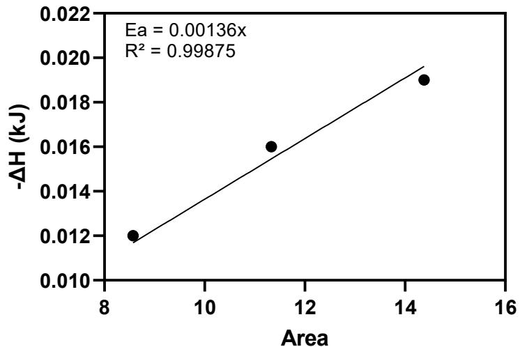
**Figure S2.** Calibration of  $\Delta H$  using  $Pt/\gamma-Al_2O_3$  with 3, 4 and 5% weight Pt. Area based on integration over time (signal x time).
