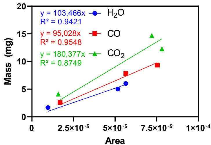
**Figure S1.** Calibration of mass using the decomposition of  $(COO)_2Ca \cdot H_2O$ . Area based on integration over time (signal x time).
