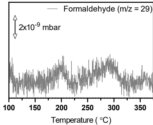
**Figure S8.** MS analysis of formaldehyde ( $m/z = 29$ ) obtained by reduction of  $\text{RuO}_2/\text{SiO}_2$  with methanol.
