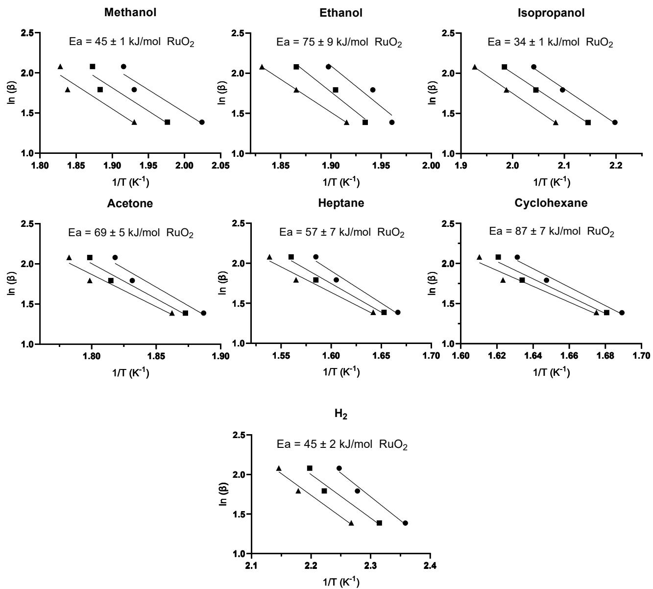
**Figure S5.** Flynn-Wall-Ozawa plots for activation energy ( $E_{app}$ ) of reduction of  $\text{RuO}_2/\text{SiO}_2$  using seven different reducing agents and calculated activation energy.
