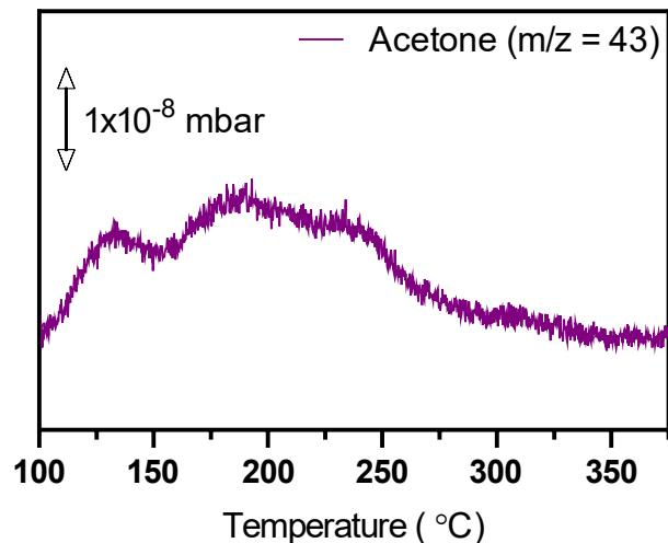
**Figure S6.** MS analysis of acetone ( $m/z = 43$ ) obtained by reduction of  $\text{RuO}_2/\text{SiO}_2$  with isopropanol.
