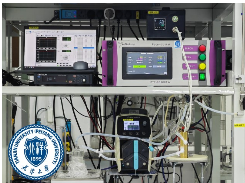
Fig. S32 The single AEMWE cell test system.
