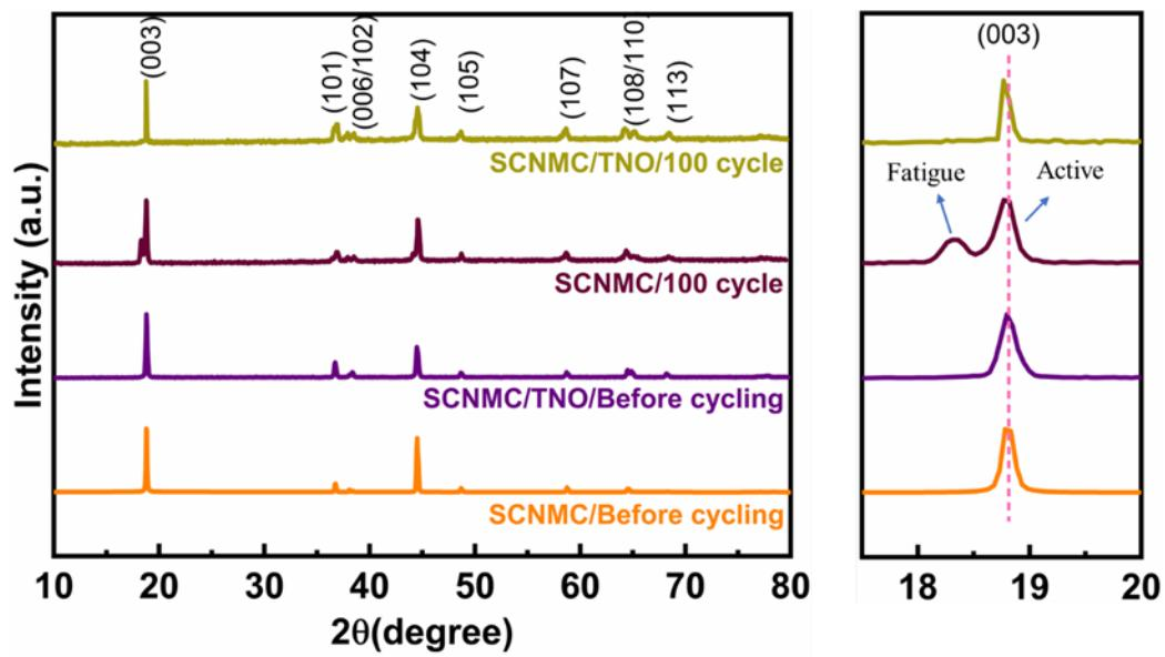
Figure S11. XRD of SCNMC and SCNMC/TNO after 100 cycles and zoom view of (003) indexed peak.
