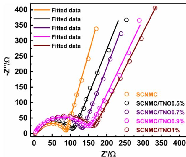
Figure S9. EIS profile of various mole % of TNO coated SCNMC
