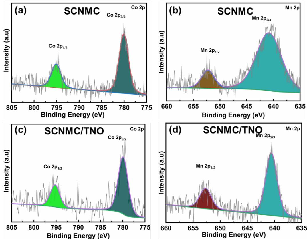
Figure S8. (a) and (c) shows Co 2p spectra with fitted components for SCNMC and SCNMC/TNO, (b) and (d) shows Mn 2p spectra with fitted components for SCNMC and SCNMC/TNO samples.
