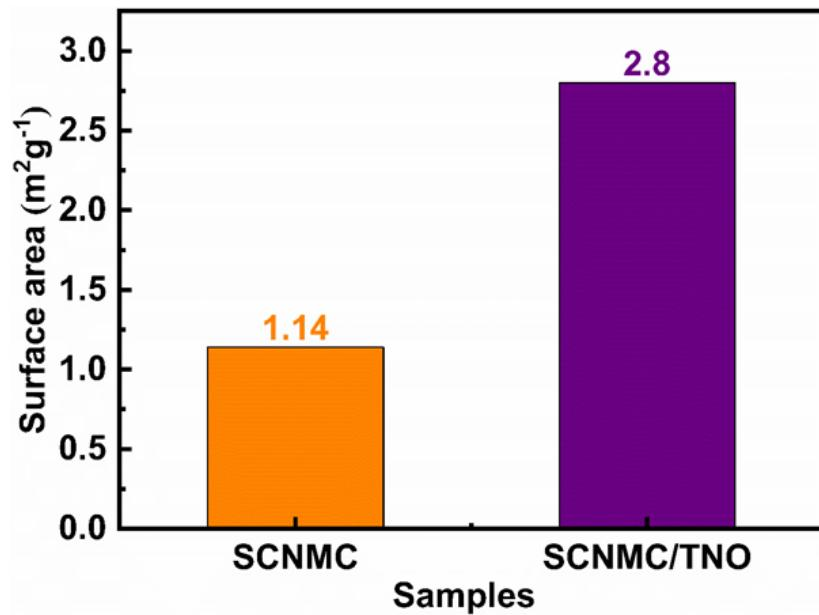
Figure S6. Specific surface area value for SCNMC and SCNMC/TNO.
