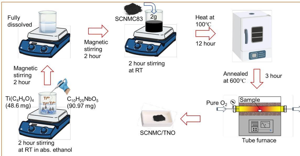
Figure S1. Experimental procedure to prepare SCNMC/TNO powder.
