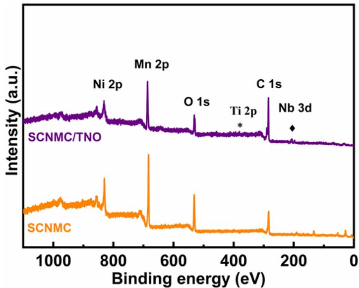
Figure S7. XPS survey spectra of SCNMC and SCNMC/TNO
