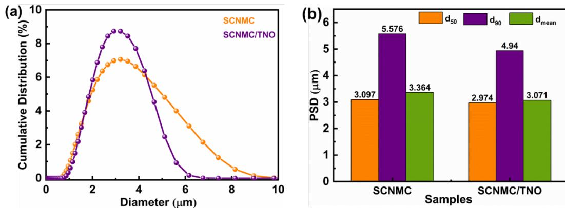
Figure S2. (a) Particle size distribution for SCNMC and SCNMC/TNO by Dynamic Light Scattering (DLS), (b)  $d_{50}$ ,  $d_{90}$ , and  $d_{\text{mean}}$  values ( $\mu\text{m}$ ).
