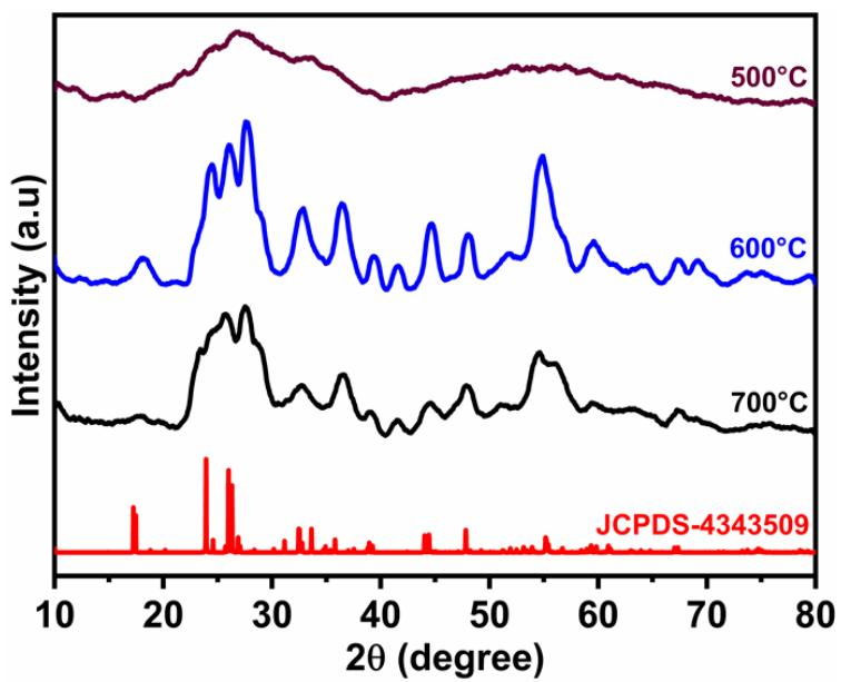
Figure S4. XRD patterns of synthesized pure  $\text{TiNb}_2\text{O}_7$  at 500 °C, 600 °C, and 700 °C.
