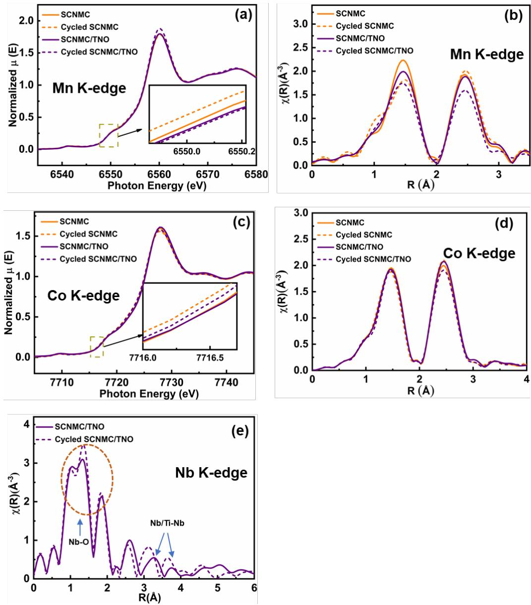
Figure S12. XANES spectra of SCNMC and SCNMC/TNO before and after 100 cycles for (a) Mn, and (c) Co; FT-EXAFS spectra for (b) Mn, (d) Co, and (e) Nb- K edge.
