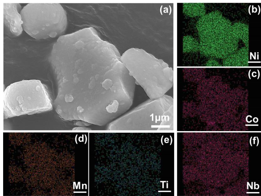
Figure S5. (a) Single particle of SCNMC/TNO, SEM-EDS mapping of (a) Ni, (c) Co, (d) Mn, (e) Ti, and (f) Nb.
