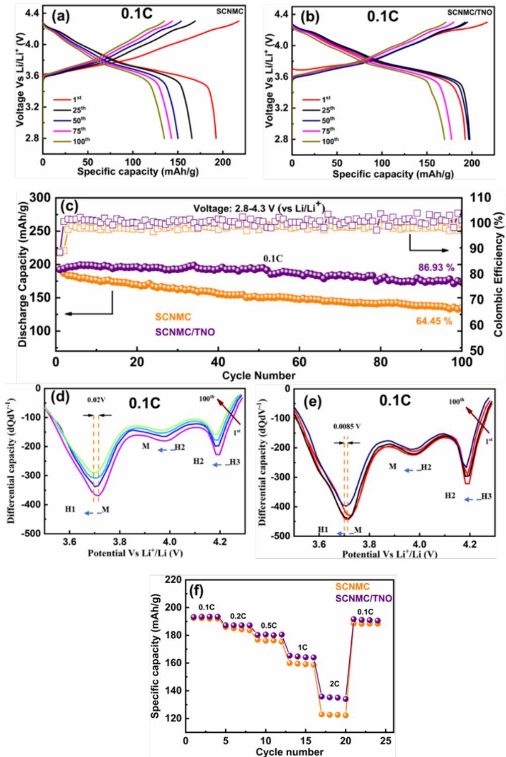
Figure S10. Li/NMC charge-discharge profiles with 1M LiPF<sub>6</sub> in EC: EMC (3:7, v:v) from 2.8 - 4.3 V at 0.1 C for (a) SCNMC, (b) SCNMC/TNO, c) corresponding discharge capacity vs coulombic efficiency plots; dQ/dV curves derived from the 1<sup>st</sup> to 100<sup>th</sup> cycle curve at 0.1 C for (d) SCNMC and (e) SCNMC/TNO, respectively, (f) rate capability.
