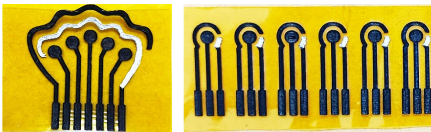
Fig. S9. Digital images of nanoPd@LIG in multi-working electrode and three-electrode systems.
