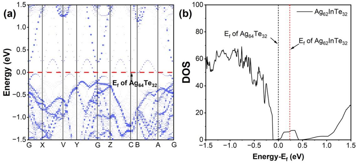
Fig. S5 (a) The band structure of  $\text{Ag}_{62}\text{InTe}_{32}$ . (b) The total DOS for  $\text{Ag}_{62}\text{InTe}_{32}$ . The black and red lines represent the  $E_f$  positions of  $\text{Ag}_{64}\text{Te}_{32}$  and  $\text{Ag}_{62}\text{InTe}_{32}$ , respectively.
