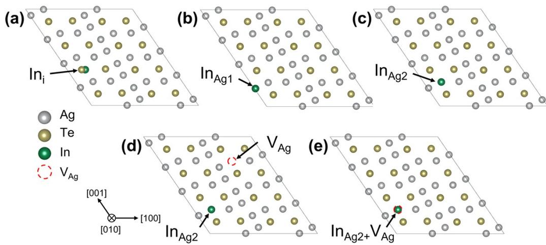
Fig. S4 The structural drawings for different defects.
