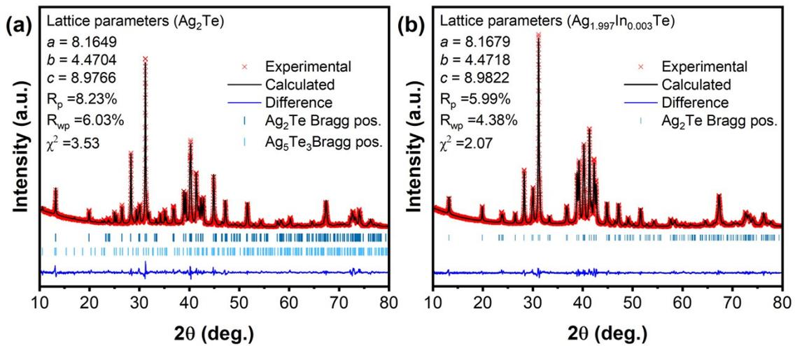
Fig. S2 Rietveld refinement profiles for (a) undoped  $\text{Ag}_2\text{Te}$  and (b)  $\text{Ag}_{1.997}\text{In}_{0.003}\text{Te}$
