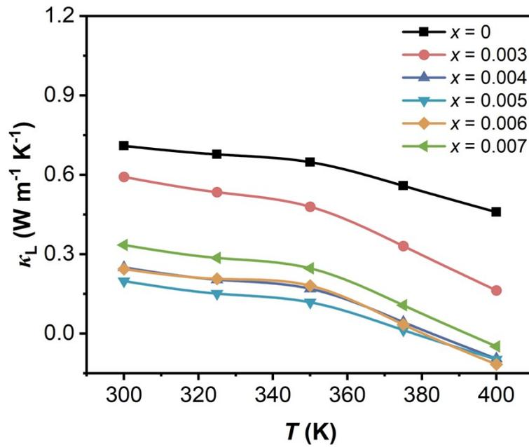
Fig. S6 Temperature dependence of lattice thermal conductivity for  $\text{Ag}_{2-x}\text{In}_x\text{Te}$  ( $x = 0-0.007$ ) samples.
