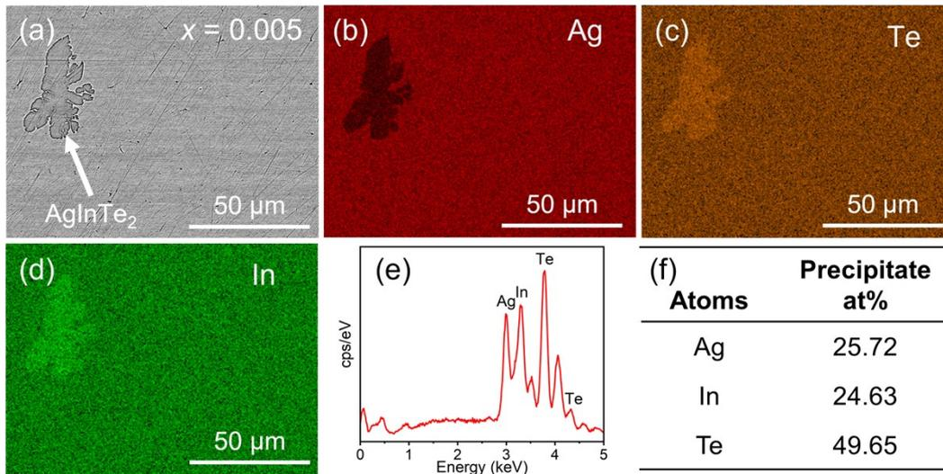
Fig. S1 Backscattering-electron (BSE) image of  $\text{Ag}_{1.995}\text{In}_{0.005}\text{Te}$  sample and (b)-(d) corresponding elemental mappings of Ag, Te and In, respectively. (e) EDS point analysis spectra and (f) EDS point analysis of Te-rich precipitates.
