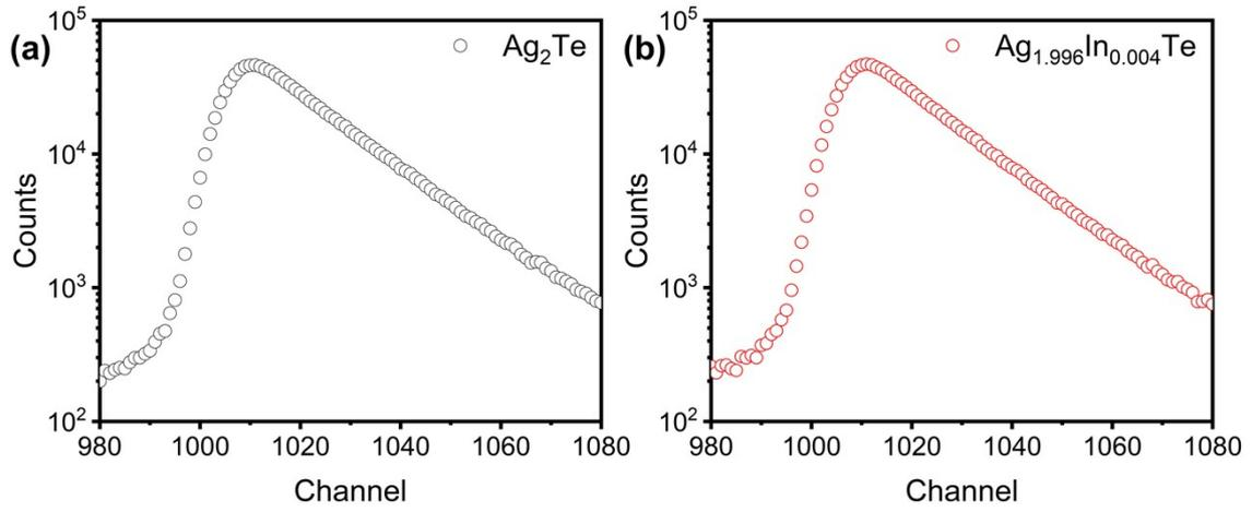
Fig. S3 Positron annihilation lifetime (PAL) spectra of (a) undoped  $\text{Ag}_2\text{Te}$  and (b)  $\text{Ag}_{1.996}\text{In}_{0.004}\text{Te}$ . (20 ps per channel)
